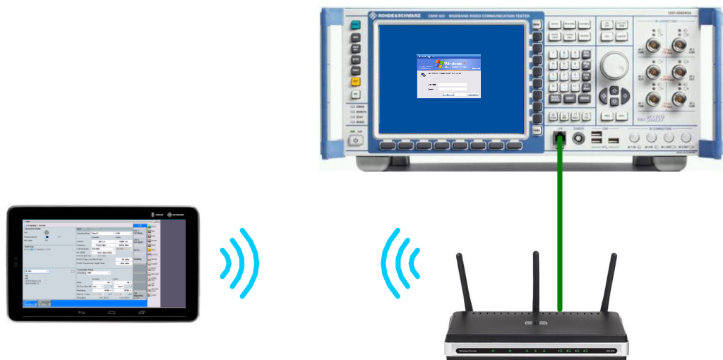
Fig. 1: T&M instrument connected with tablet via WLAN router
