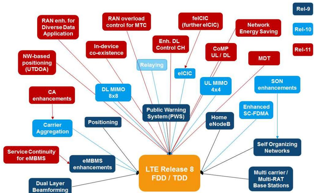
Fig. 1-1: 3GPP Release 8 to 11 technology component dependencies
