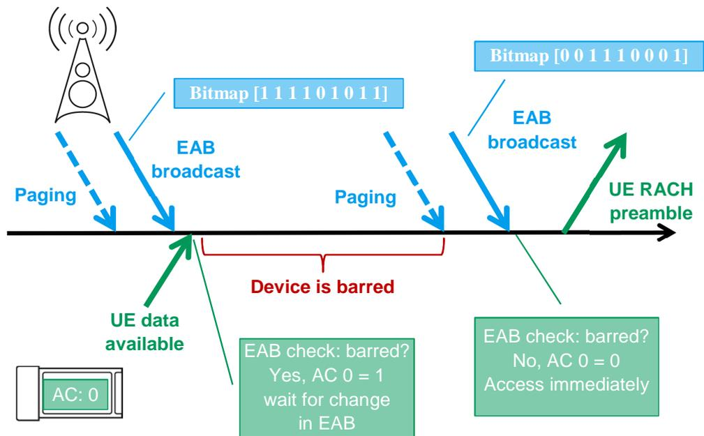
Fig. 2-21: EAB principle
