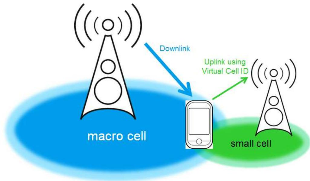
Fig. 2-11: Virtual Cell ID for Uplink CoMP
