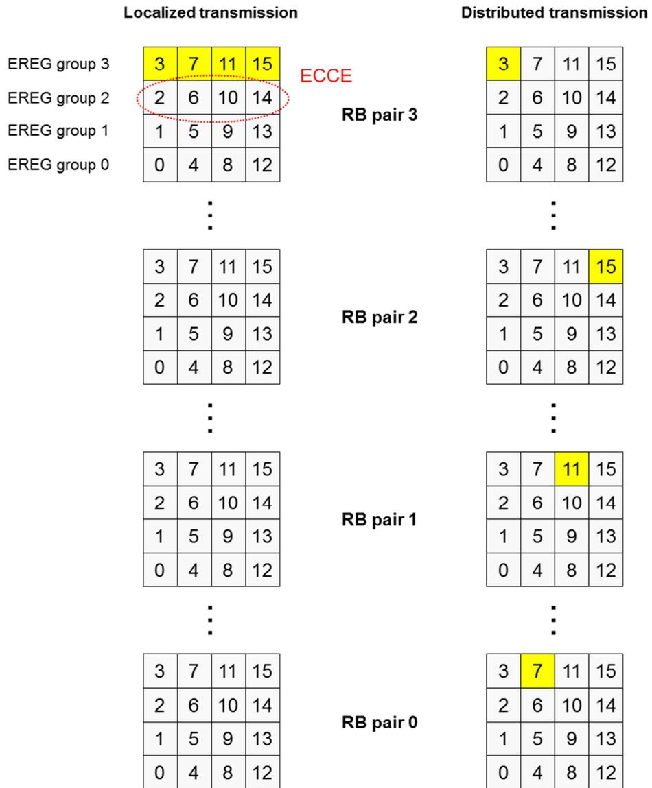
Fig. 2-15: E-PDCCH – Localized versus Distributed Transmission
