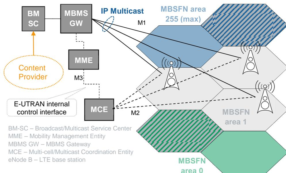
Fig. 2-17: MBMS architecture and interfaces
