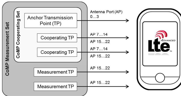
Fig. 2-6: Downlink CoMP Cooperating and Measurement set for cells using the same cell identity.
