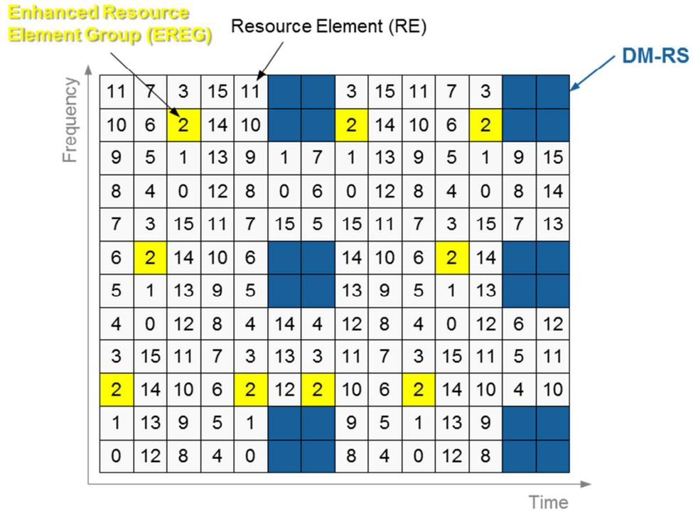
Fig. 2-13: Enhanced Resource Element Group (EREG) for E-PDCCH
