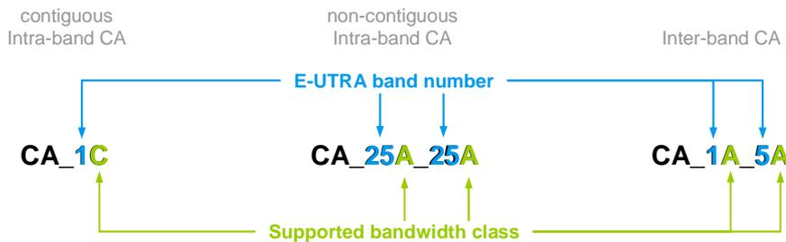
Fig. 2-3: Notation of carrier aggregation support (type, frequency band, and bandwidth)
