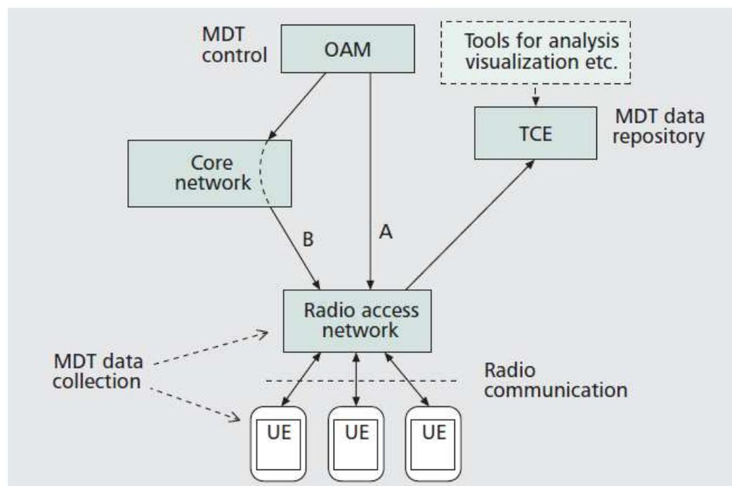
Fig. 2-22: Measurement control of MDT by the OAM. Path A denotes the management-based MDT, path B the signaling-based MDT (source [16]).
