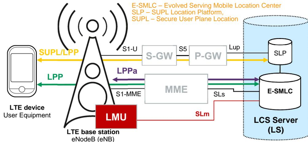
Fig. 2-16: E-UTRA supported positioning network architecture
