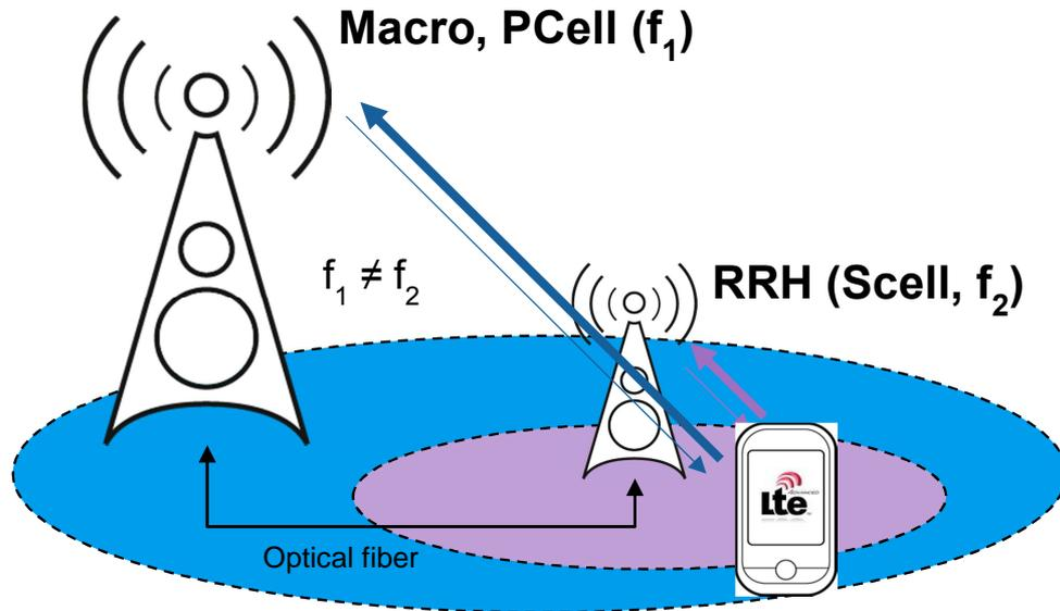
Fig. 2-1: CoMP scenario 3 requires different timing advance if multiple carriers are used in UL
