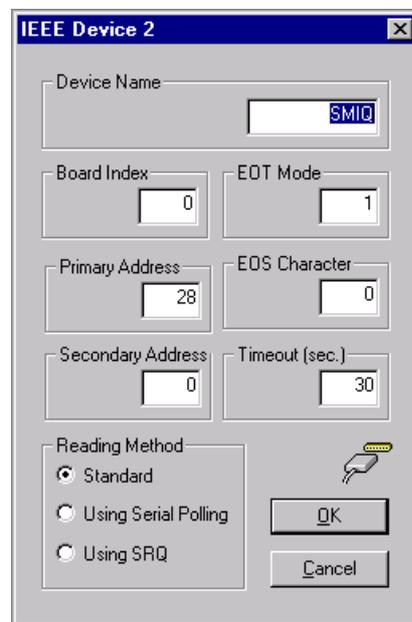
Fig. 13: Winbatch window for remote-control parameters
