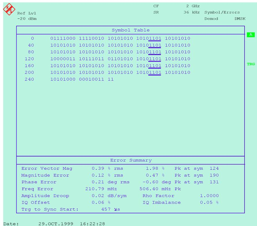
Fig. 4: Phase / frequency error for NBU
