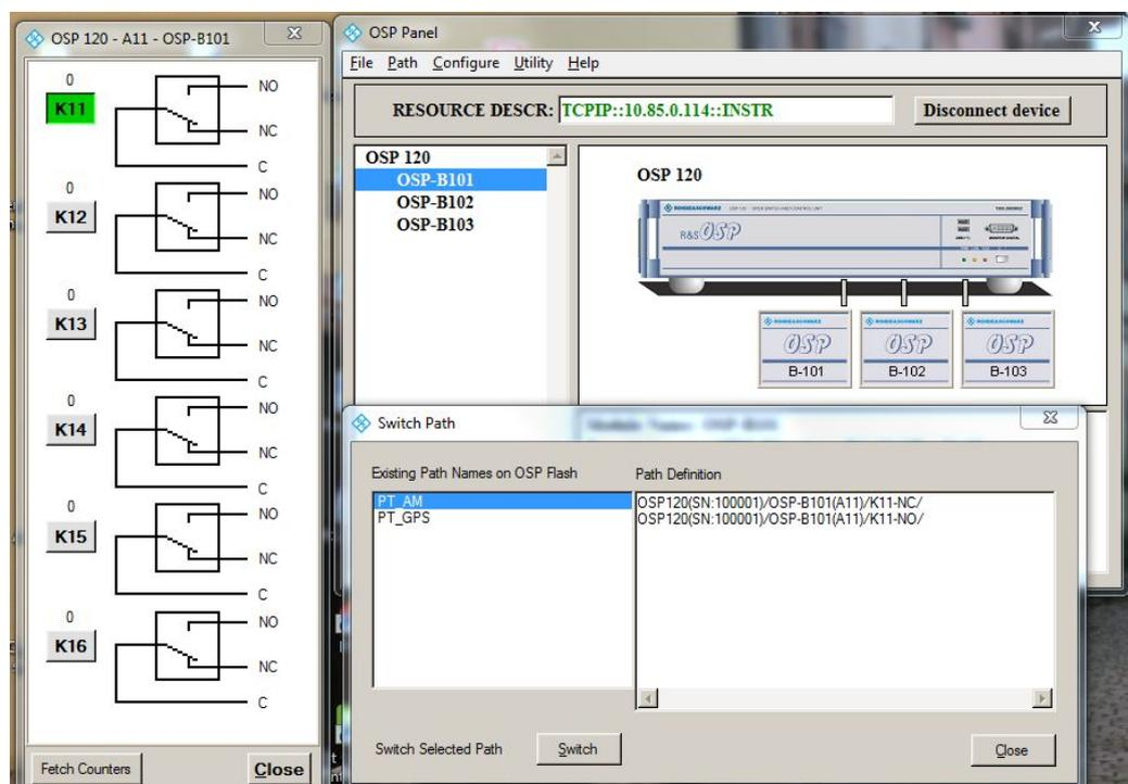
Figure 5-4: Path definition for AM using OSP panel software
