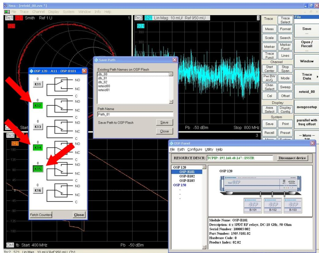
Figure 2-3: Green check marks have to be set to include the relays into the path definition (red arrows)
