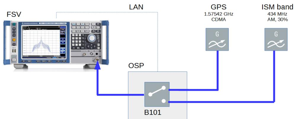
*Figure 5-3: Reference example using FSV along with two generators*
