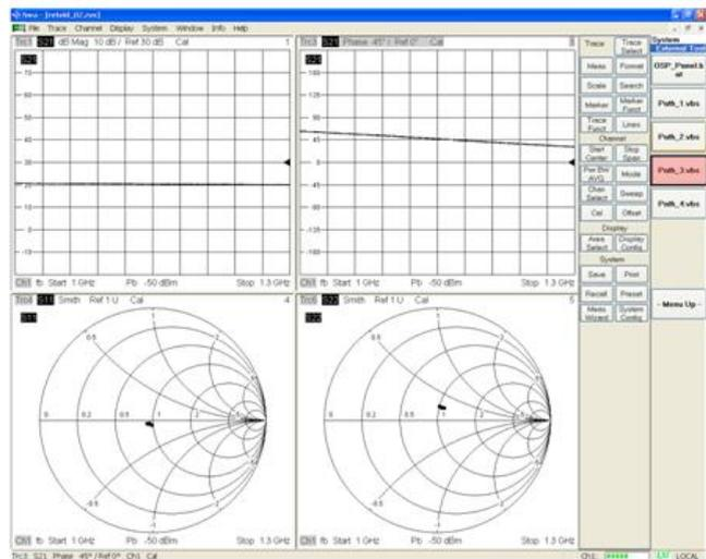
Figure 4-5: Results are immediately displayed when pressing the red marked softkeys at the right of the VNA
