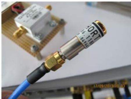
Calibration standards have to be mounted at the ends of both cables in order to perform calibration including all paths up to the DUT.
