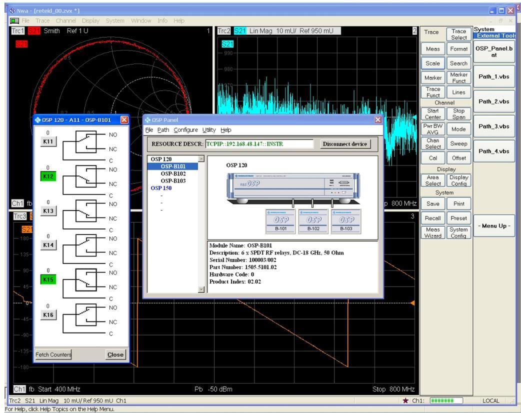
Figure 1-1: OSP Panel Software being installed on a VNA to control external switch matrices
