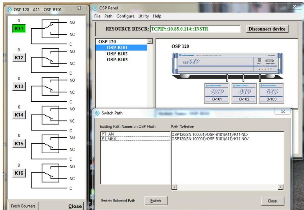
Figure 5-5: Path definition for GPS using OSP panel software
