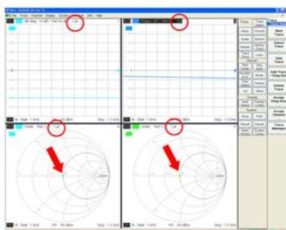
After calibration the CAL id is set (red circles) and the S11 and S22 results are close to the center of the Smith Chart (red arrows), according to the very good 50 Ohms impedance of the DUTs input and output.
