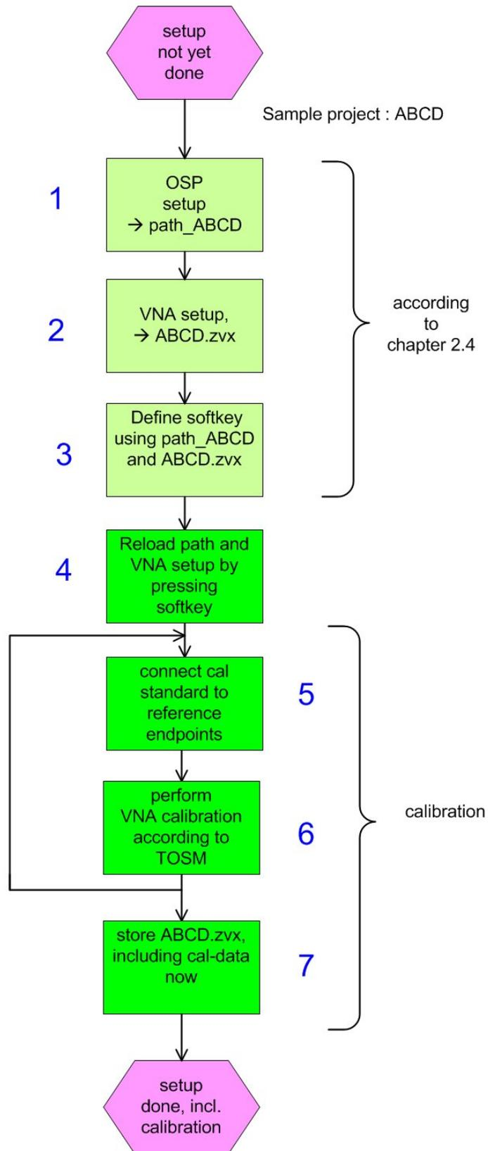
Figure 3-2: Calibration workflow to extend ABCD.zvx by calibration data
