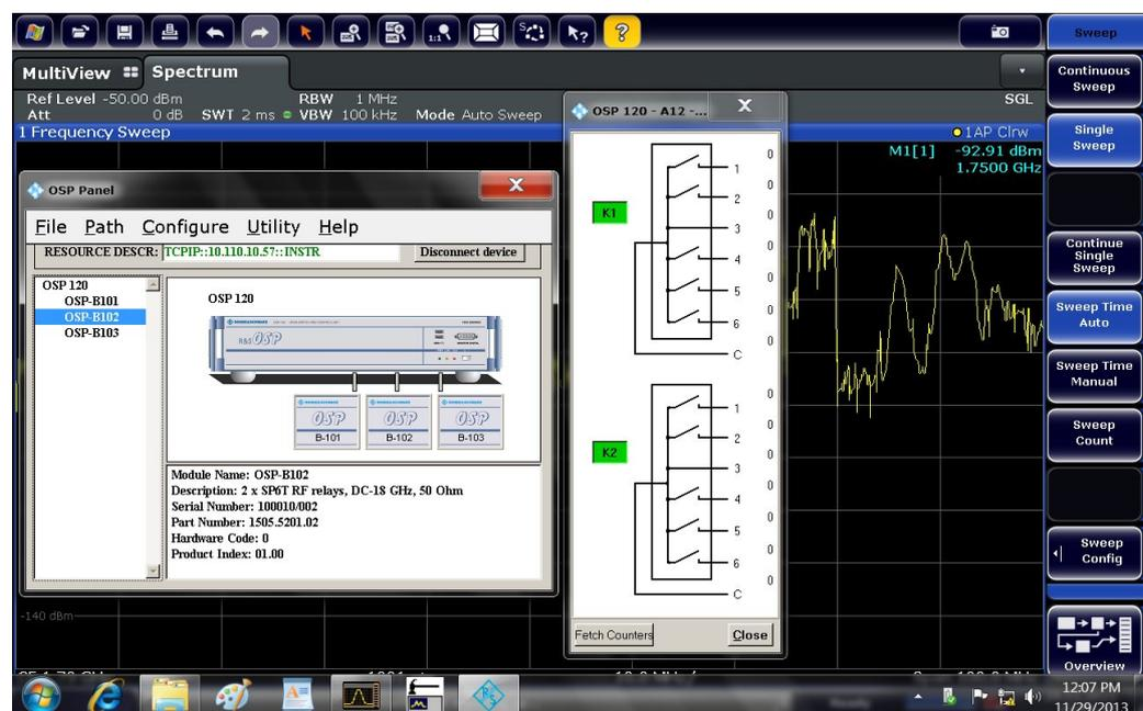
Figure 5-2: Direct remote control of the switch matrix OSP via spectrum analyzer FSW and an external LAN Router
