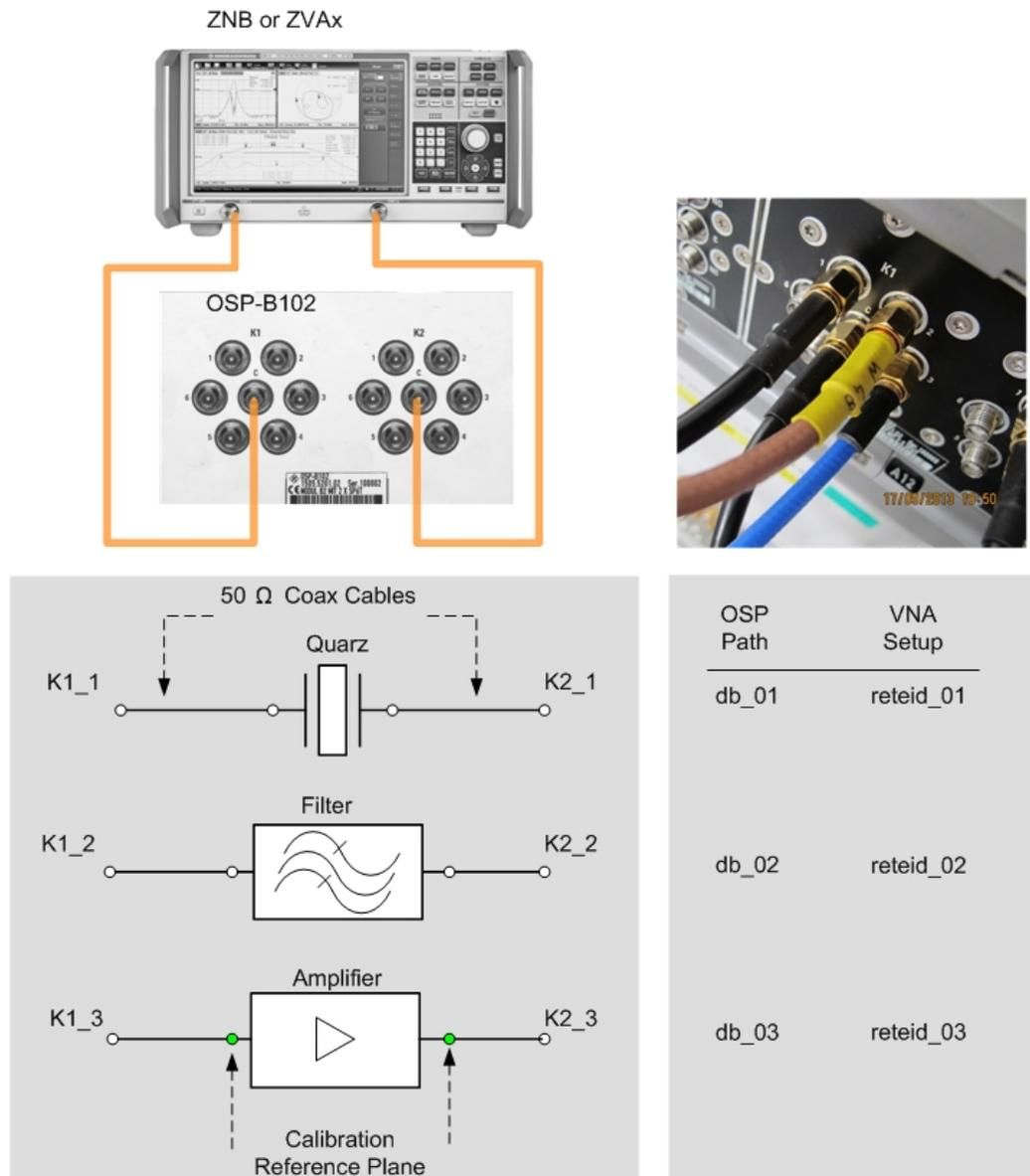
Figure 4-1: The figure shows the block diagram, upper left, connections to the OSP K1-Port, photo in the upper right, DUTs and connections, lower left and the OSP PATH names along with the appropriate VNA setup according to each DUT, table in the lower right.
