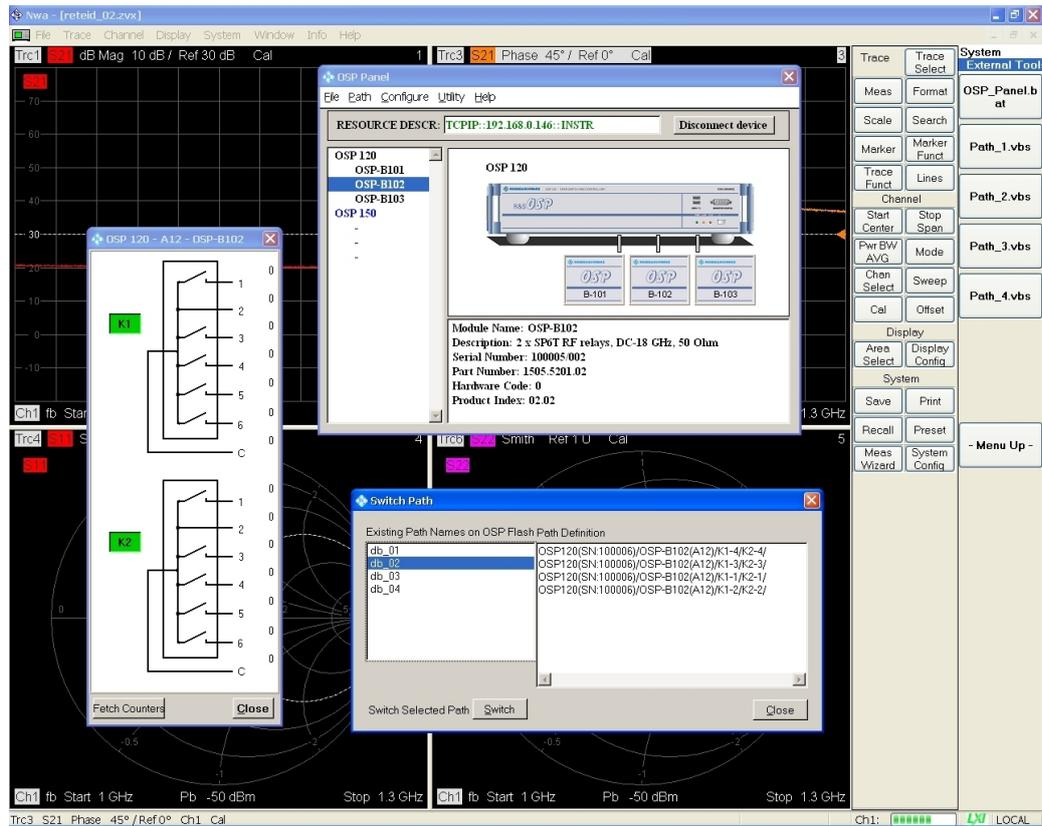
**Figure 4-2:** Shows the definition of the path for the band filter test using the OSP Panel Software installed on the VNA. The settings of OSPs K1 and K2 are finally stored in the OSP path named "db\_02"
