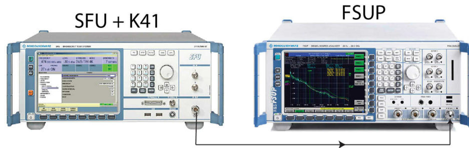
Figure 3-7: Measurement setup to verify custom phase noise profile using an FSUP
