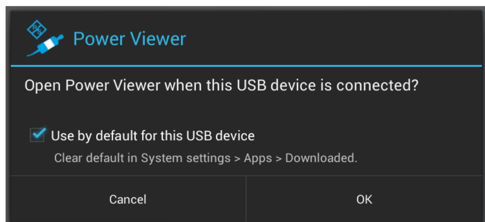
Fig. 2-2: R&S®Power Viewer Mobile detects the R&S®NRP USB sensor automatically
