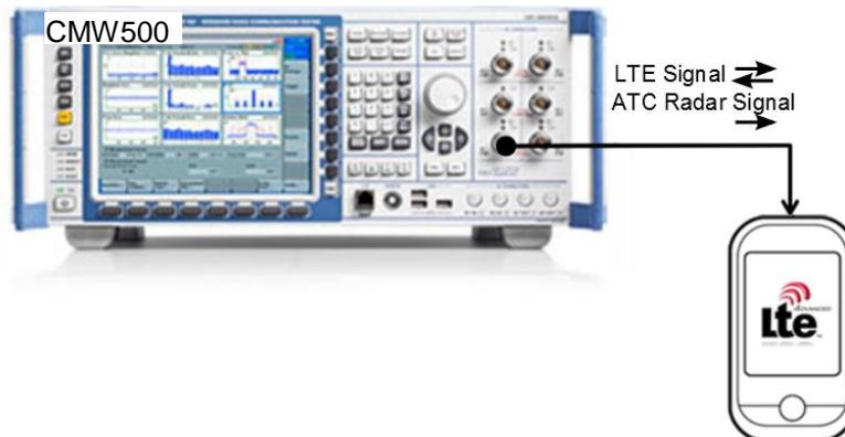
Figure 4-4: CMW500 with advanced RF frontend and DUT
