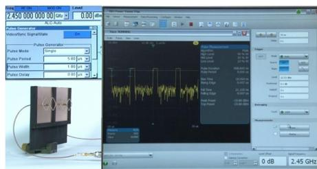
By means of this configuration it is shown how to transmit and to receive pulsed radar signals over the air. The pulse evaluation capabilities of the R&S® NRP-Z81 peak power probe are demonstrated, for instance how to reduce noise effects by averaging. The pulse shapes are varied at the signal generator and can be observed at the PC which is evaluating signals coming from the peak power probe via USB.
