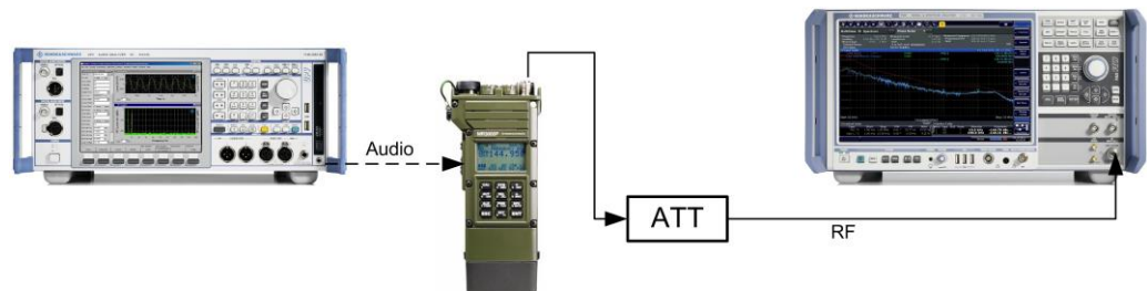
Fig. 14: Basic setup for the transmitter test. The analyzer measures the TX signal from a radio via an attenuator. The input signal can be an audio signal from the UPV audio generator, for example.
