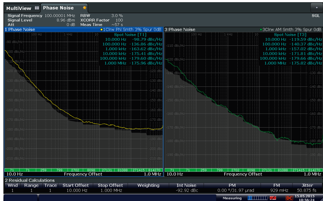
Fig. 28: Phase noise measurement using the FSWP.
