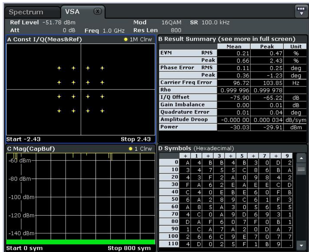
Fig. 18: Example for the analysis of a 16QAM signal using the K70. The figure shows the constellation diagram, an overview of the most significant results and the symbol (bit) stream.
