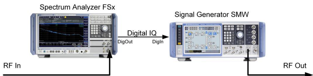
Fig. 48: RF fading using a spectrum analyzer and a signal generator. The I/Q data sampled by the FSx is transmitted to the SMW via a digital interface, faded and then upconverted to the original frequency.
