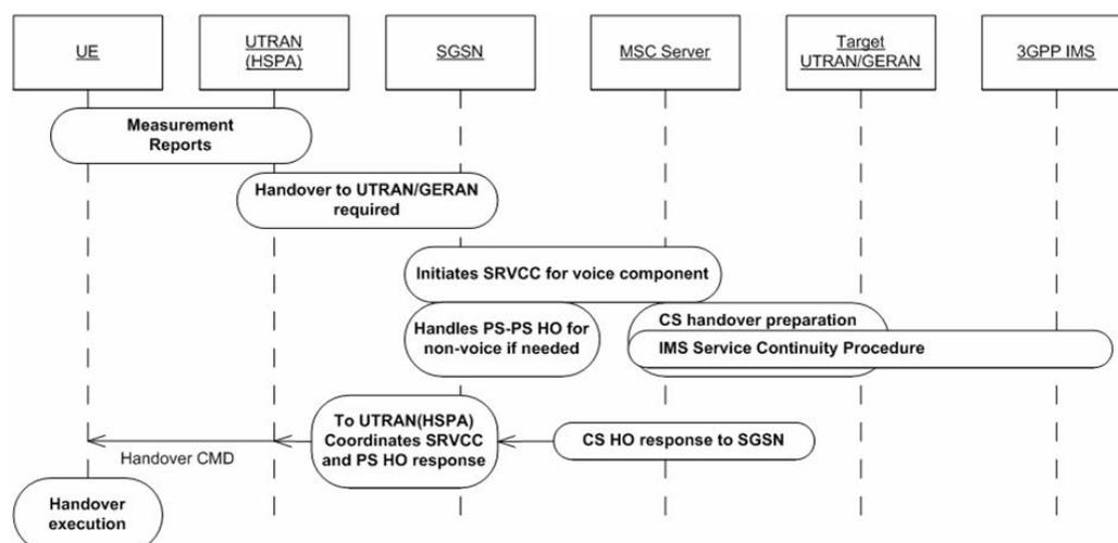
Figure 47: Overall high level concepts for SRVCC from UTRAN (HSPA) to UTRAN/GERAN
