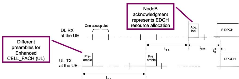
Figure 40: UL/DL timing relation for Enhanced Uplink in CELL\_FACH as seen at the UE [3]
