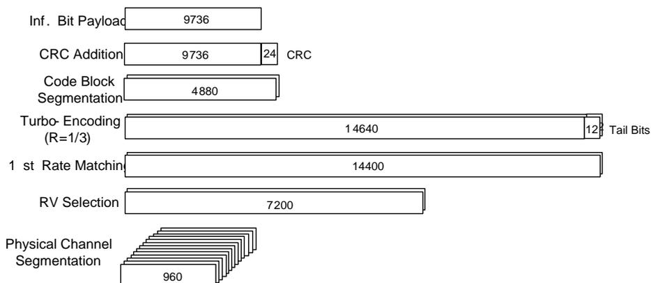
**Figure 5: Coding rate for Fixed Reference Channel H-Set 9 Secondary Transport Block**
