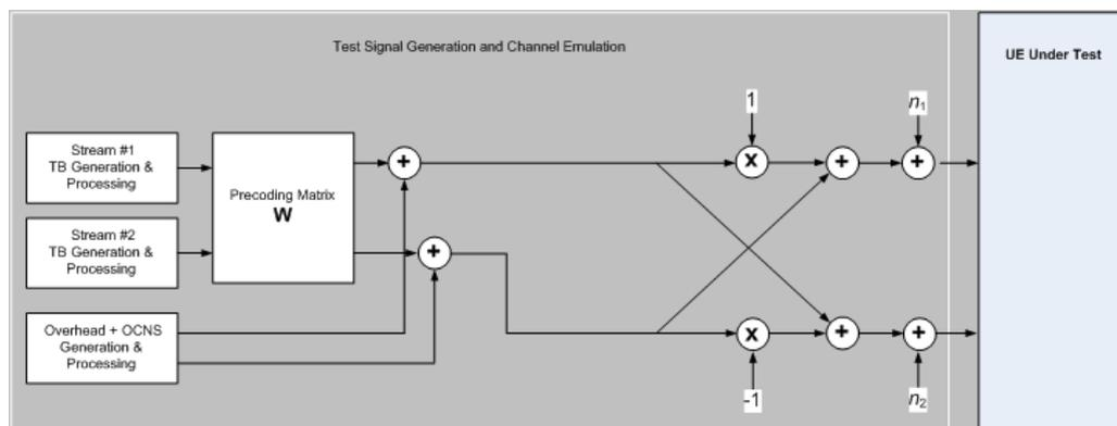
Figure 8: Test setup under MIMO Dual Stream Static Orthogonal Conditions
