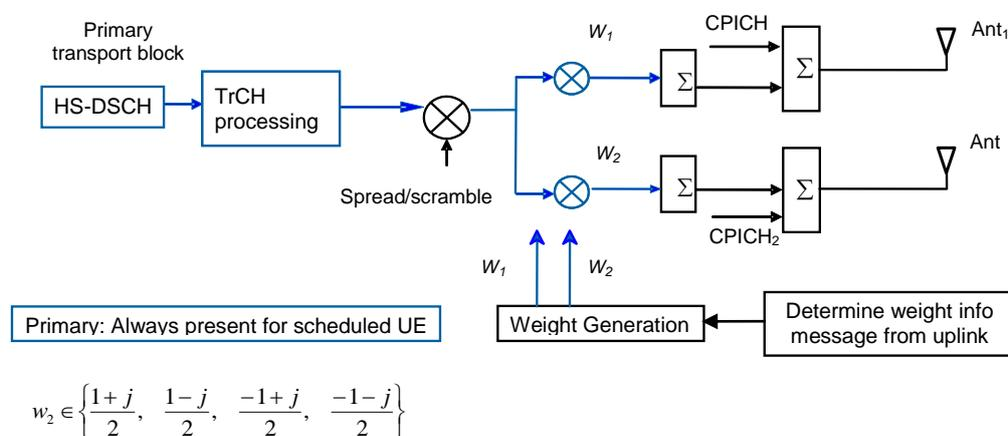
**Figure 56: Generic downlink transmitter structure to support MIMO operation for HS-PDSCH transmission when single-stream restriction is configured**
