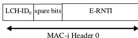
Figure 44: MAC-i header part for E-RNTI transmission
