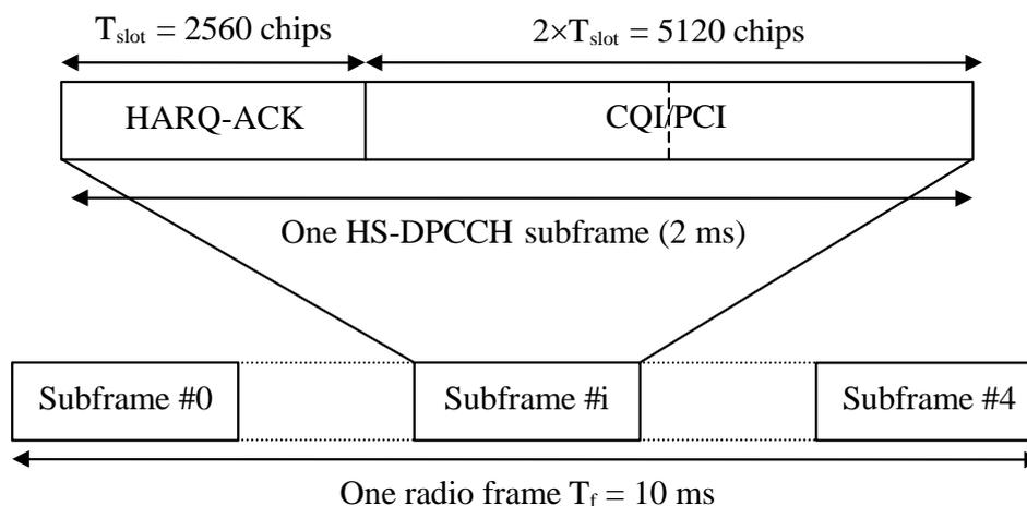
Figure 58: Frame structure for uplink HS-DPCCH
