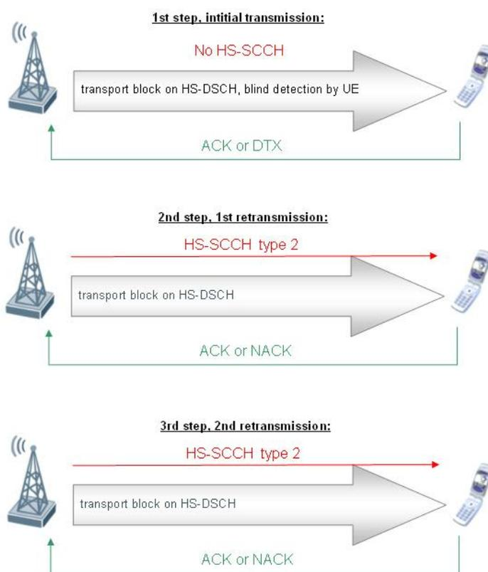
Figure 13: HS-SCCH less operation
