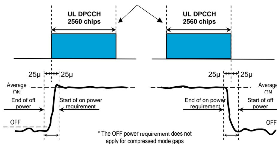
Figure 16: Transmit ON/OFF template for discontinuous uplink DPCCH transmission
