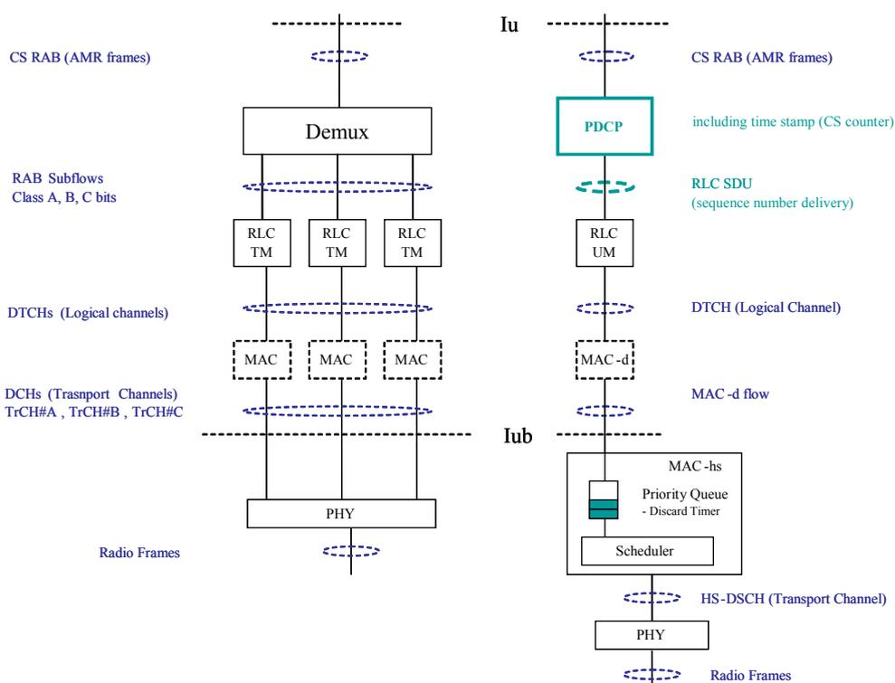
**Figure 28: Downlink U-plane multiplexing: Legacy vs. CS over HSPA scheme**
