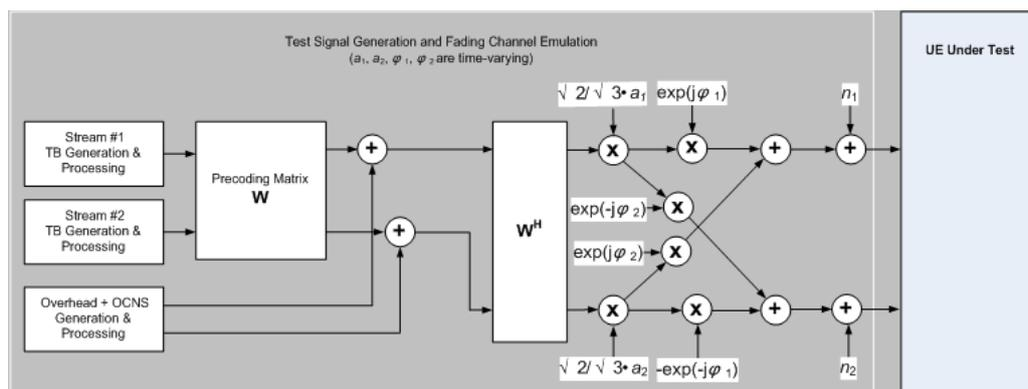
Figure 7: Test setup under MIMO Dual Stream Fading Conditions
