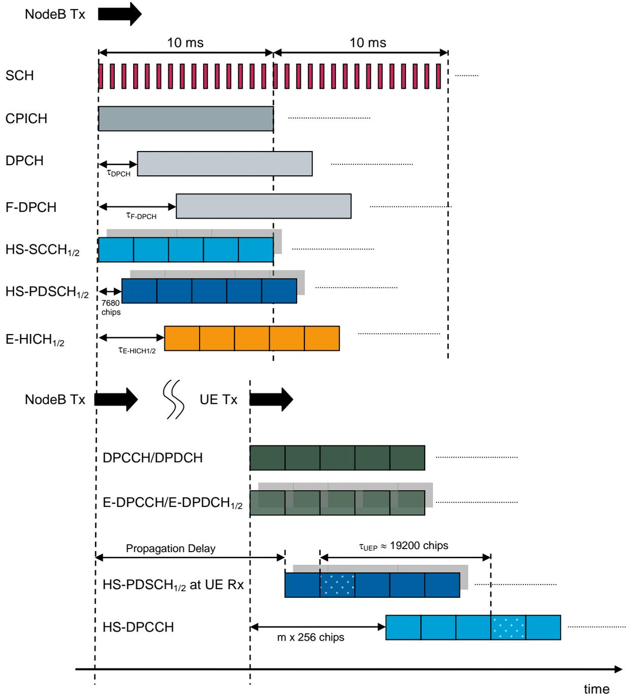
Figure 50: Timing relation of between physical channels in dual cell HSUPA operation
