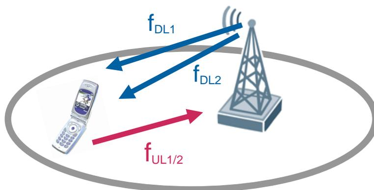
**Figure 31: Dual Cell HSDPA operation**
