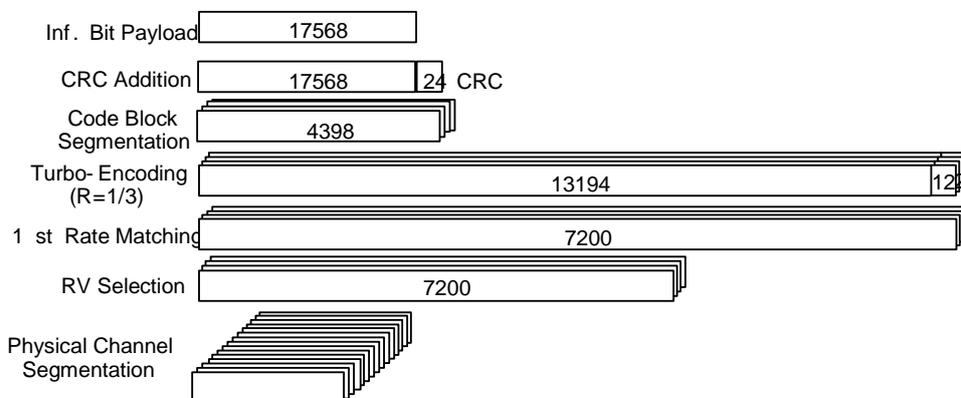
**Figure 4: Coding rate for Fixed Reference Channel H-Set 9 Primary Transport Block**
