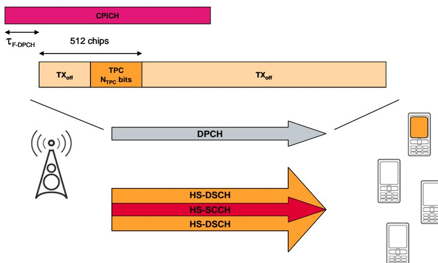
**Figure 17: Rel6 Frame structure for F-DPCH**
