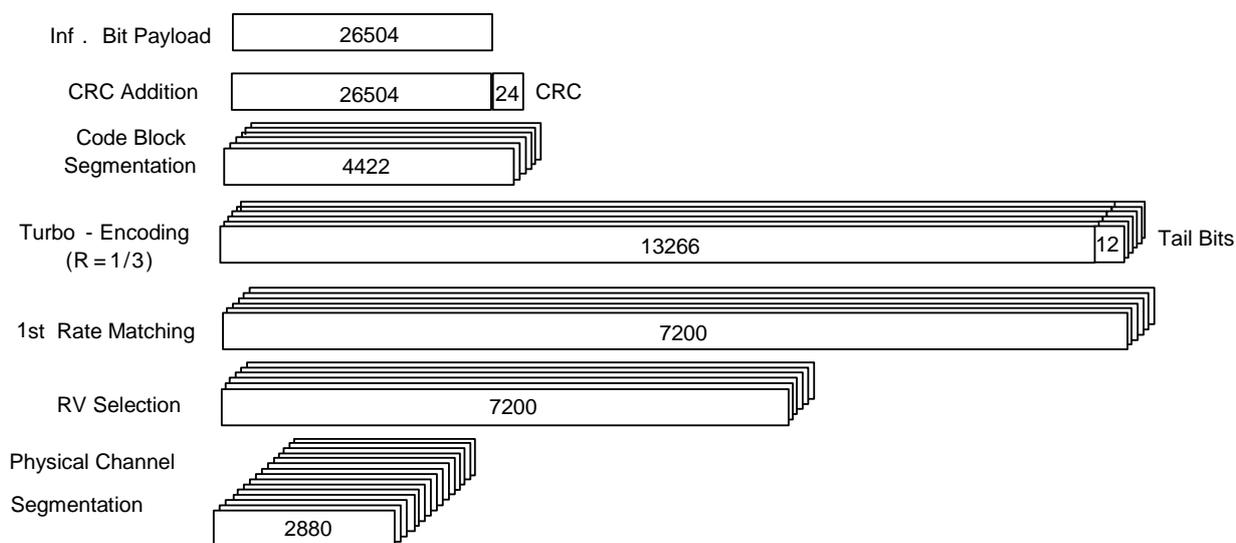
Figure 26: Coding rate for Fixed Reference Channel H-Set 11 Primary Transport Block
