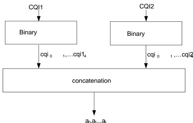
**Figure 32: Concatenated CQI values for dual cell HSDPA**
