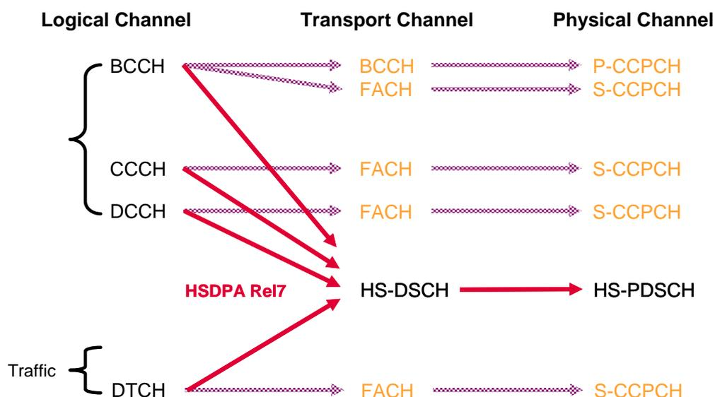
**Figure 23: Mapping of logical channels on transport and physical channels in CELL\_FACH state**
