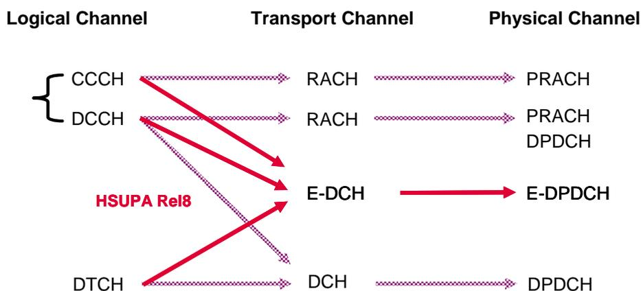
**Figure 39: Mapping of logical channels on transport and physical channels for enhanced uplink in CELL\_FACH state**
