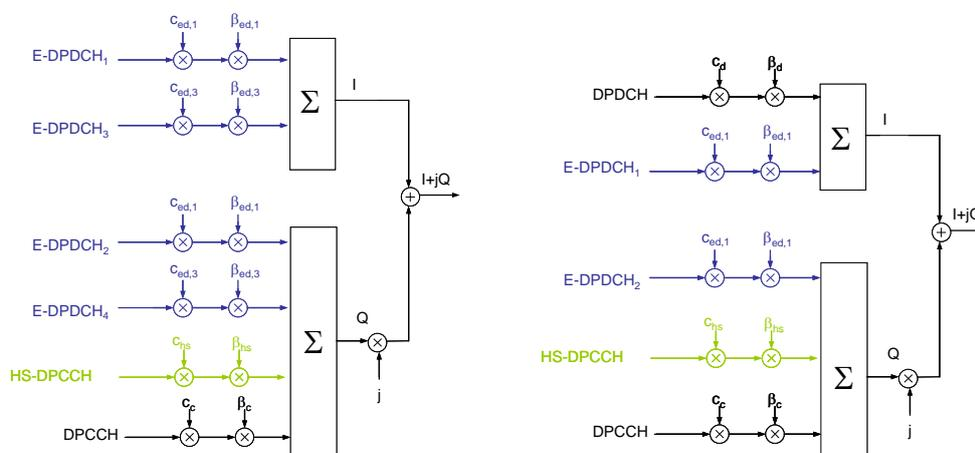
**Figure 33: Physical Channel mapping in case of four EDPDCH codes and two EDPDCH codes**
