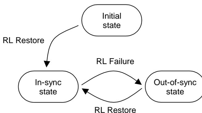
Figure 41: Node B radio link set states and transitions [2]
