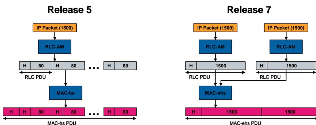
Figure 21: Flexible RLC PDU size operation
