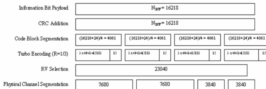
**Figure 11: Fixed Reference Channel (FRC8) – 16QAM parameters**
