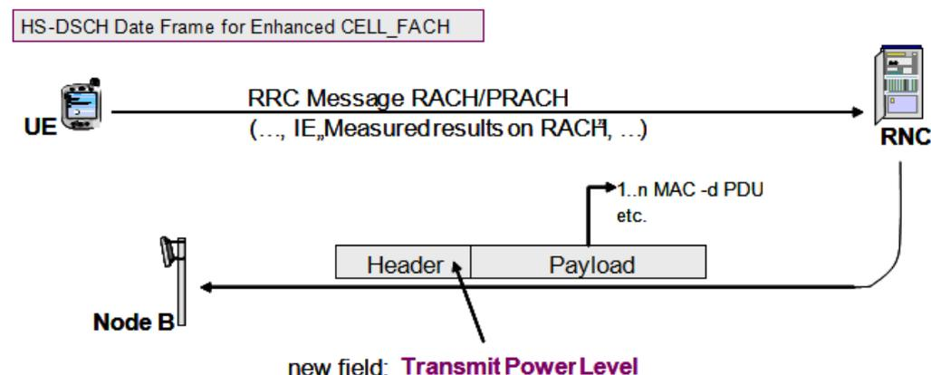
Figure 25: Measurement reporting procedure in Enhanced CELL\_FACH
