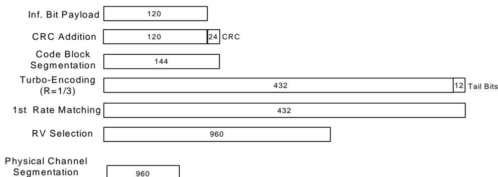
**Figure 34: Coding rate for fixed reference channel H-Set 12 (QPSK)**
