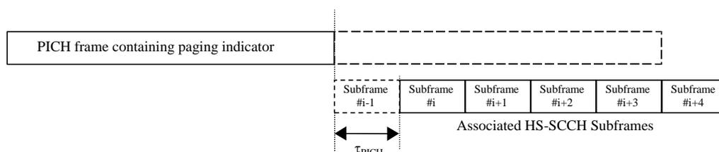
**Figure 24: Timing relation between PICH frame and associated HS-SCCH subframes**
