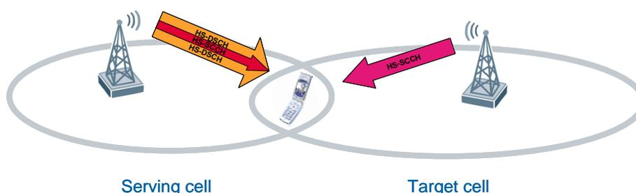
Figure 48: Enhanced serving HS-DSCH cell change procedure
