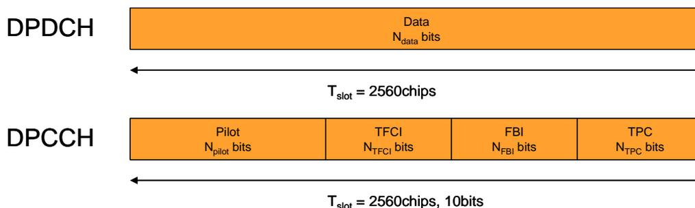
Figure 15: Uplink DPDCH/DPCCH slot format (one slot shown)
