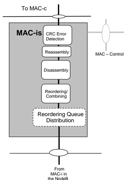
**Figure 45: UTRAN side MAC architecture / MAC-is details (for CCCH transmission)**
