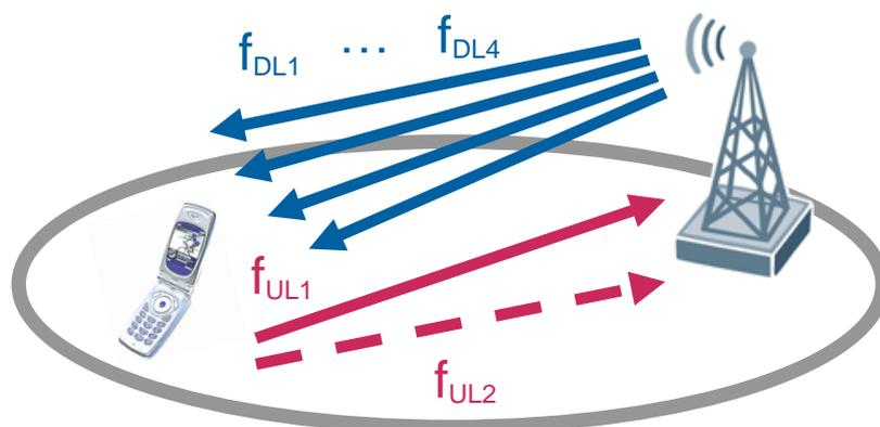
**Figure 57: Principle of four carrier HSDPA operation**
