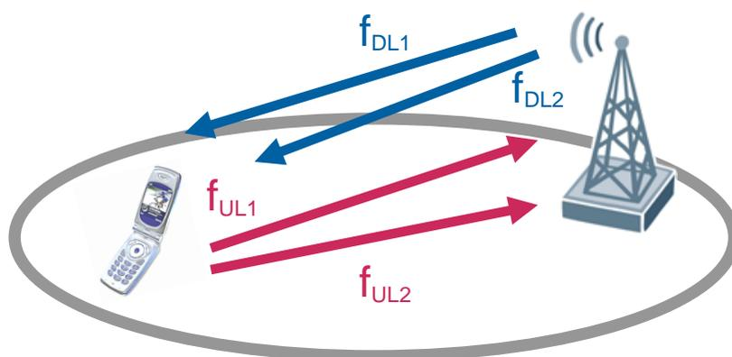
*Figure 49: Dual Cell HSUPA operation (including Dual Cell HSDPA)*
