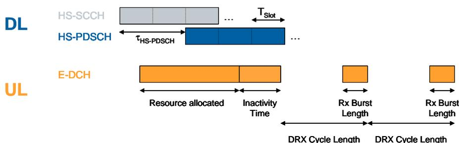
Figure 46: HS-DSCH DRX operation in CELL\_FACH state
