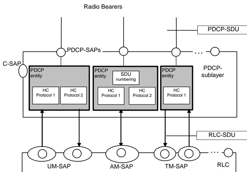
**Figure 29: PDCP structure**
