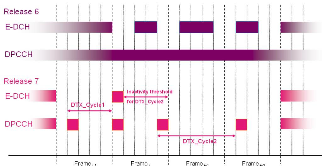
Figure 12: Uplink DTX example, 2 ms TTI (pre-/postambles not shown), [2]
