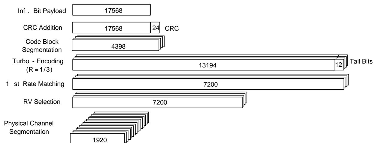
Figure 27: Coding rate for Fixed Reference Channel H-Set 11 Secondary Transport Block
