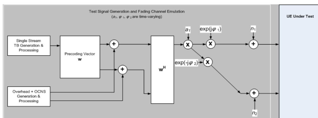
**Figure 6: Test setup under MIMO Single Stream Fading Conditions**
