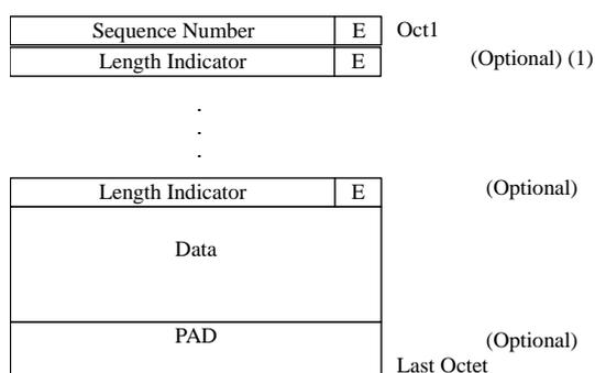
**Figure 30: Unacknowledged Mode Data (UMD) PDU**
