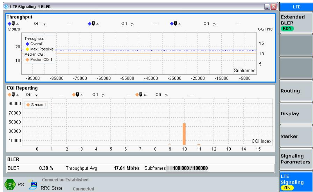
Fig. 3-22: LTE RX measurement for Tx diversity (MISO).
