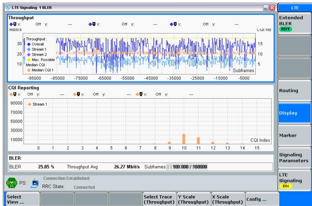
Fig. 3-28: LTE RX measurement for 2x2 MIMO. The measurements are adapted automatically for both streams individually as well as in the form of an overall assessment.
