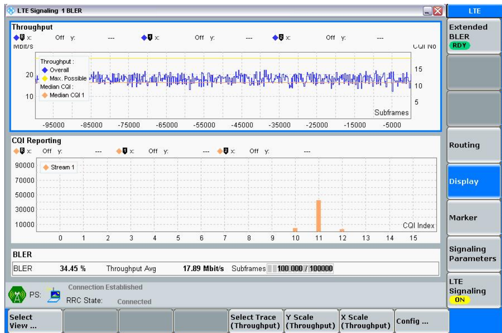
Fig. 3-18: LTE RX measurement for Rx Diversity (SIMO).
