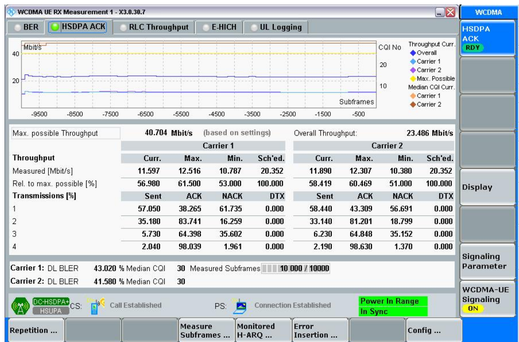
Fig. 4-22: WCDMA RX measurement for DC-HSPA. The measurements are adapted automatically for both streams individually and as an overall assessment.
