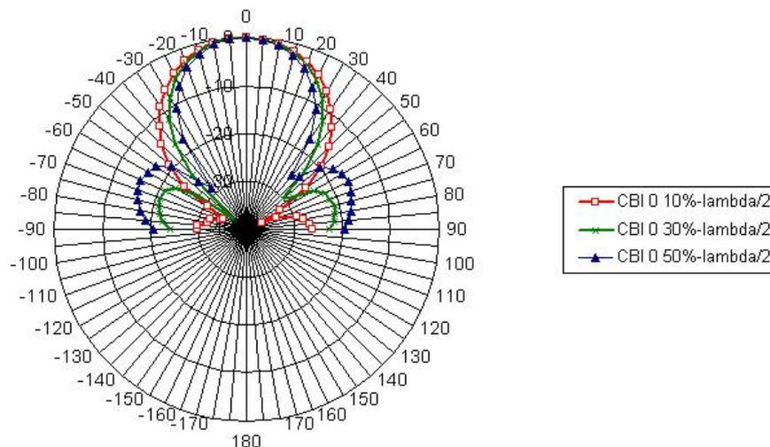
**Figure 4:** The antenna diagram is affected by the distance  $d$  between the antennas. In this example,  $d$  is 10 %, 30 %, and 50 % greater than  $\lambda/2$ . (CBI 0 refers to code book index 0, see chapter 3.2.4)
