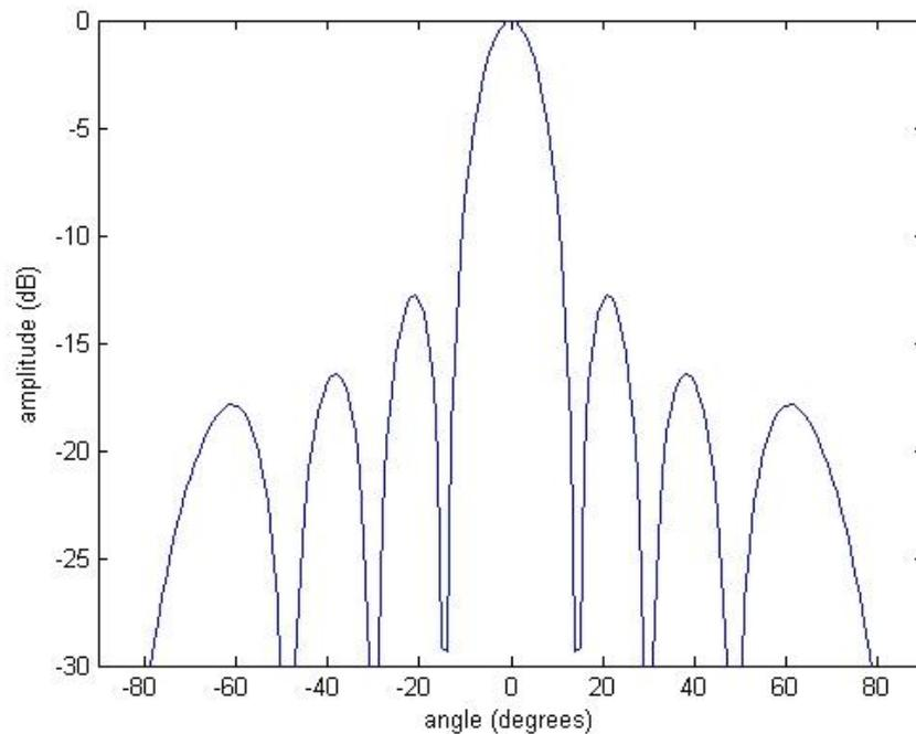
**Figure 3: Beam pattern example of an 8-element ULA**
