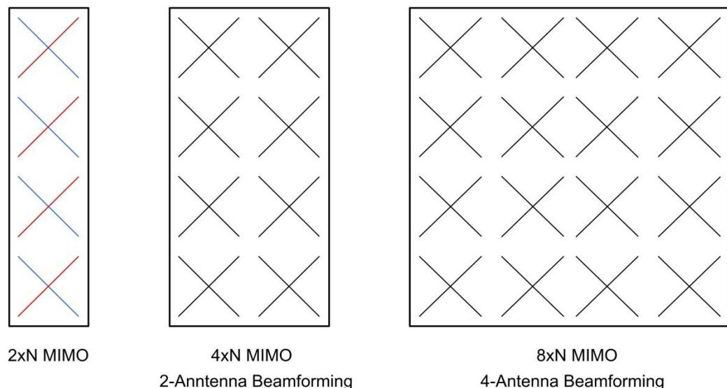
**Figure 5: Various cross-polarized base station antenna arrays for MIMO and beamforming.**
