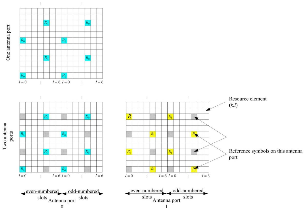
**Figure 6: Distribution of the downlink cell specific reference signals in LTE; see top for one antenna and bottom for two antennas. [1]**
