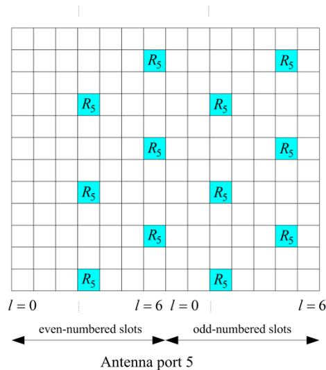
**Figure 7: Distribution of reference signals for transmission mode 7 [1]**
