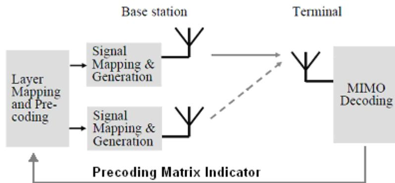
Figure 13: Block diagram for TM 6
