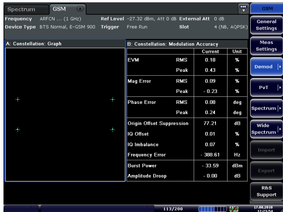
Figure 15: Constellation diagram of a AQPSK signal and measured modulation accuracy values
