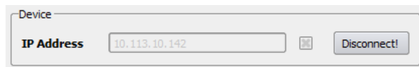
Figure 4: Connection to the instrument established in FSH4Remote, the address is greyed out, Disconnect button appears.
