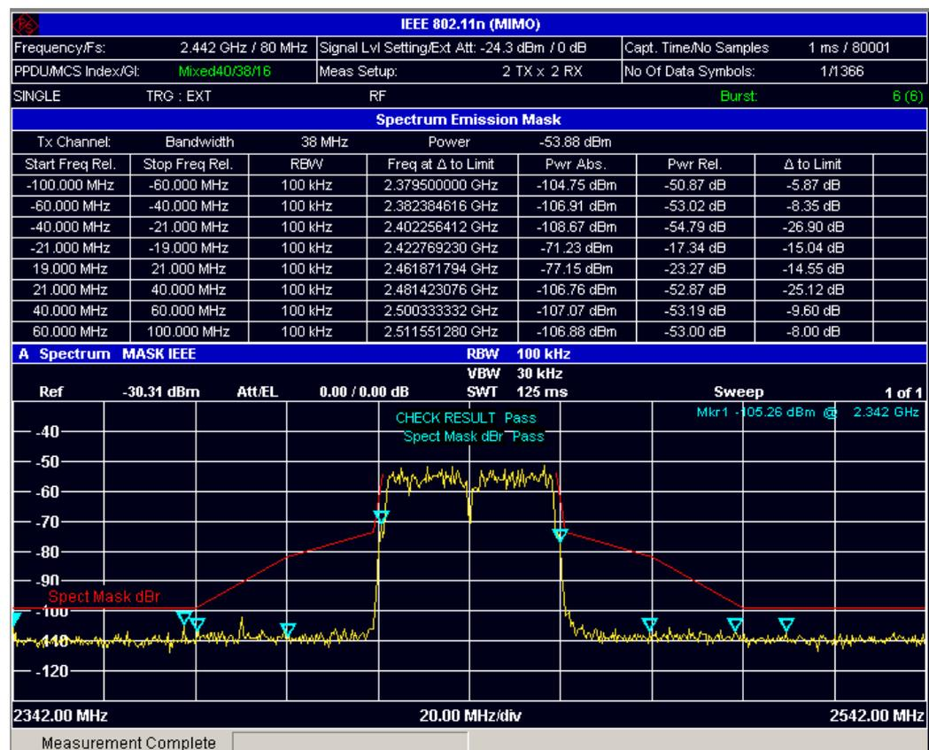
Fig. 57: Spectrum emission mask.
