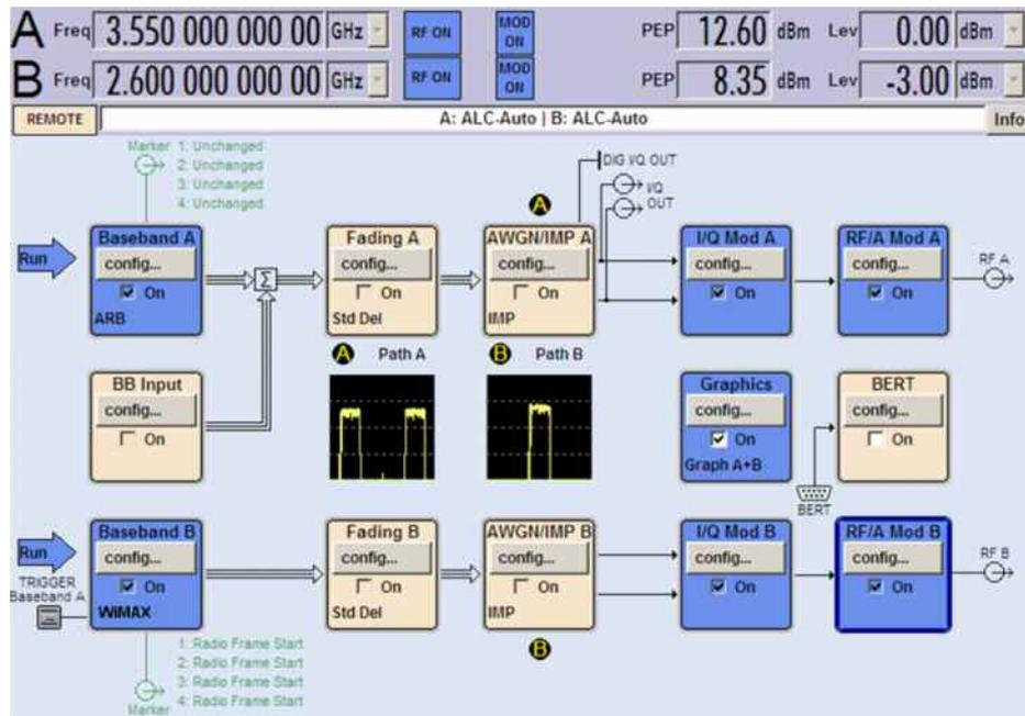
Figure 36: Generating scenario 12 of Table 1 with a 2-path SMU. Path A delivers 2x20 MHz carriers in distributed placement using its multi-carrier ARB function at 3.5 GHz band. Path B delivers a single 20 MHz carrier at 2.6 GHz band. RF A and RF B are externally combined.
