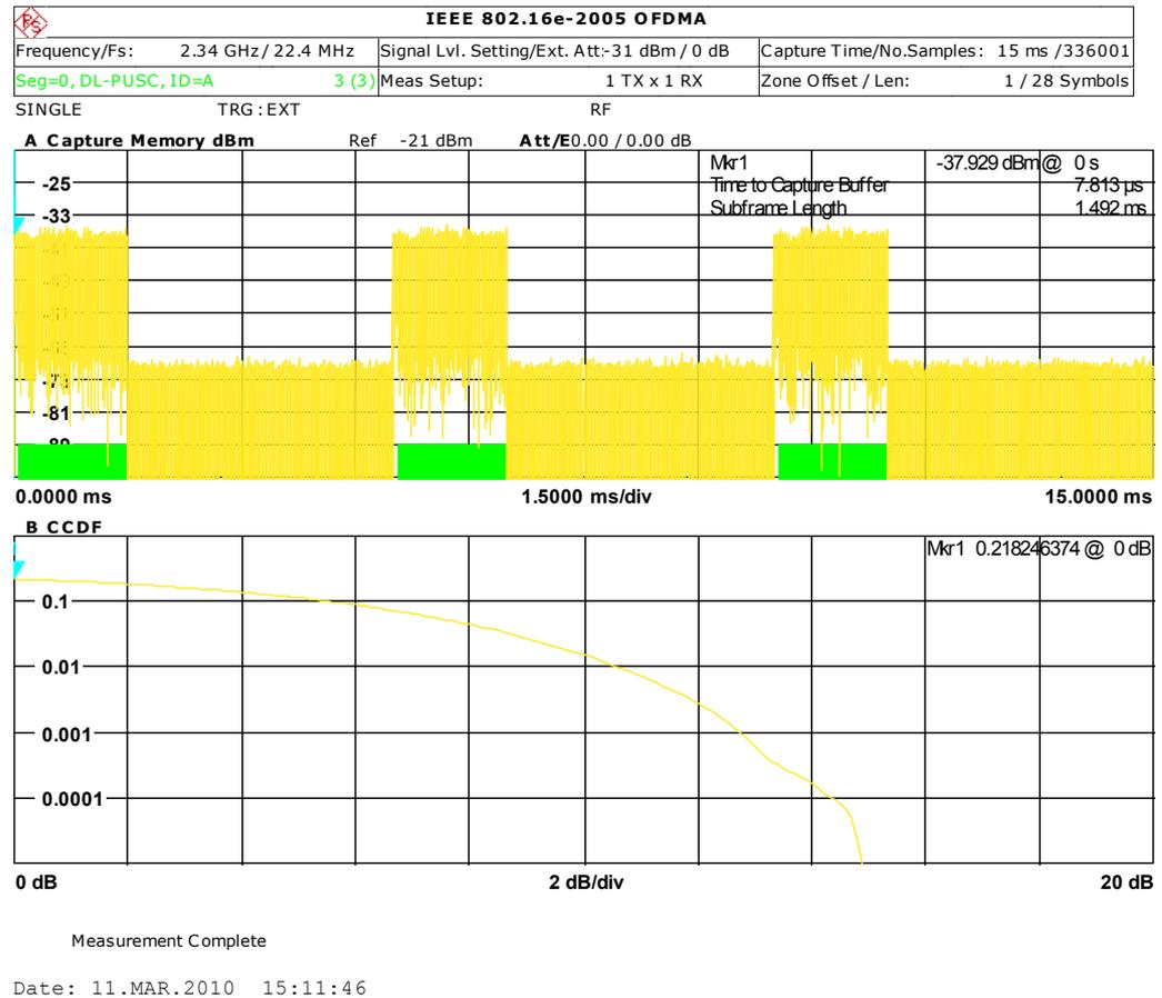
**Figure 43:** In screen A (upper) the capture buffer, in screen B (lower) the CCDF is shown.
