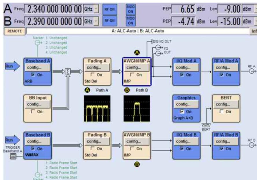
**Figure 32: Configuration of a 2-channel SMU for generating 5 x 20 MHz WIMAX 802.16e carriers in band 40**
