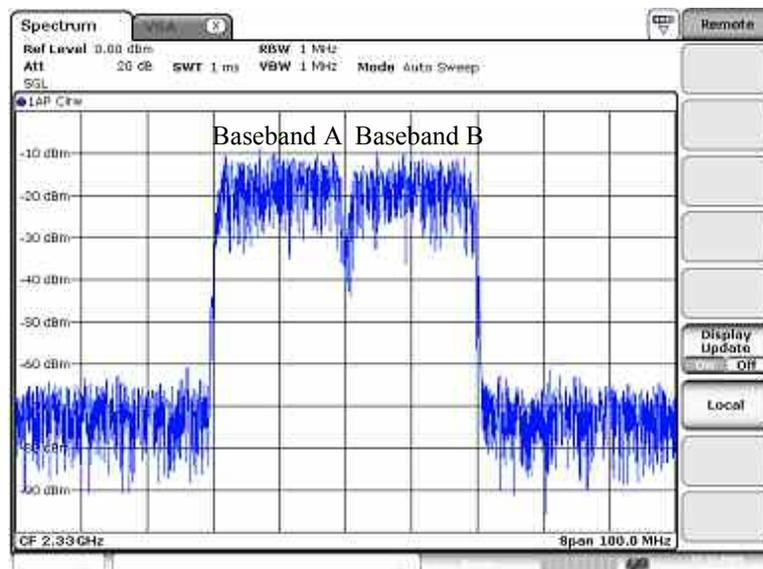
Figure 12: Spectrum of two contiguously placed 20 MHz WIMAX 802.16e Signals generated by an SMU as described above.
