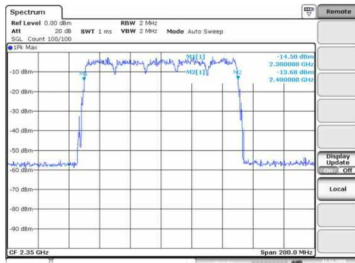
**Figure 34: Output spectrum of contiguous 5x20 MHz carriers**
