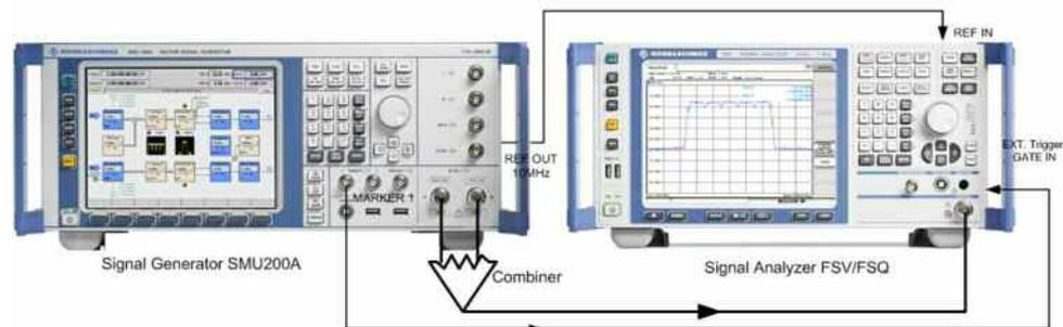
**Figure 31: Test setup with a 2-channel SMU200A (2 baseband modules, 2 RF modules)**
