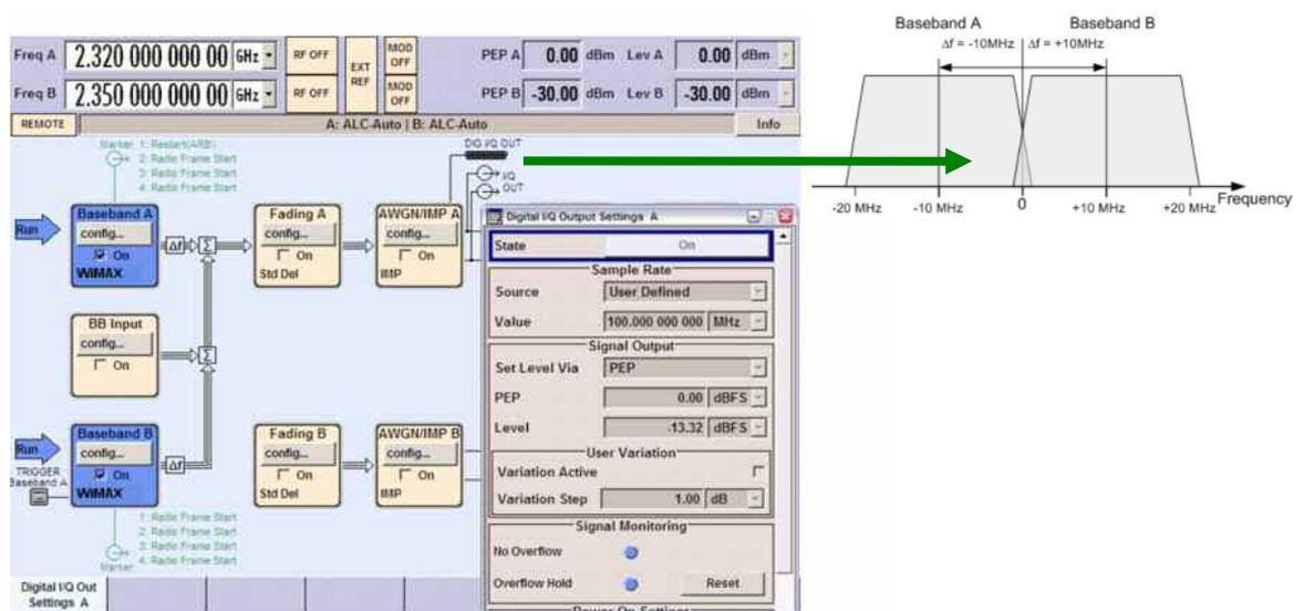
Figure 19: Upper SMU Screen: baseband A&B are combined and output at Digital IQ Out.
