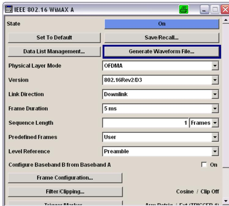
*Figure 25: The currently setup WIMAX 802.16e signal is saved as an arbitrary waveform file via the softkey "Generate Waveform File..."*
