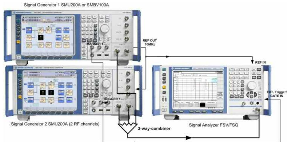
**Figure 38:** Configuration for multi-band deployment scenarios 7 or 10 of Table 1. Three RF channels are combined externally.
