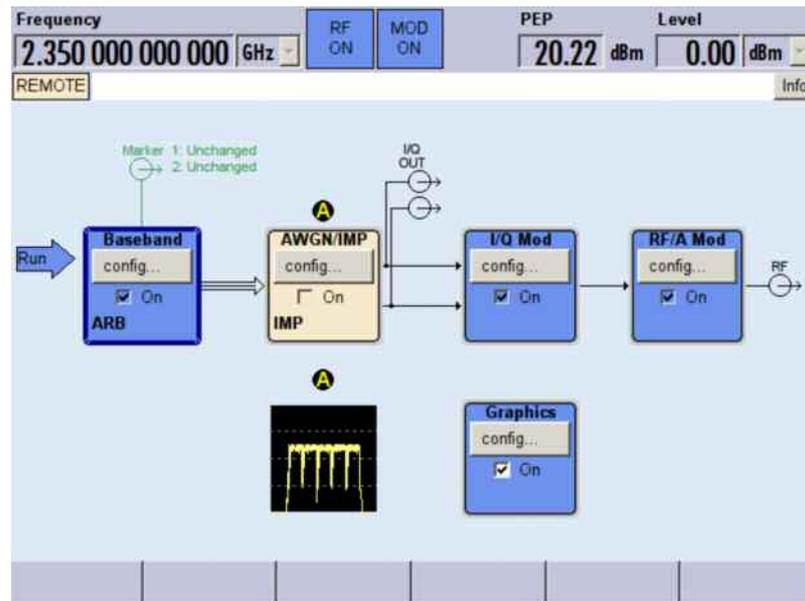
**Figure 33: Generating deployment scenario 2 or 3 (5x20 MHz carriers) with a single SMBV using the multi-carrier ARB mode.**
