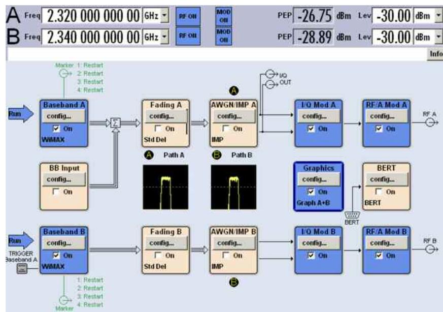
**Figure 16: SMU configuration for adding 2 WIMAX 802.16e carriers at RF A and RF B externally with an RF power combiner.**
