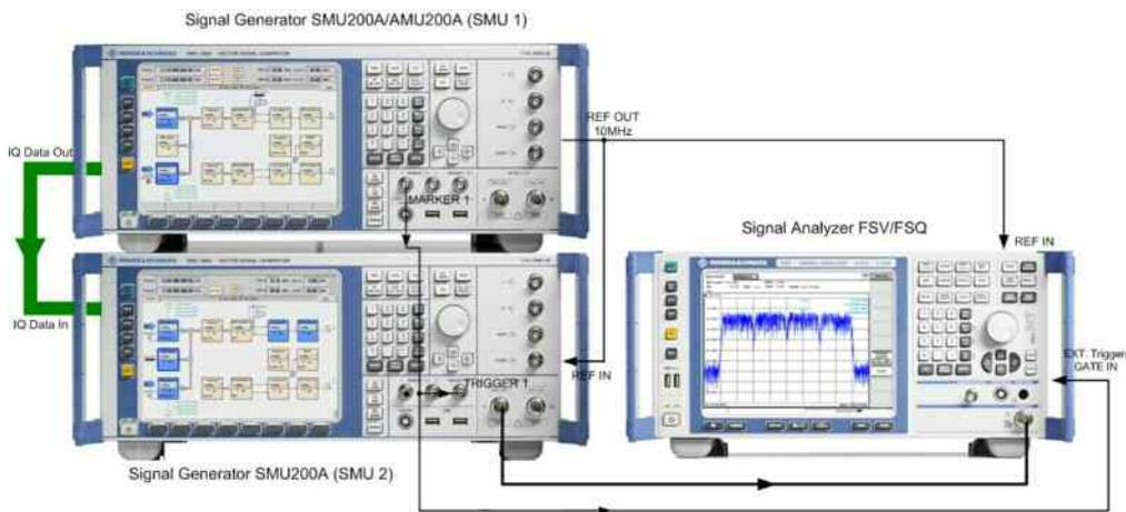
Figure 18: Combining the digital baseband output signal of a second generator
