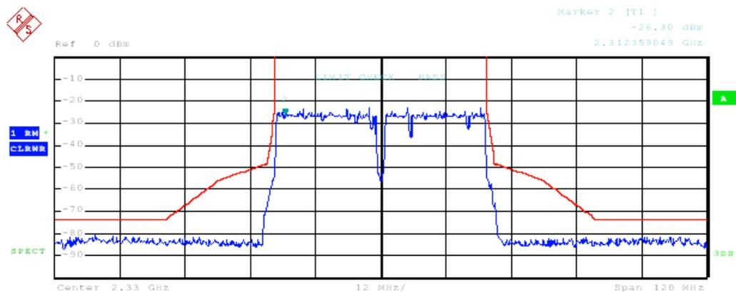
**Figure 46: Spectrum emission mask measurement with an FSQ on a contiguously placed 802.16m signal (2 x 20 MHz carriers) generated by an SMU**
