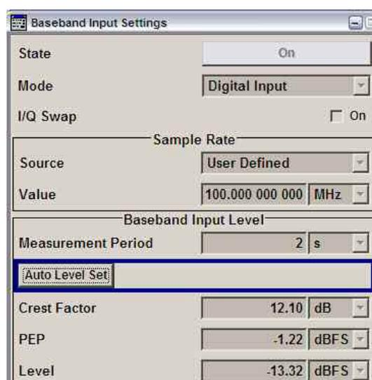
**Figure 21: Baseband input settings of SMU2. The sample rate is set to 100 MHz.**
