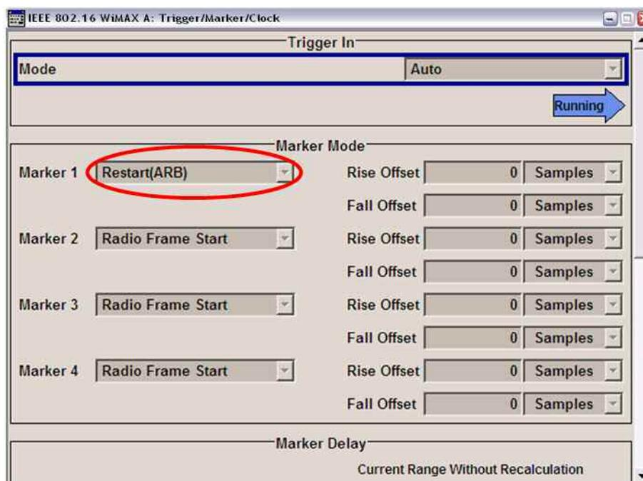
**Figure 20: Marker/Trigger Settings of SMU1. Marker 1 is set to Restart(ARB) to get a trigger signal for SMU2 of Figure 18.**
