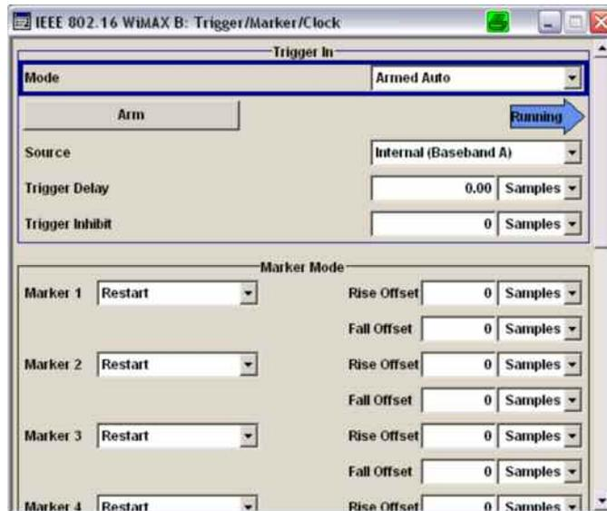
Figure 11: Trigger In of baseband B is set to trigger source Internal (baseband A) in mode Armed Auto, to start baseband A and B synchronously.
