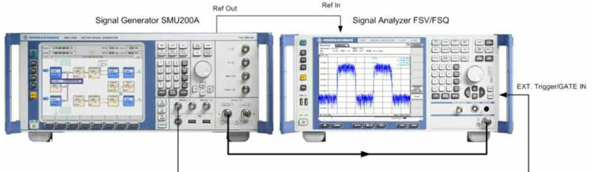
**Figure 7: Test setup for generating a 2-carrier 802.16m signal in contiguous or distributed mode (addition in baseband)**
