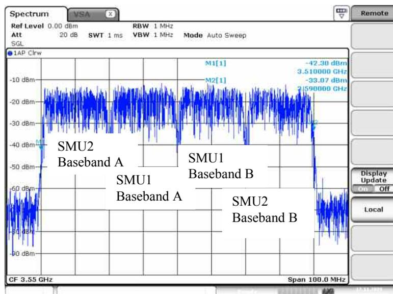
Figure 24: Example carrier aggregation in operating band 24. Up to 4 WIMAX 802.16e carriers with 20 MHz bandwidth each are combined to the SMU's RF A output.
