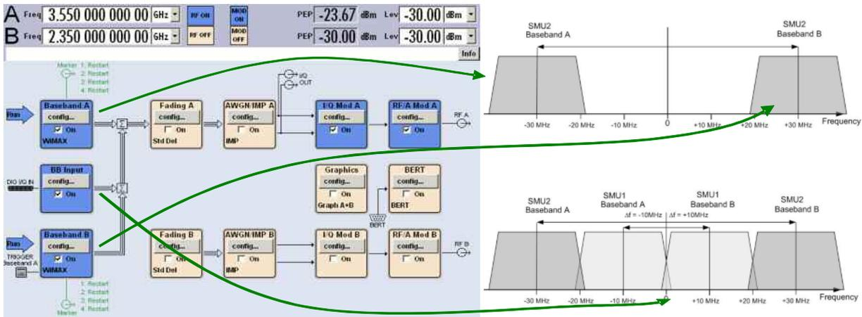
**Figure 22: The SMU2 digital baseband input receives the digital baseband signal of SMU1 and combines it with its own baseband A and B to a signal with 4 continuously placed carriers.**
