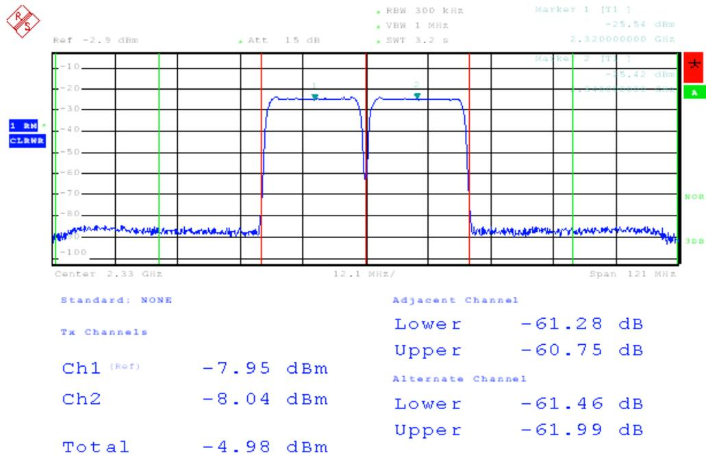
**Figure 45: Multi-carrier ACLR measurement of FSQ on two 802.16e signal (2 carriers each with 20 MHz bandwidth)**
