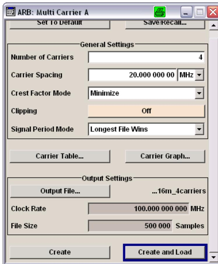
Figure 28: SMU/SMBV Screen detail: The 4-carrier signal is created and loaded via "Create and Load"
