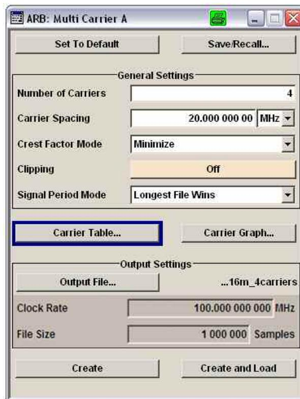
**Figure 26: SMU/SMBV screen detail: setup the multi-carrier signal with 4 carriers with a spacing of 20 MHz**
