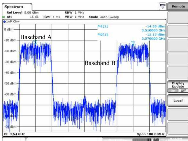
Figure 14: Distributed placement of 2 WIMAX 802.16e carriers with 20 MHz bandwidth each within the WIMAX 802.16e frequency band 3.5 GHz (addition in baseband).
