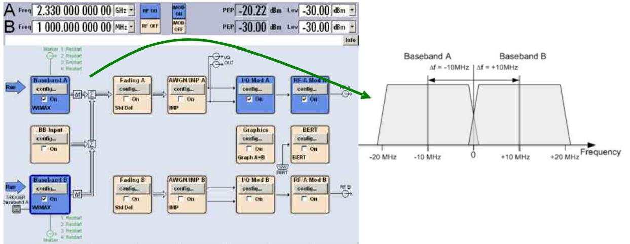
**Figure 10: Baseband B is routed to baseband A to produce a contiguously placed 802.16m signal containing two carriers with 20 MHz bandwidth each.**
