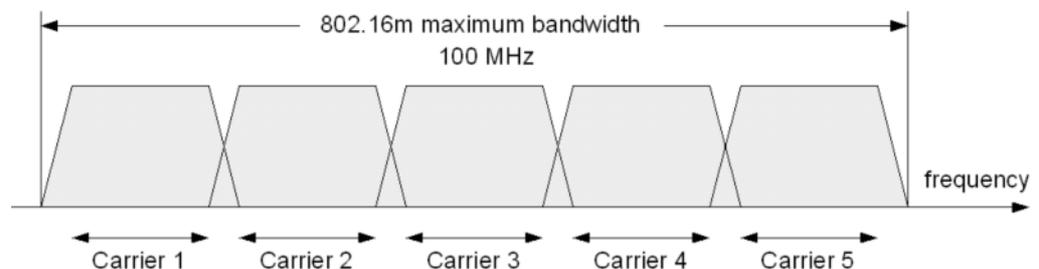
**Figure 1: 802.16m maximum bandwidth in contiguous deployment**
