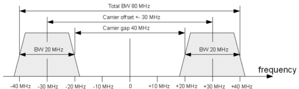
Figure 6: Two carriers with 40 MHz gap
