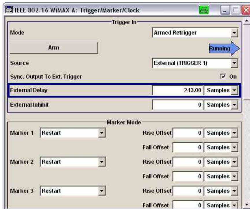
Figure 23: Trigger Settings of SMU2. Adjust External Delay to the same Trigger to Frame Start Offset as the SMU1 signal has.
