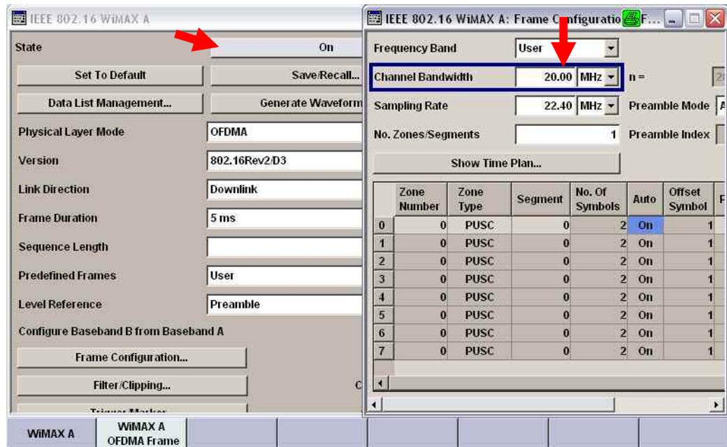
**Figure 8: Generating an WIMAX 802.16e Signal with 20 MHz bandwidth**
