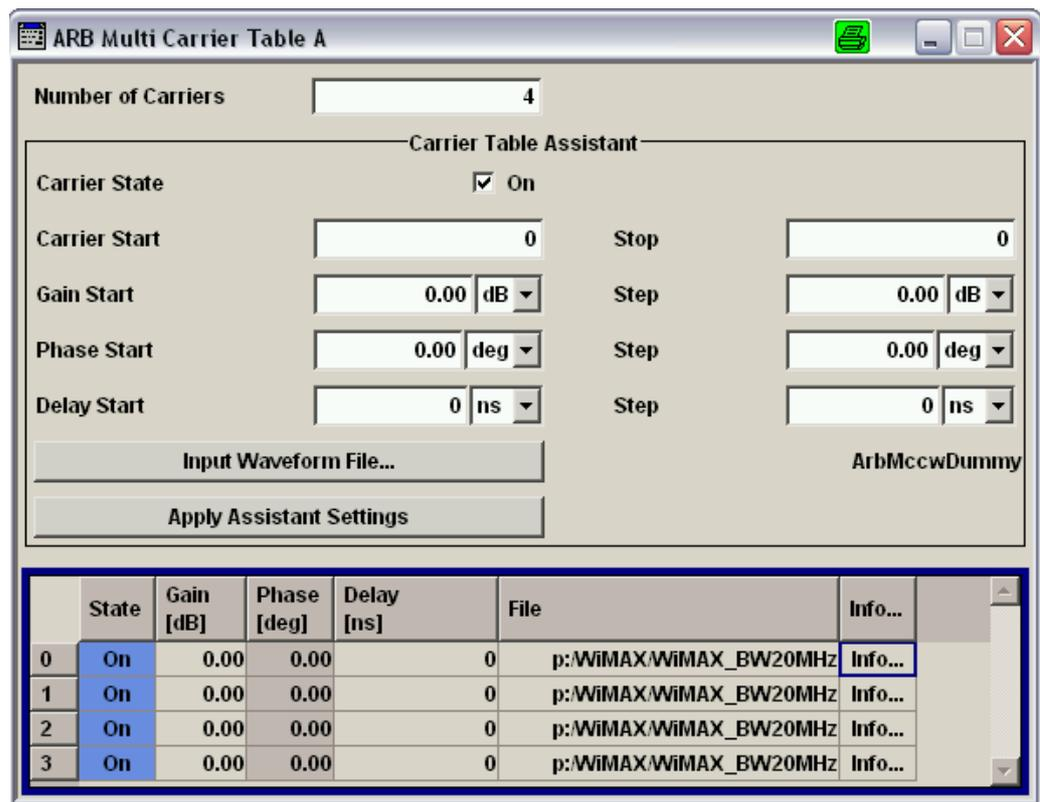
Figure 27: SMU/SMBV Screen Detail: multi-carrier table configuration
