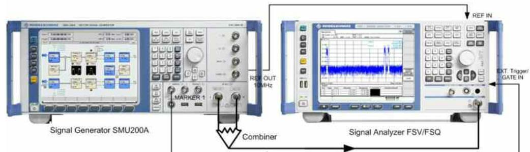
Figure 35: Test setup with a 2-channel SMU200A (2 baseband modules, 2 RF modules)
