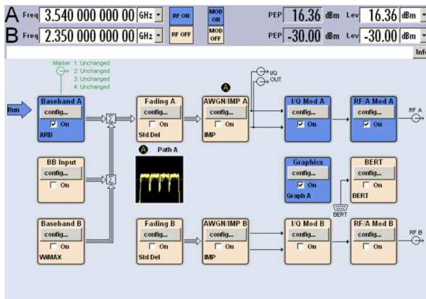
Figure 29: SMU Screen: 802.16m signal with 4 contiguously placed carriers, each with 20 MHz bandwidth using the Multi-carrier arbitrary Waveform mode.
