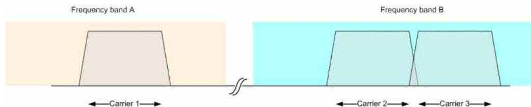
**Figure 2: 802.16m distributed spectrum deployment**
