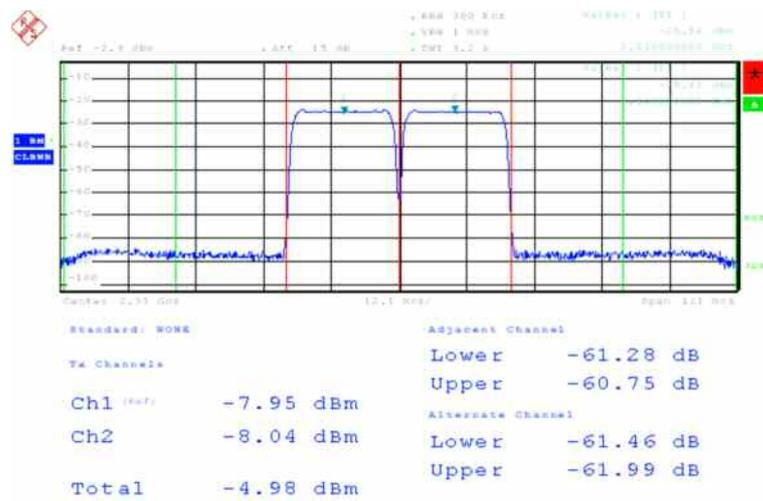
**Figure 17: ACLR performance of 2 contiguously placed carriers with 20 MHz bandwidth each, measured with an FSQ.**
