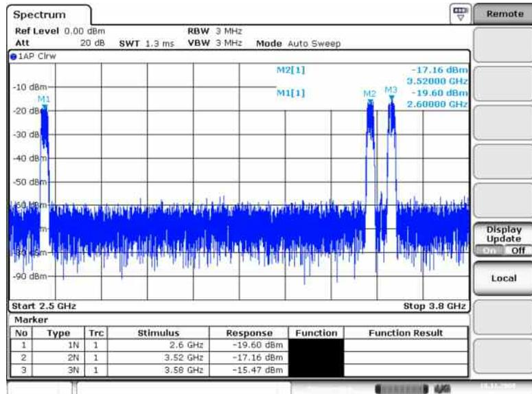
Figure 37: Example multi-band distributed spectrum allocation at band 7 (2.6 GHz) and at band 41 (3.5 GHz) (scenario 12 of Table 1) generated with a 2-path SMU.
