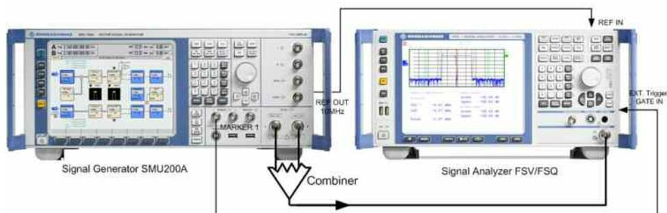
Figure 15: Adding 2 RF channels of an SMU externally with a power combiner to generate 2 WIMAX 802.16e carriers
