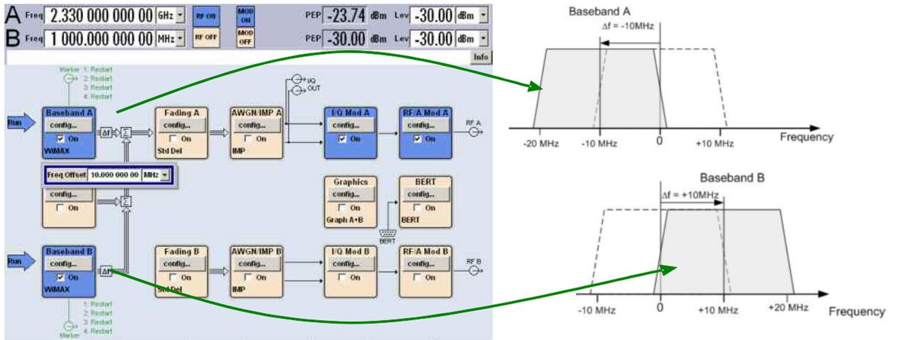
**Figure 9: Baseband A is set to a frequency offset of -10 MHz, baseband B to a frequency offset of +10MHz.**
