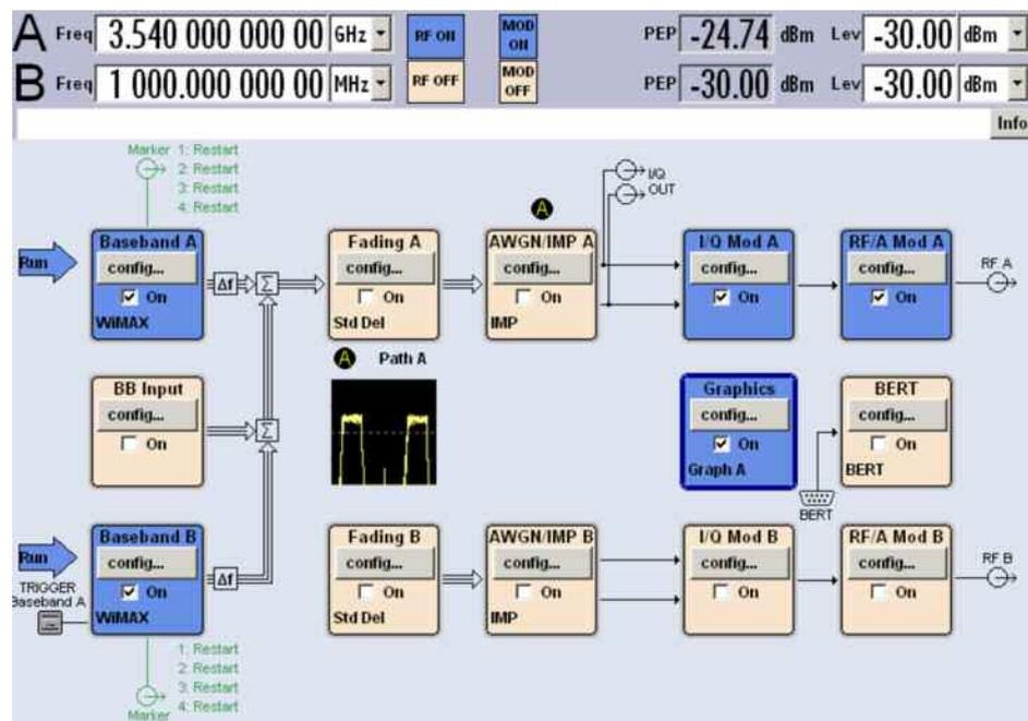
Figure 13: SMU Screen: Combining 2 baseband signals distributed in an SMU (addition in baseband)
