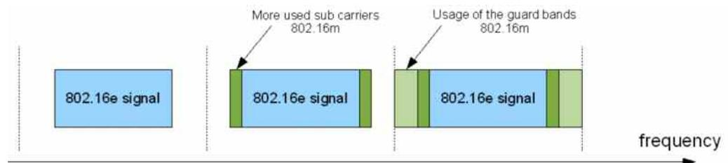
Figure 3: usage of the guard bands in 802.16m
