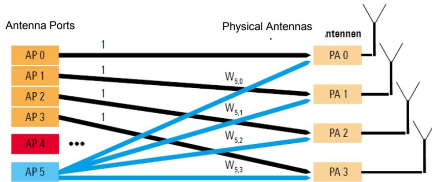
Figure 13: Mapping of logical antenna ports to physical transmit antennas (3GPP Release 8)
