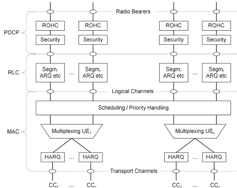
**Figure 11: Downlink layer 2 structure [3]**
