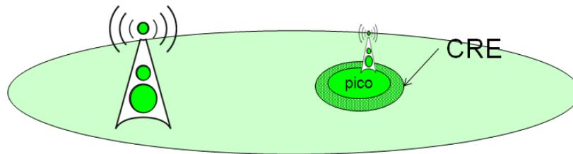
**Figure 21: Example cell layout of a heterogeneous network using a pico cell within a macro cell**
