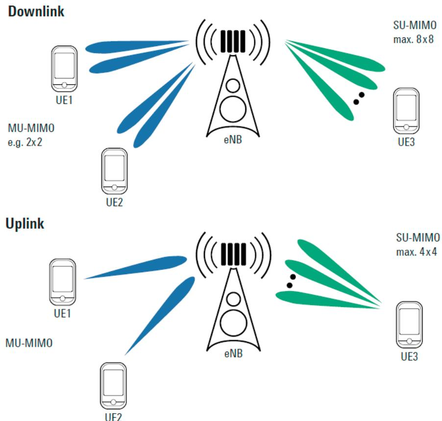
Figure 14: Supported transmit layers in LTE-Advanced
