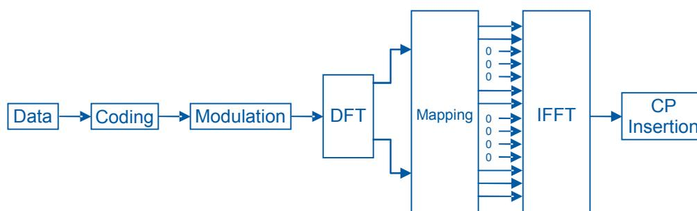
Figure 17: Block diagram for clustered SC-FDMA
