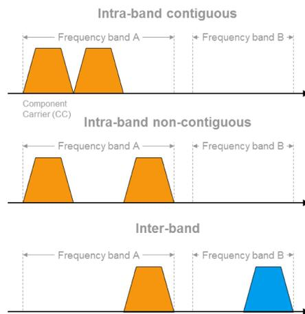
Figure 6: LTE-Advanced spectrum deployment
