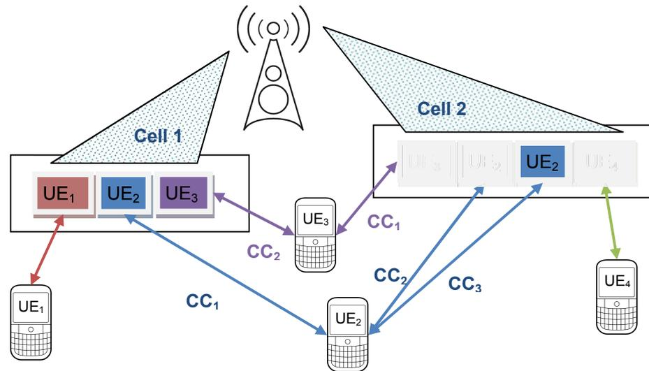
**Figure 4: LTE-Advanced maximum bandwidth in contiguous deployment**
