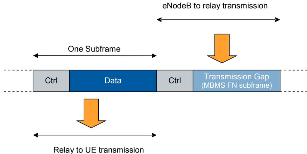
**Figure 25: Example of relay-to-UE communication using normal subframes (left) and eNodeB-to-relay communication using MBSFN subframes (right)**
