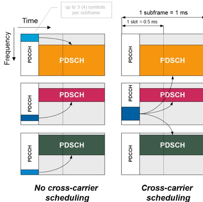
Figure 9: Cross carrier scheduling in comparison to LTE Release 8
