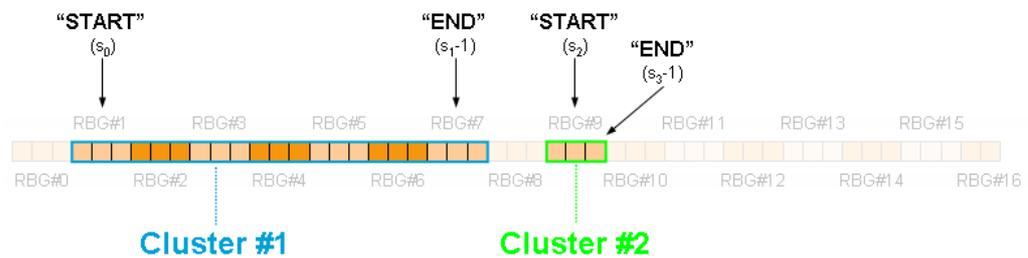
Figure 18: Example for a two-cluster allocation for a 10 MHz (50 RB) signal
