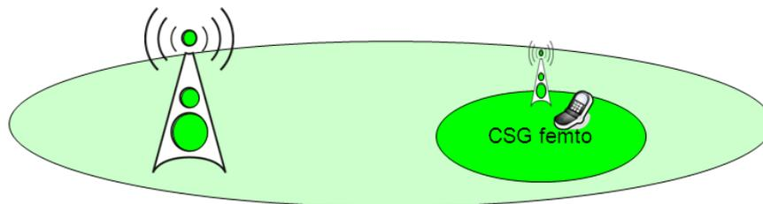
**Figure 22: Interference scenario for Femto cells**
