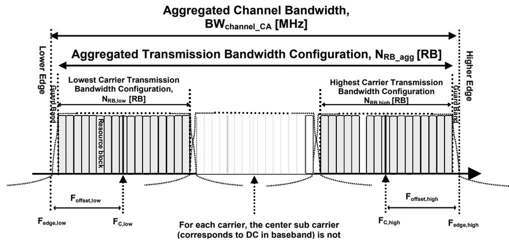
Figure 7: Definition of Aggregated channel bandwidth and aggregated channel bandwidth edges [5]
