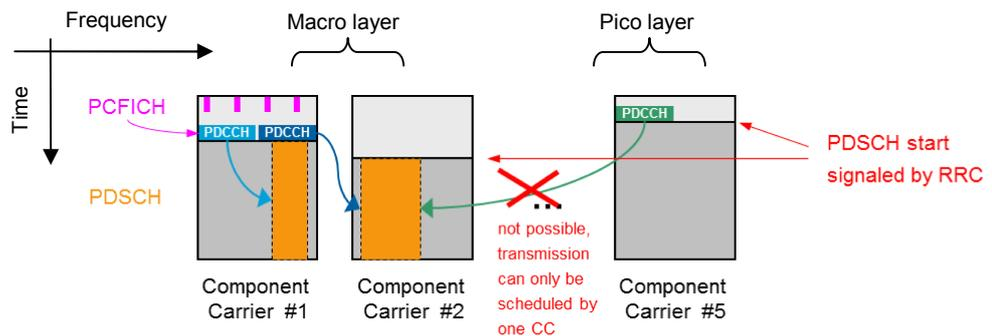
Figure 10: Cross carrier scheduling for support in heterogeneous networks
