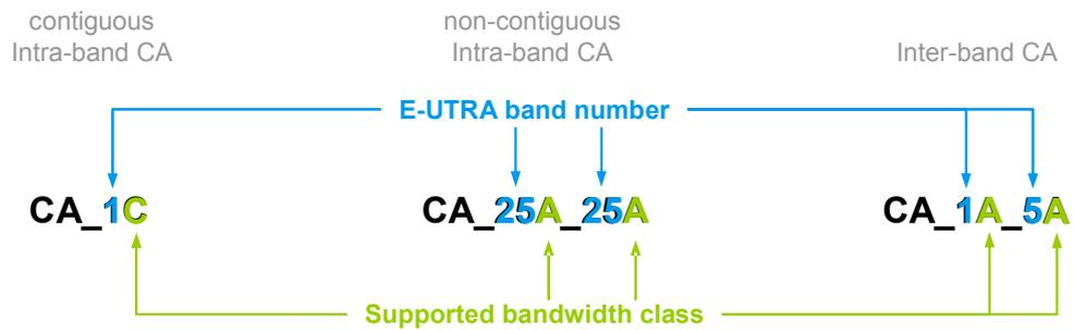
Figure 8: Notation of carrier aggregation support (type, frequency band, and bandwidth)
