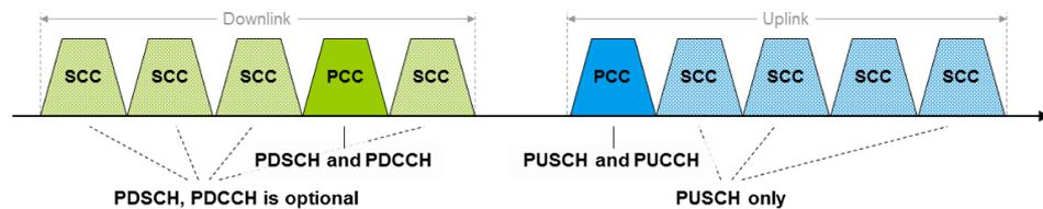
**Figure 5: Channel allocation on PCC and SCC**
