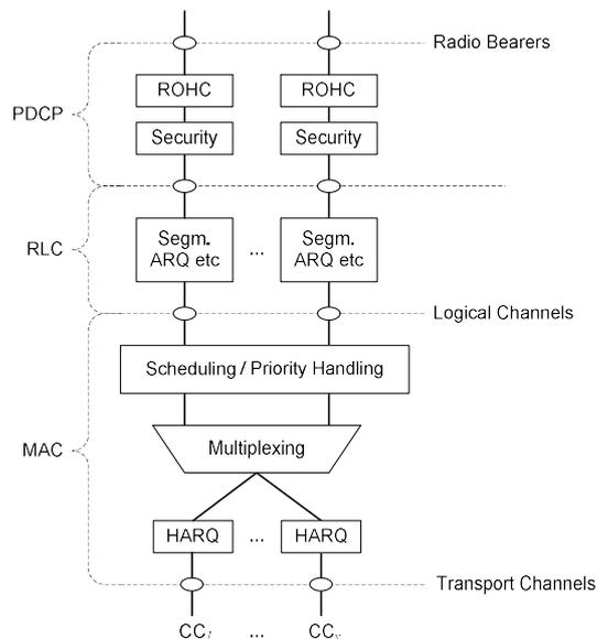
**Figure 12: Uplink layer 2 structure [3]**
