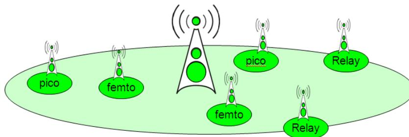
**Figure 20: Example cell layout of a heterogeneous network**
