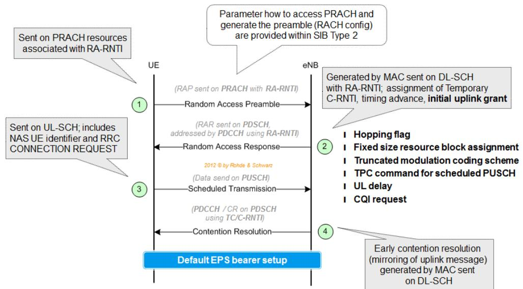
Figure 2: LTE attach procedure
