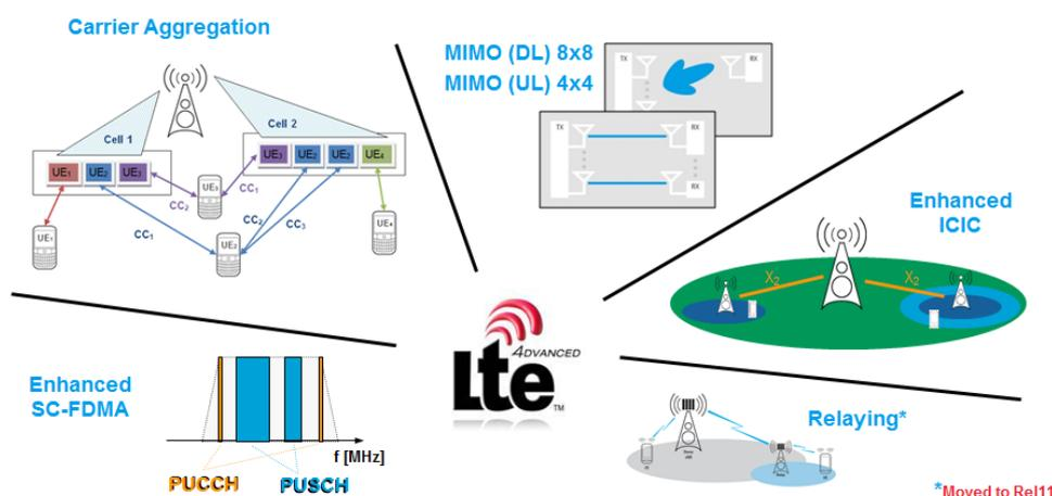
Figure 1: Main LTE-Advanced technology components (overview)
