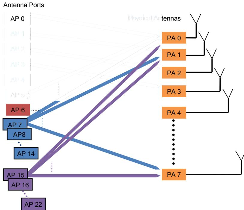
Figure 15: Mapping of logical antenna ports to physical transmit antennas (3GPP Release 10)
