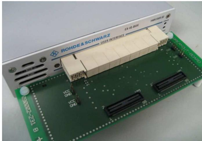
Figure 70: Differential breakout board
