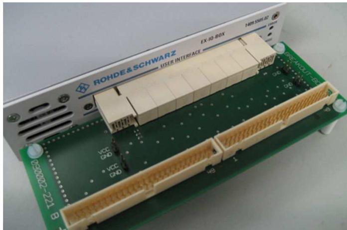
**Figure 69: Single-ended breakout board**
