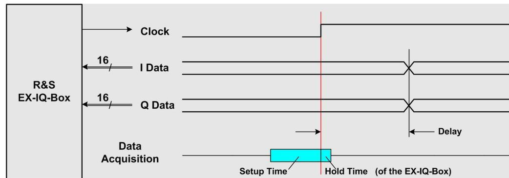
Figure 64: Case 4 - RX, internal clock
