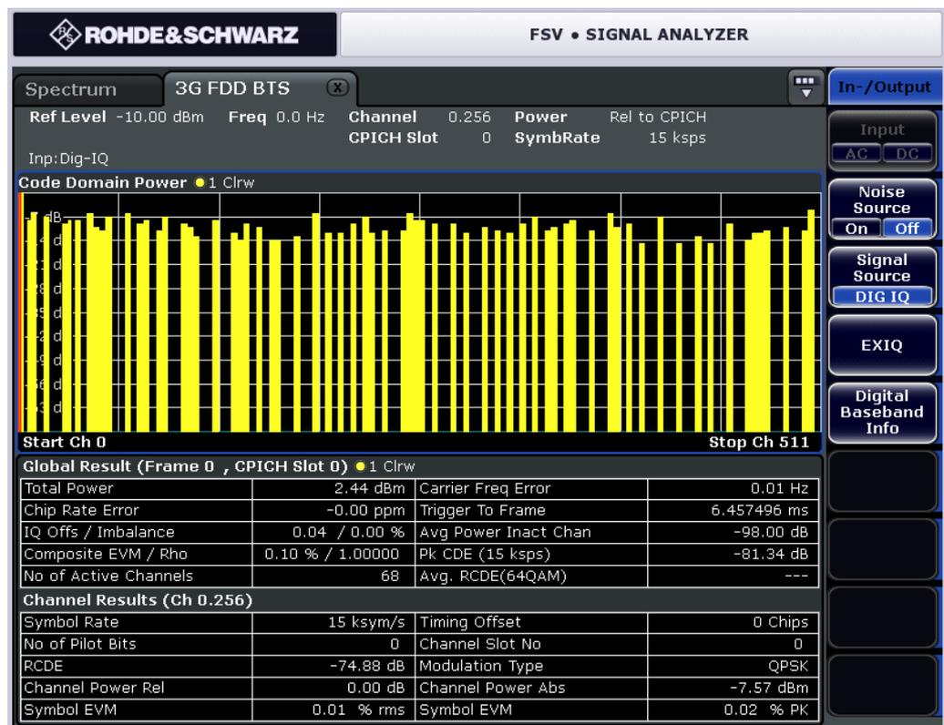
Figure 43: Dig. IQ Data Evaluation by the 3GPP BTS option
