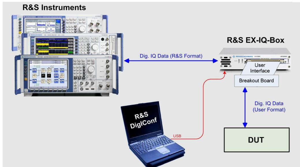
**Figure 1: The R&S EX-IQ-Box as an interface between R&S-formatted and user-formatted IQ data**
