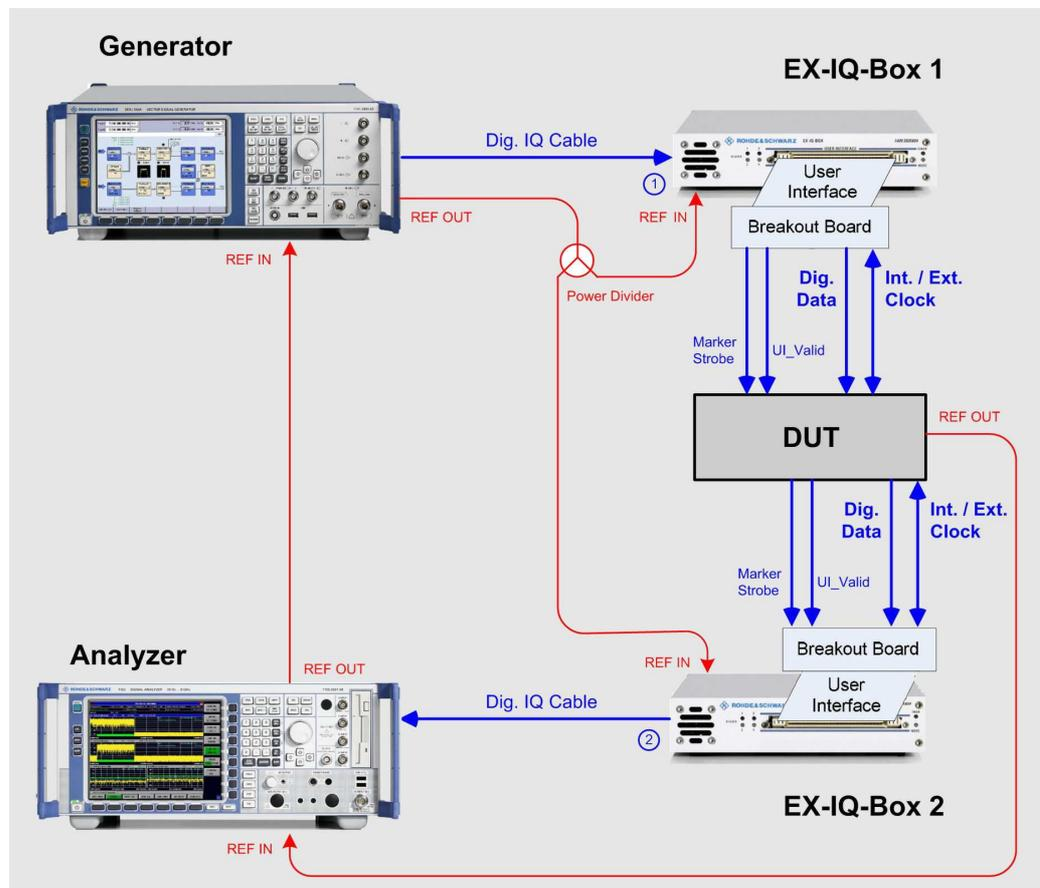
Figure 53: DUT between the IQ transmitter and IQ receiver
