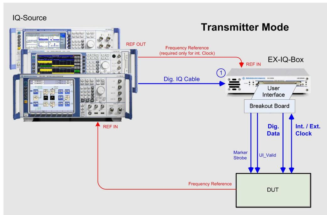
Figure 23: Instruments and signals in transmitter mode
