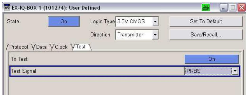
**Figure 56: TX Test: Select the pattern and go**
