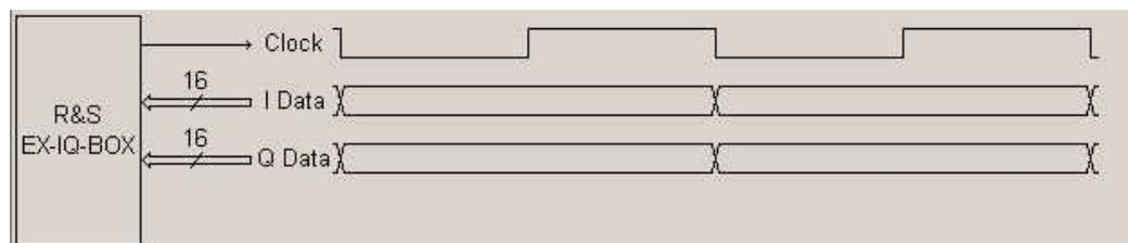
**Figure 58: Safe Clock Phase for low data rates**
