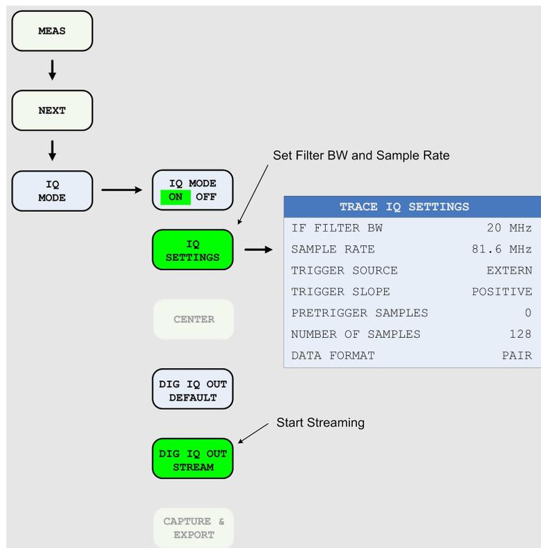
**Figure 31: Analyzer configuration for IQ streaming**
