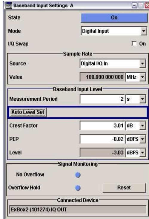
Figure 46: Configuring the R&S AMU baseband input
