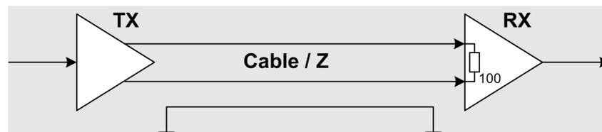
**Figure 65: Differential data transmission**
