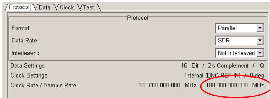
**Figure 29: Where to get the Sample Rate value**
