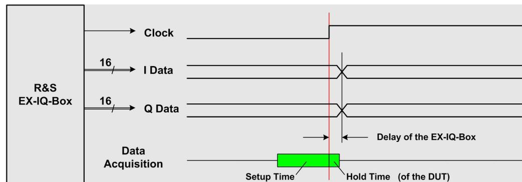
**Figure 59: Case 1 - TX, internal clock**
