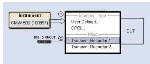
Figure 18: Selecting a transient recorder
