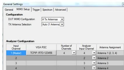
Figure 2-22: Using the RTO for MIMO measurements
