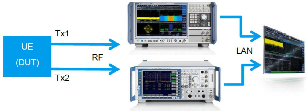
Figure 2-32: Test setup for measuring a 2x2 uplink MIMO signal
