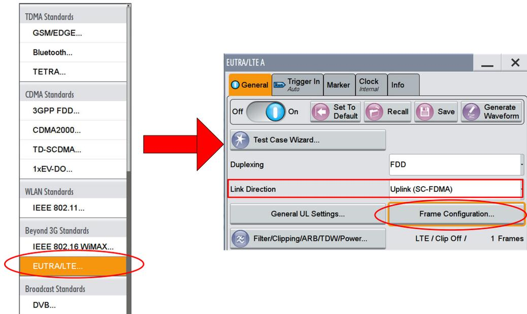
The **General** section allows selecting either LTE Rel 8/9 or LTE Rel 10. When using Rel 10 per UE the content field shows simultaneous PUCCH and PUSCH. Two sets of resource blocks can be configured in accordance with 3GPP specifications as illustrated in [Figure 2-15](#).
