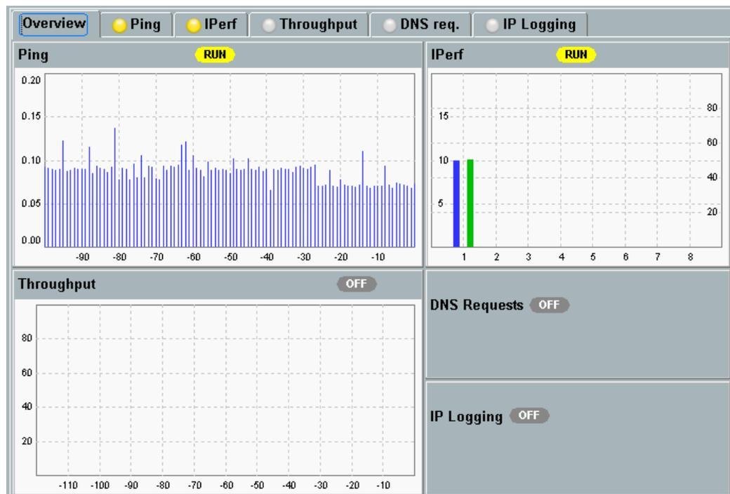
Figure 2-44: Overview of the tests in the data application unit. PING, IPPerf and Throughput at a glance.
