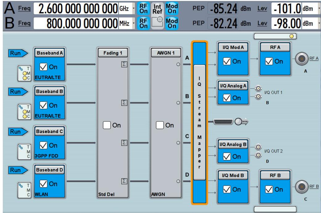
Figure 2-7: SMW example with four different signals
