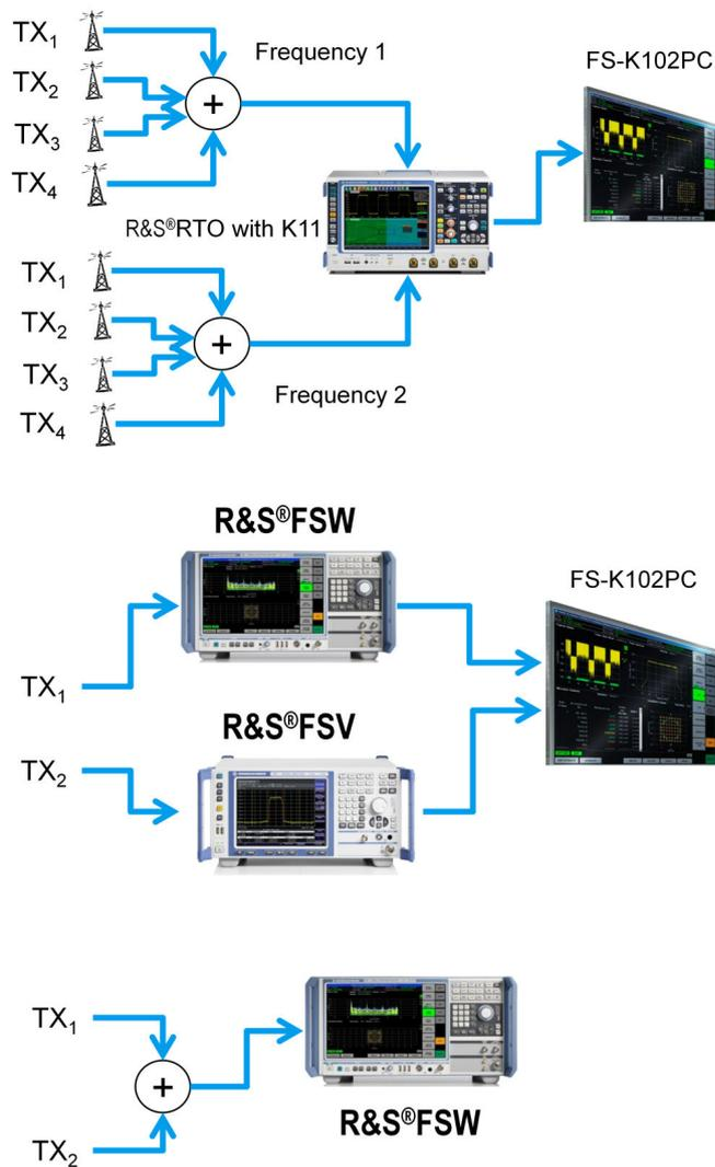
Figure 2-28: different setups measuring TAE for carrier aggregation
