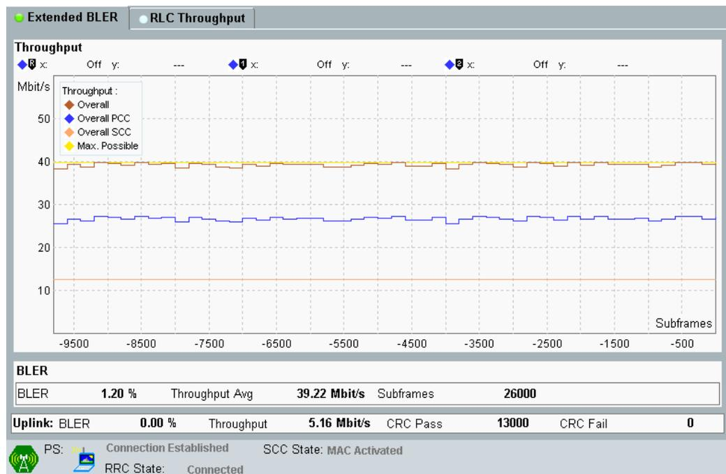
Figure 2-43: LTE RX measurement for Carrier Aggregation. The throughput for both CCs and the overall throughput are displayed.
