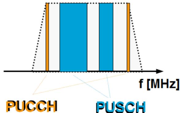
Figure 2-3: Simultaneous PUCCH/PUSCH and clustered uplink operation
