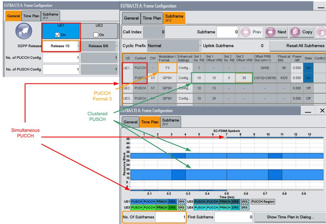
Figure 2-15: Configuring Clustered PUSCH and simultaneous PUCCH/PUSCH
