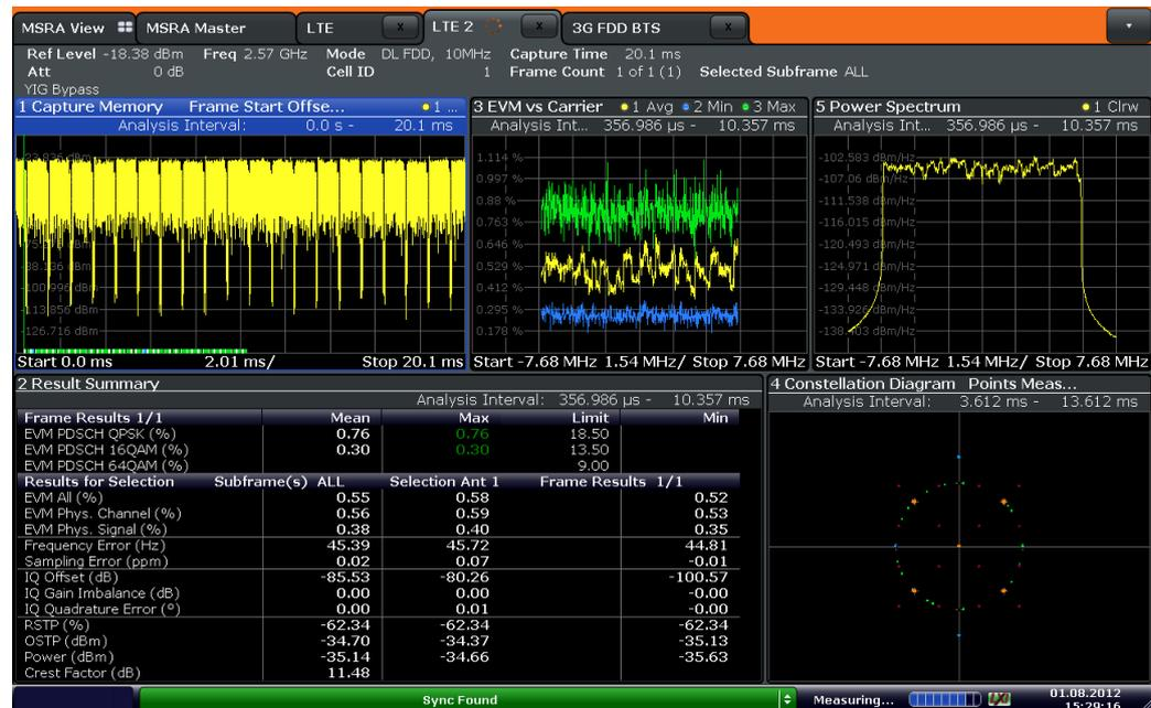
Figure 2-23: LTE measurements on a single component carrier using FSW-K100
