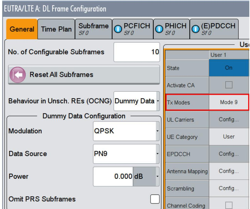
Figure 2-16: SMW: TM9 settings in the general DL frame configuration
