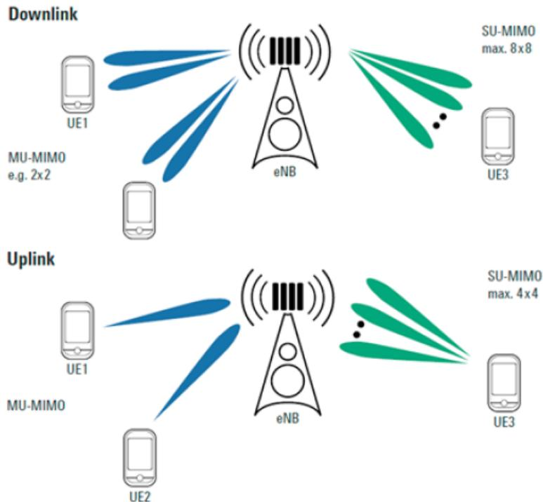
Figure 2-5: Supported transmit layers in LTE-Advanced
