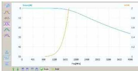
**Figure 11: Insertion loss + input VSWR**
