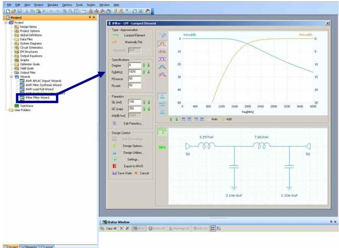
Figure 5: AWR® iFilter™ filter synthesis wizard
