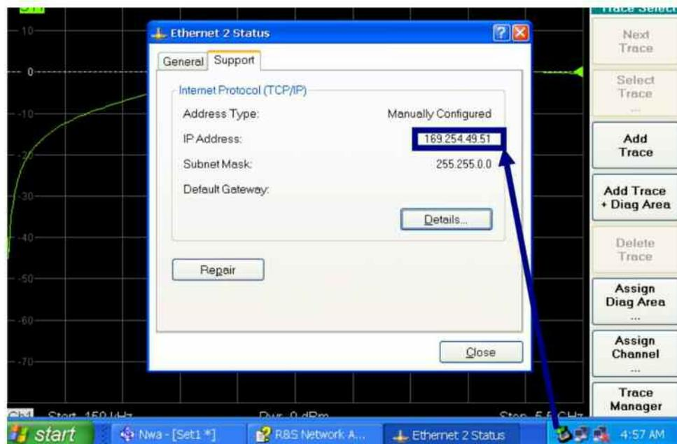
Figure 25: Acquiring the IP address of the R&S<sup>®</sup> ZVB
