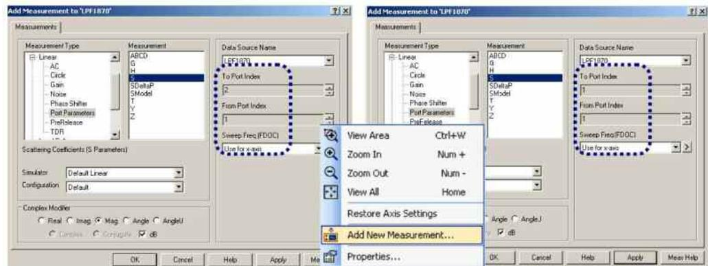
**Figure 16: Adding new measurements to the graph by right click**
