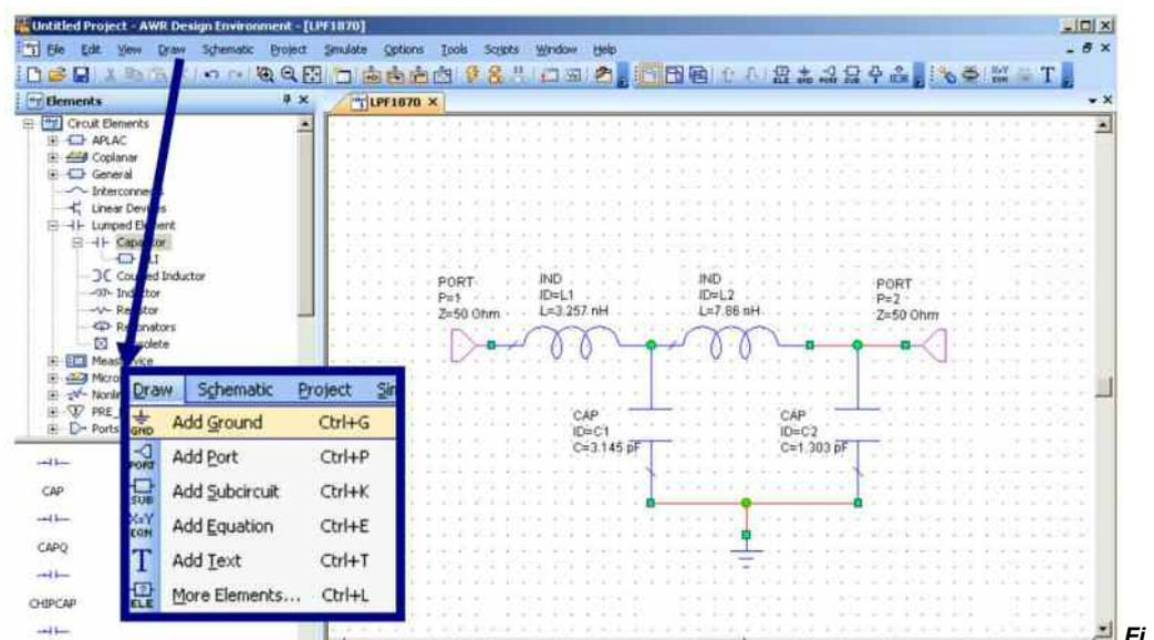
**Figure 4: Adding grounds and ports to the circuit**
