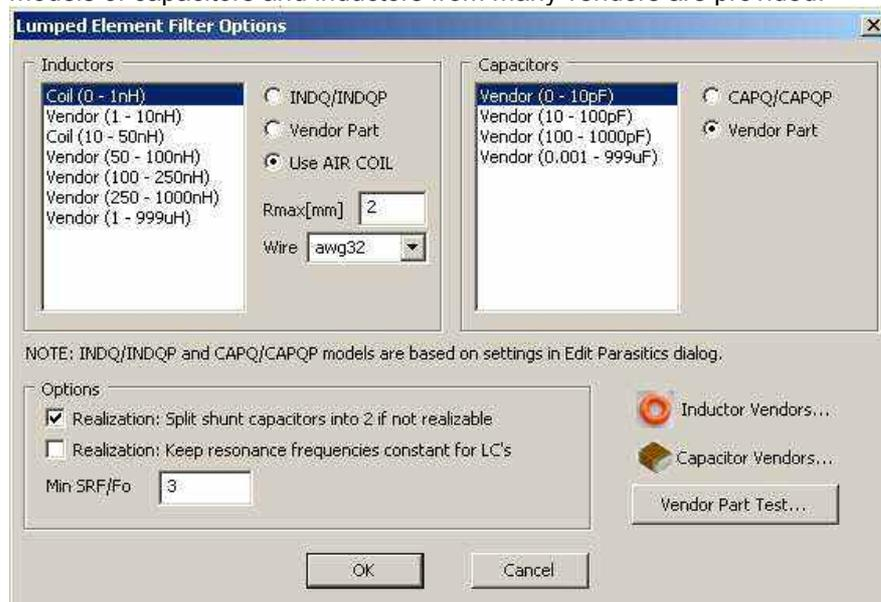
Figure 7: Lumped element filter options
