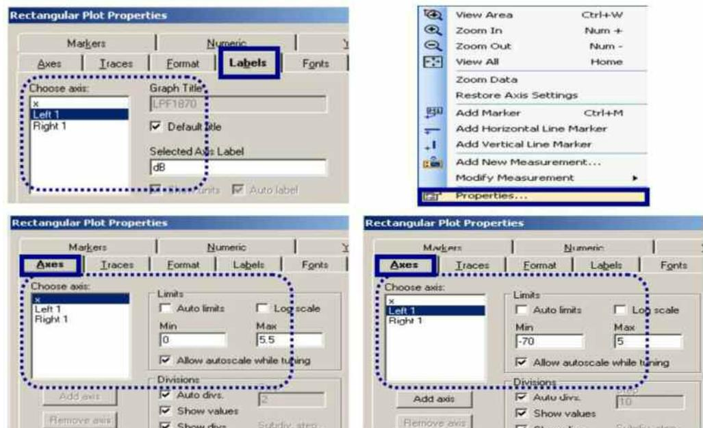
Figure 18: Graph properties for adjusting the scaling and labeling of the axes
