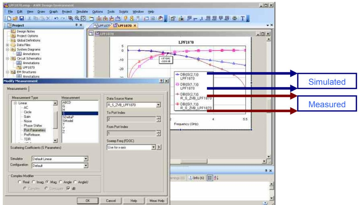
Figure 28: Appending an imported data source into a simulated graph
