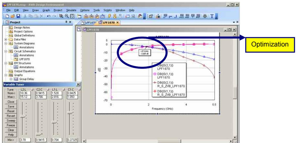
Figure 30: Optimizing simulated lumped elements
