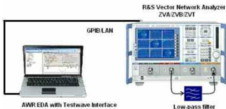
**Figure 2: Test setup for filter simulation and validation**
