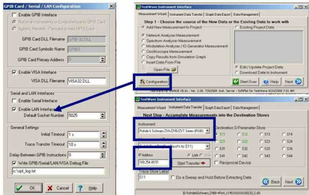
Figure 26: Configuration of transfer via LAN and type of measurement
