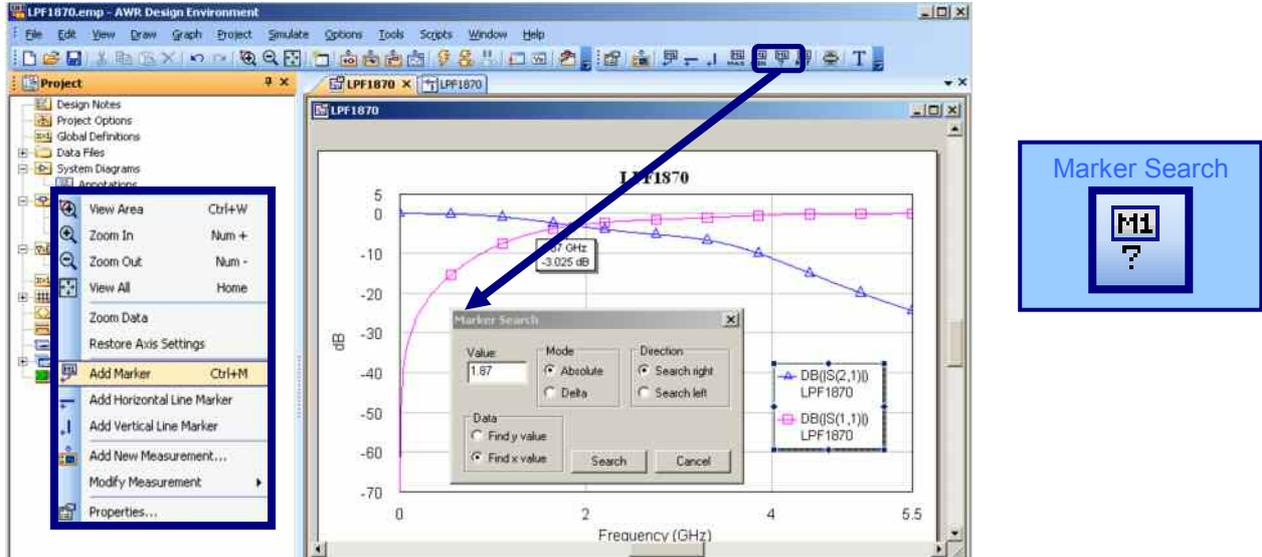
Figure 20: Adding markers and pointing markers to a specified location via "Marker Search"
