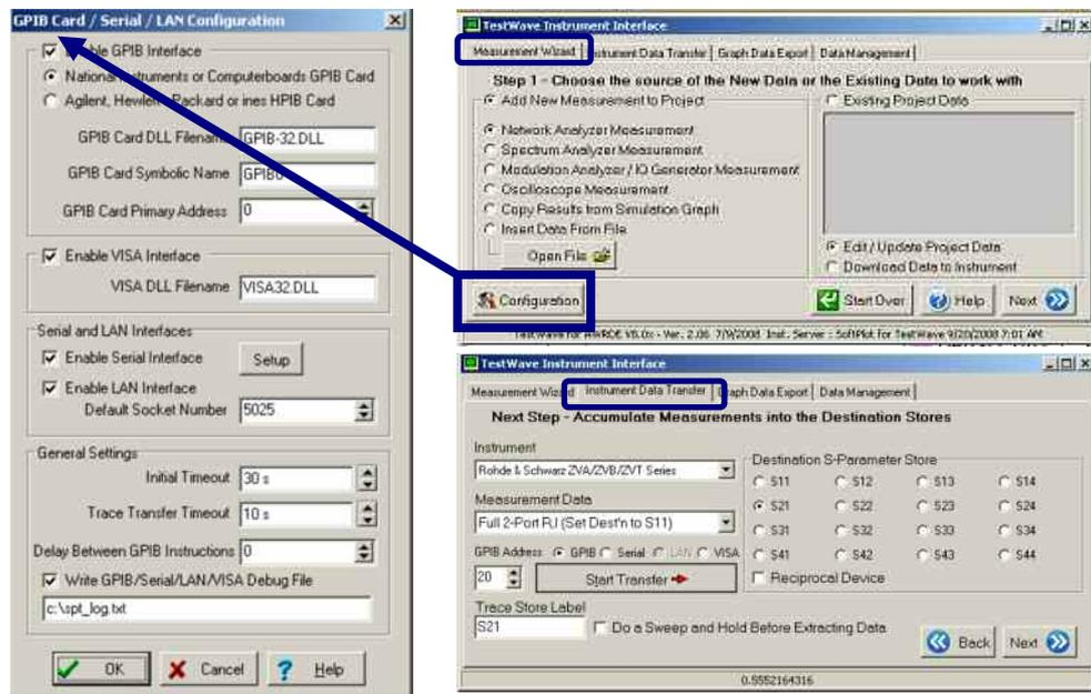
Figure 24: Configuration of transfer via GPIB and type of measurement
