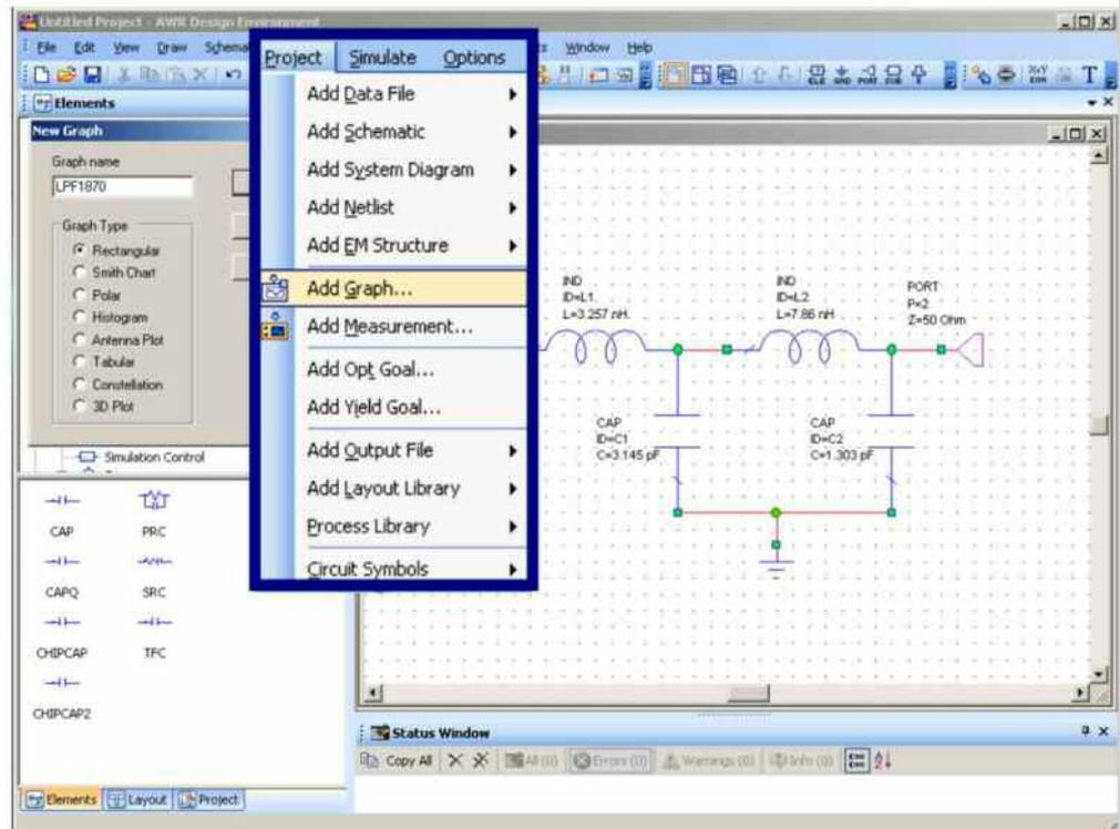
**Figure 15: Adding graphs and measurements to plot**
