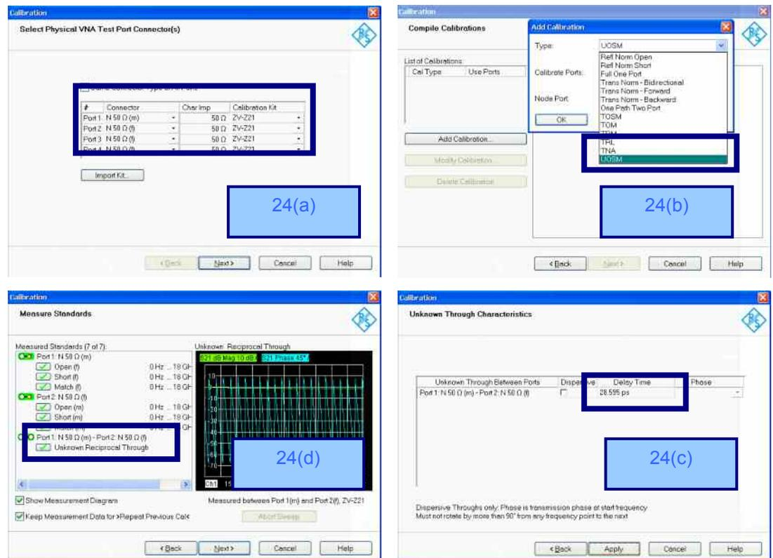
Figure 23: Calibration of R&S® ZVB vector network analyzer using the USOM method
