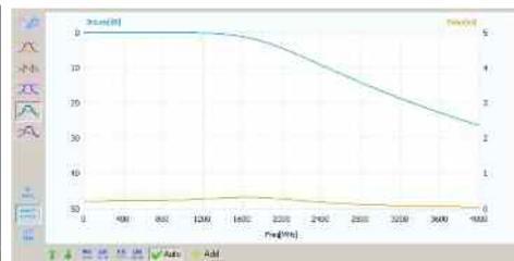
**Figure 12: Insertion loss + group delay**
