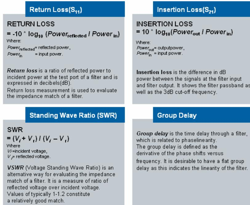
**Figure 22: Scorecard for filter measurement**
