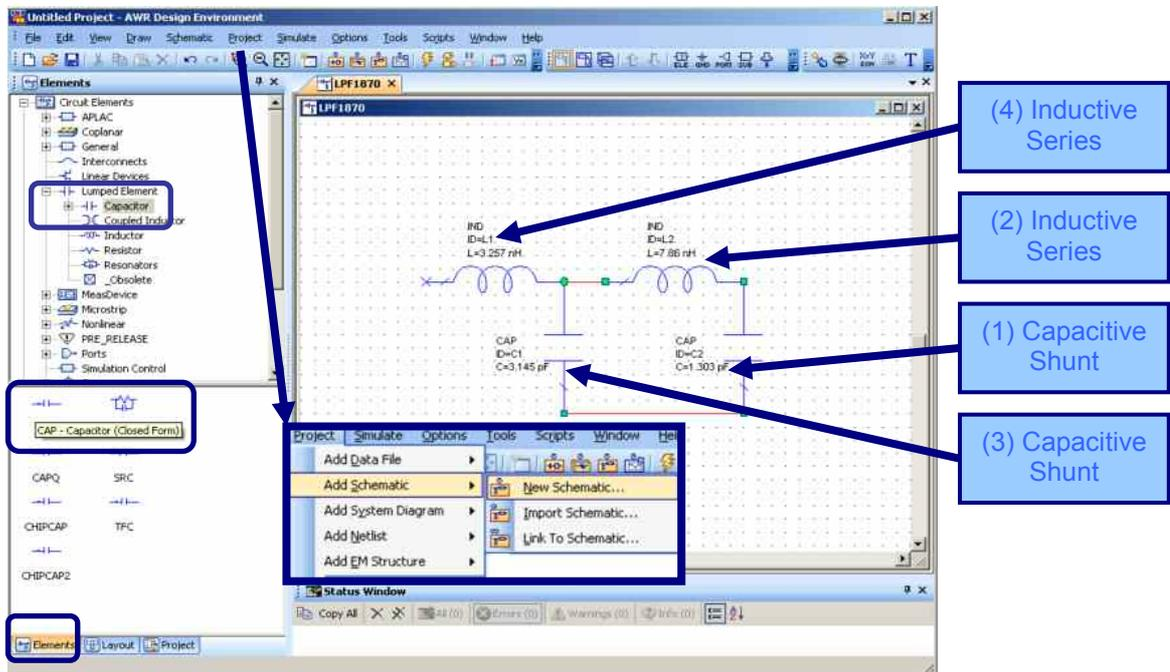
**Figure 3: Adding lumped elements into a schematic with values calculated from Table 1**
