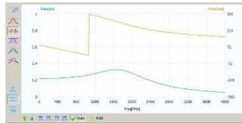
**Figure 10: Group delay + insertion phase**
