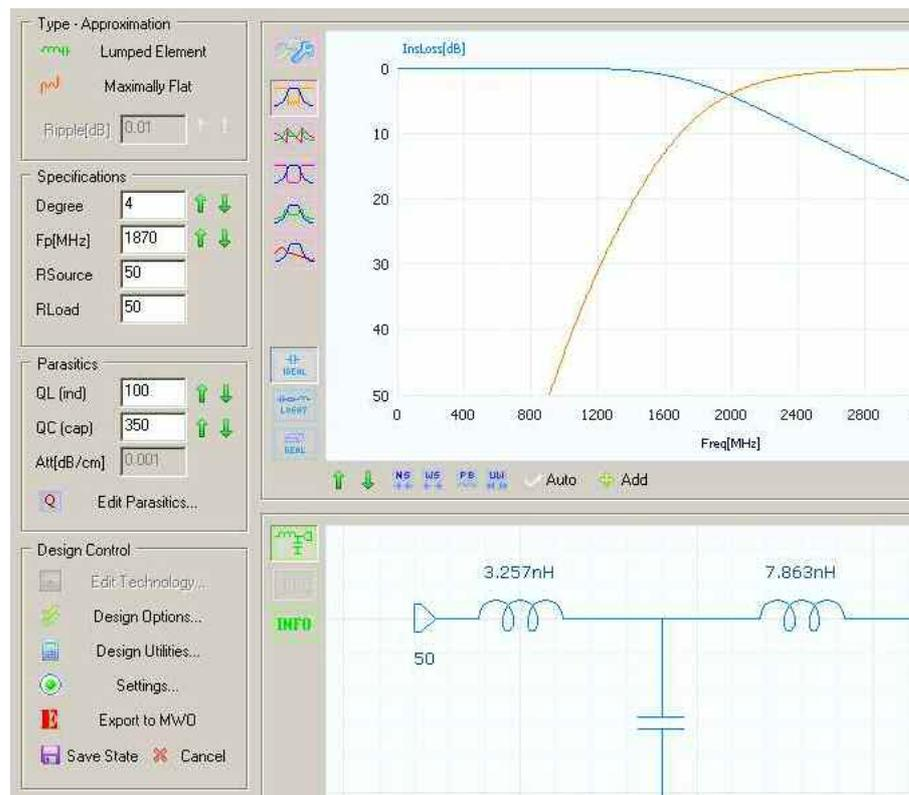
Figure 6: AWR® iFilter™ filter wizard – main filter design dialog
