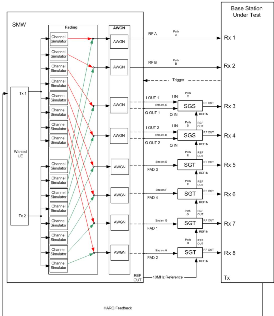
Fig. 3-42: Test setup for PUSCH test 8.2.1A for 8 antennas with one SMW
