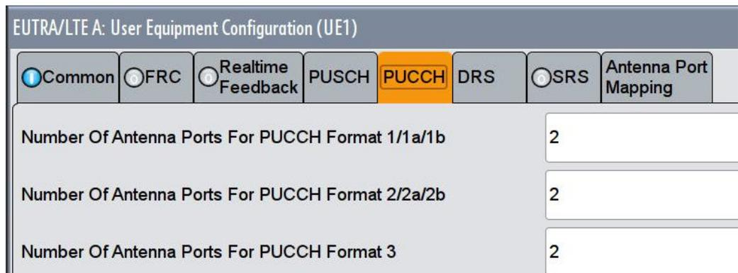
Fig. 3-145: Number of antenna ports for the different PUCCH formats is 2
