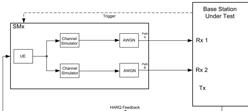
Fig. 3-77: Test setup for PUSCH test 8.2.7 for 2 antennas
