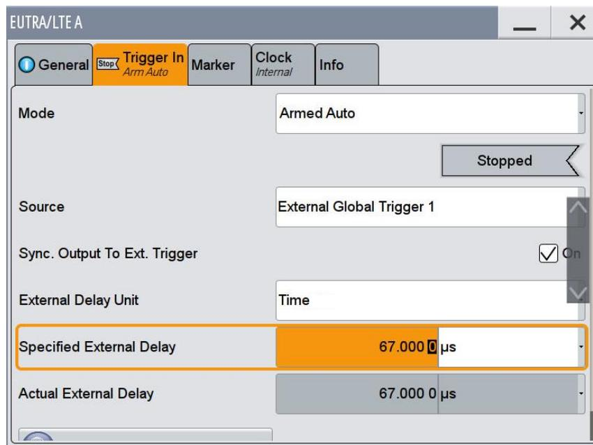
Fig. 3-238: NPRACH timing offset via trigger delay
