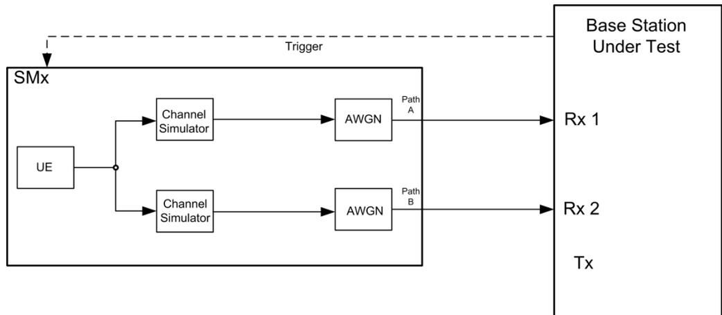
Fig. 3-206: Test Setup for PUCCH Test 8.4.1 for 2 Antennas
