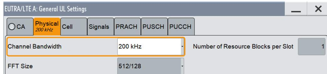
Fig. 3-10: NB-IoT standalone mode uses 200 kHz bandwidth
