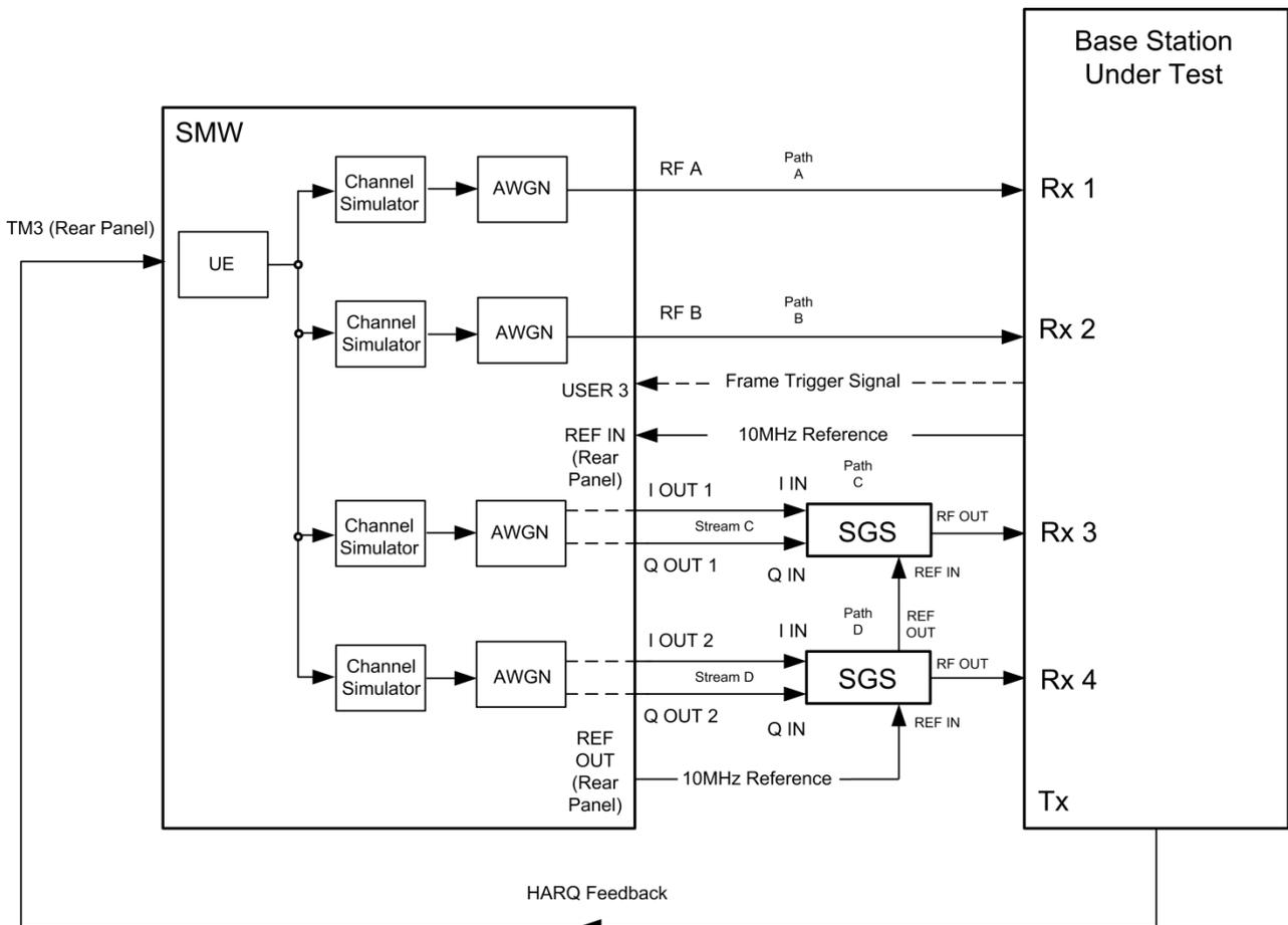
Fig. 3-34: Test setup for PUSCH test 8.2.1 for 4 antennas with one SMW
