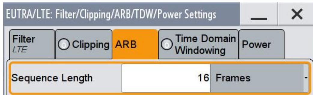
Fig. 3-226: 16 frames to generate the pattern continuously
