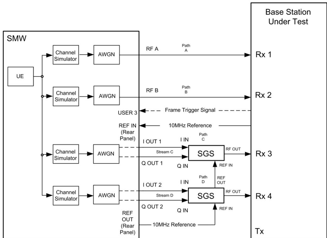
Fig. 3-132: Test setup for PUCCH test 8.3.6 for 4 antennas with one SMW
