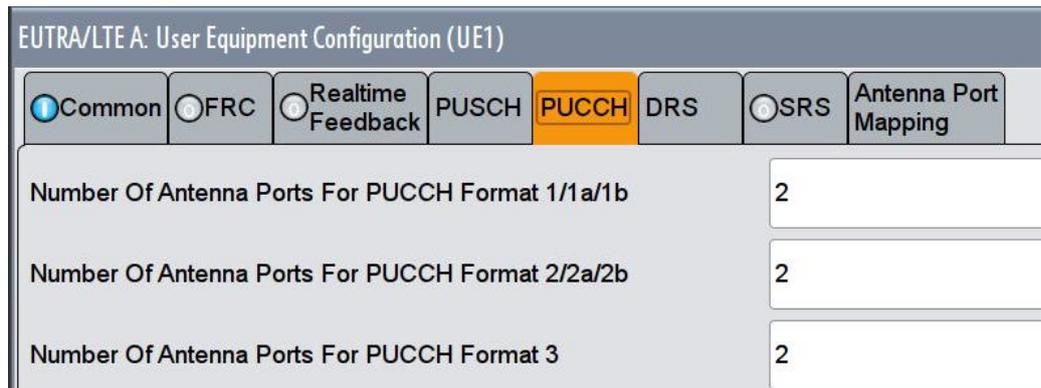
Fig. 3-164: Number of antenna ports for the different PUCCH formats is 2
