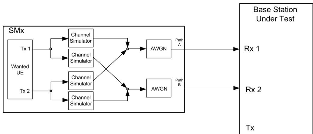
Fig. 3-141: Test setup for PUCCH test 8.3.7 for 2 antennas
