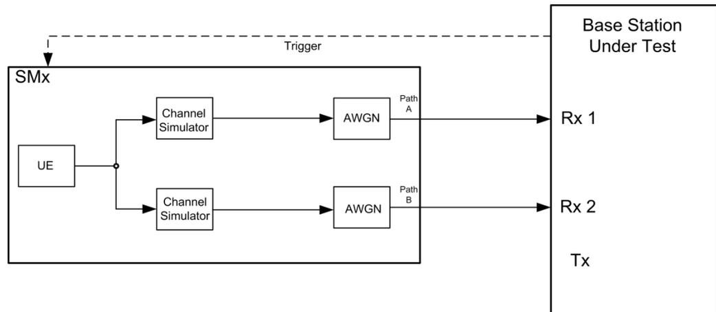
Fig. 3-63: Test setup for PUCCH test 8.2.3
