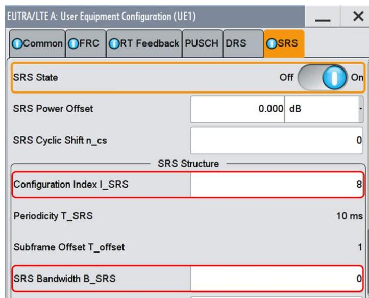
Fig. 3-57: Setting the SRS parameters in the UE
