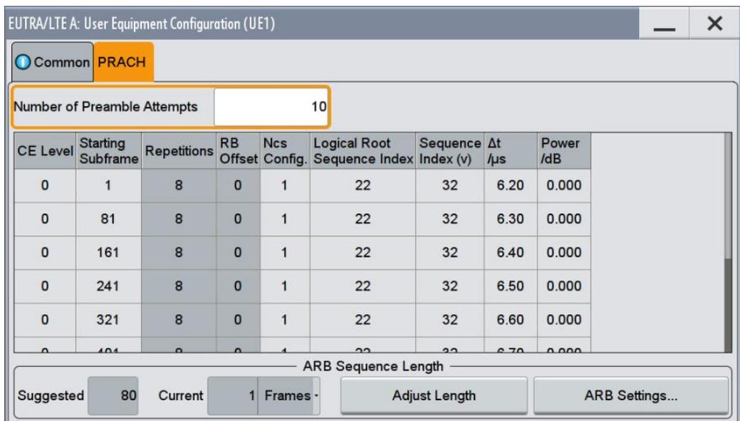
Fig. 3-218: Details of the Test Preambles.
