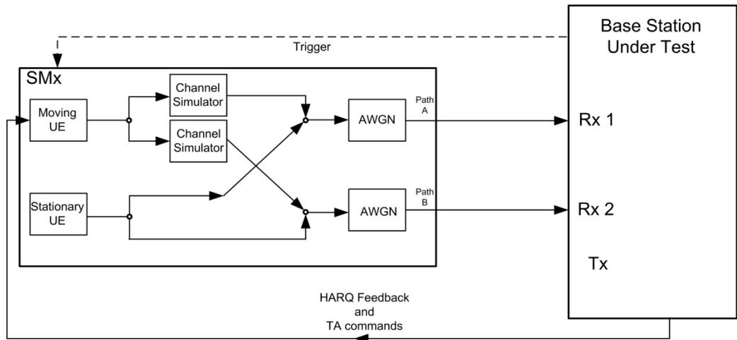
Fig. 3-50: Test setup for test 8.2.2
