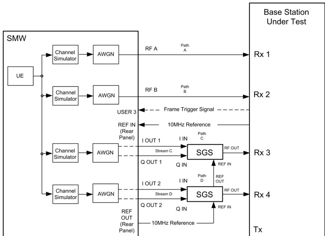
Fig. 3-112: Test setup for PUCCH test 8.3.4 for 4 antennas with one SMW
