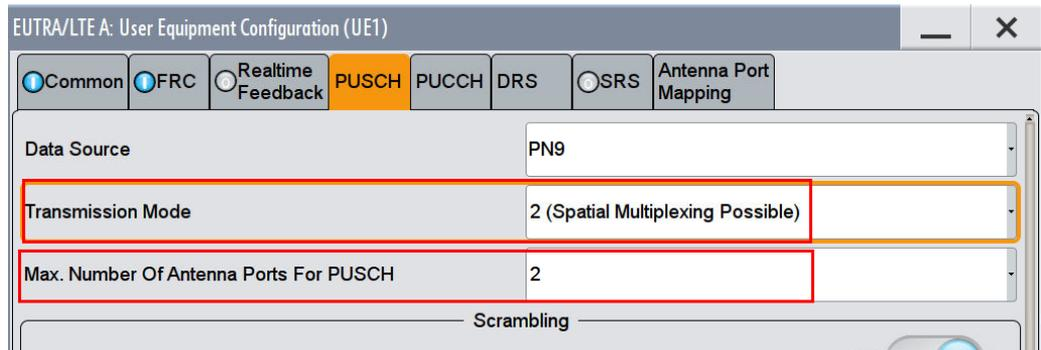
Fig. 3-45: Transmission mode (TM2) and number of antenna ports
