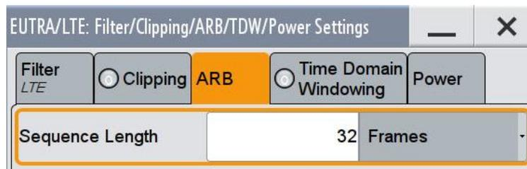
Fig. 3-230: 32 frames to generate the pattern continuously
