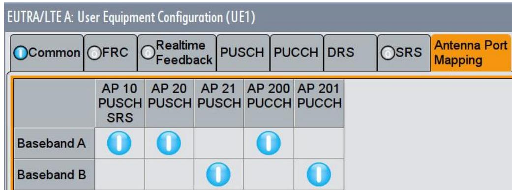
Fig. 3-156: The antenna port mapping. The PUCCH AP200 is generated by BB A, the AP201 by BB B
