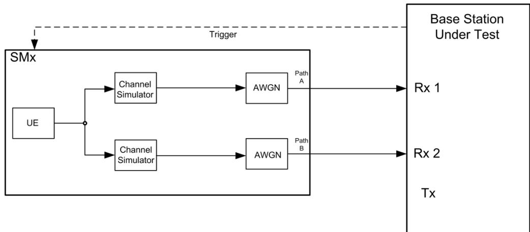
Fig. 3-111: Test setup for PUCCH test 8.3.4 for 2 antennas
