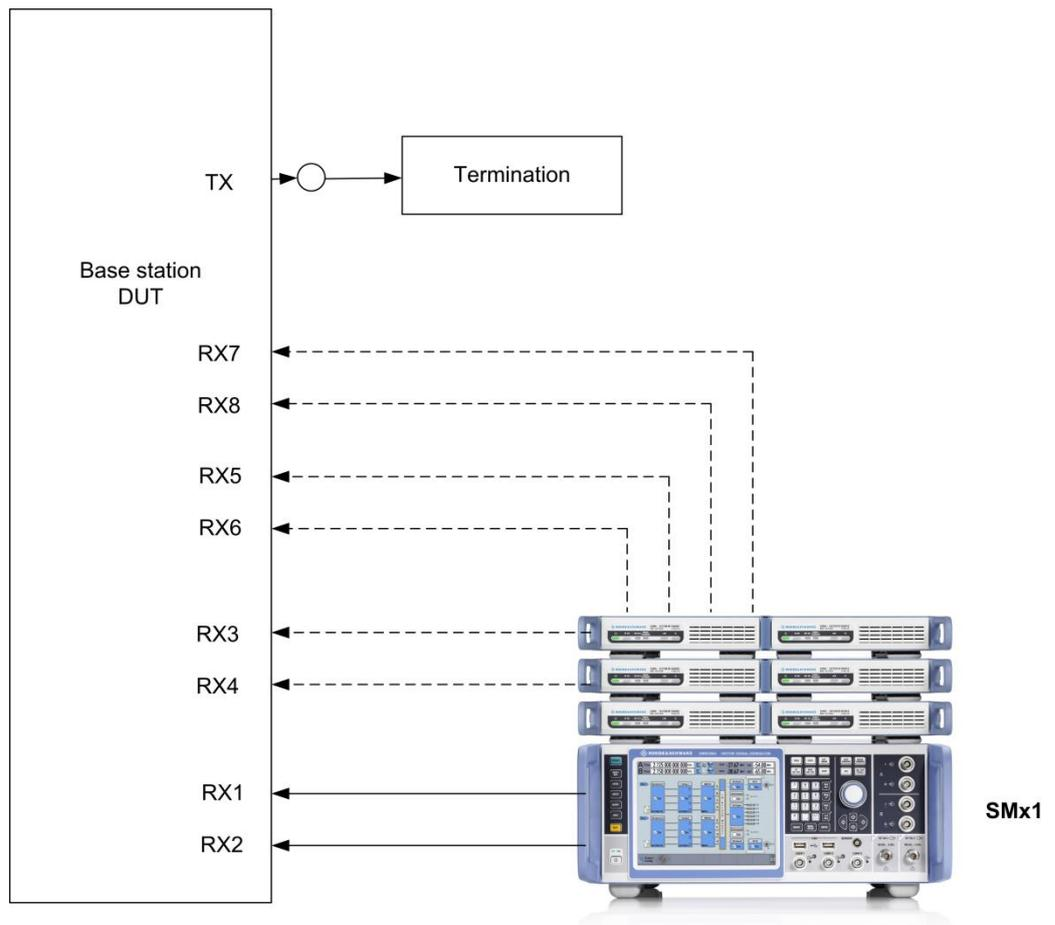
Fig. 2-1: Px Test Setup; To generate signals for four Rx antennas, one SMW plus two SGS are necessary. To generate signals for eight Rx antennas, one SMW plus six SGx are necessary.
