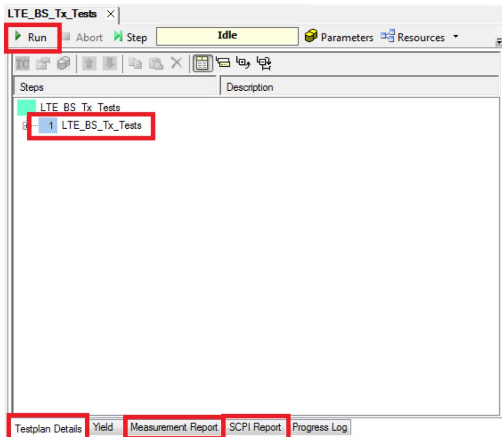
Fig. 4-2: Overview of a test plan in TStrun. The test plan in the example contains only one test (LTE\_BS\_Tx\_Tests). After the test is completed, the bar along the bottom can be used to display the measurement and SCPI reports.
