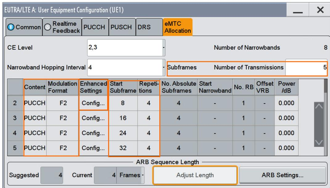
Fig. 3-181: Five transmissions of NPUSCH format 2 to generate the wanted pattern
