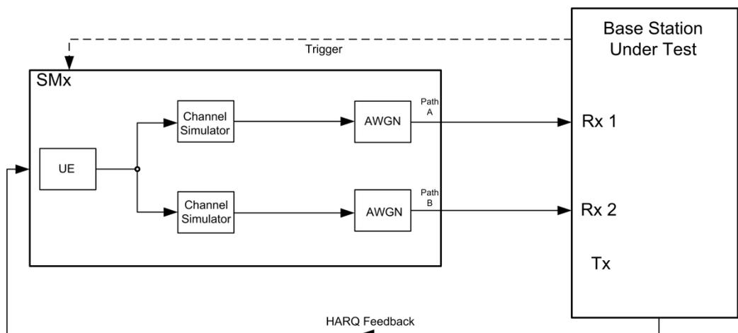
Fig. 3-223: Test Setup for NB-IoT tests 8.5 (the feedback is necessary for 8.5.1 only)
