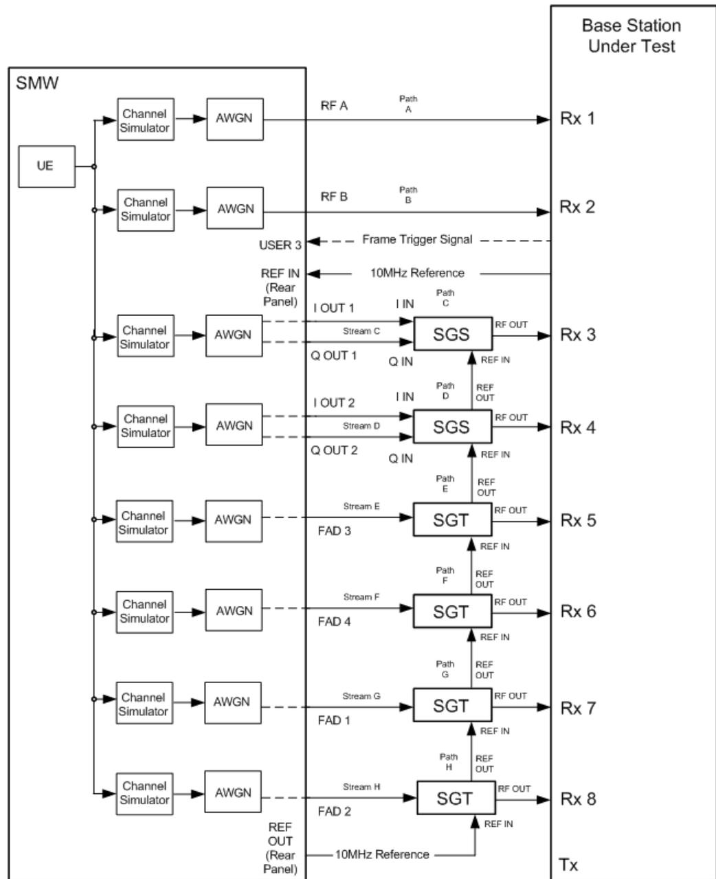
Fig. 3-113: Test setup for PUCCH test 8.3.4 for 8 antennas with one SMW
