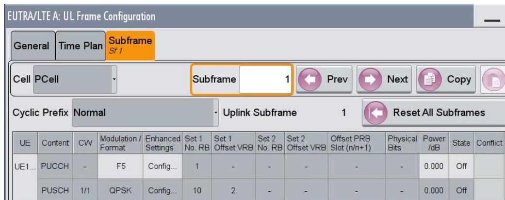
Fig. 3-201: In the second configurable subframe (subframe #1) the PUCCH is not transmitted (state Off)
