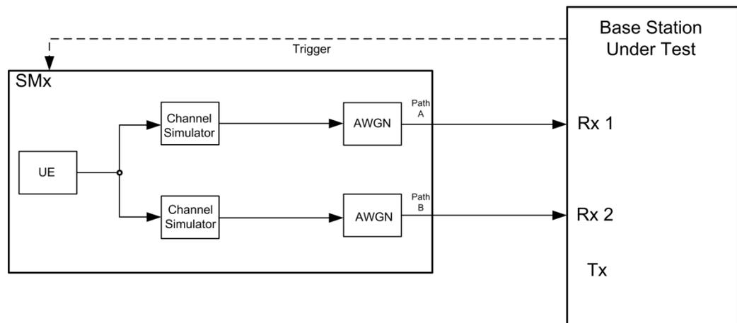
Fig. 3-179: Test setup for PUCCH test 8.3.11
