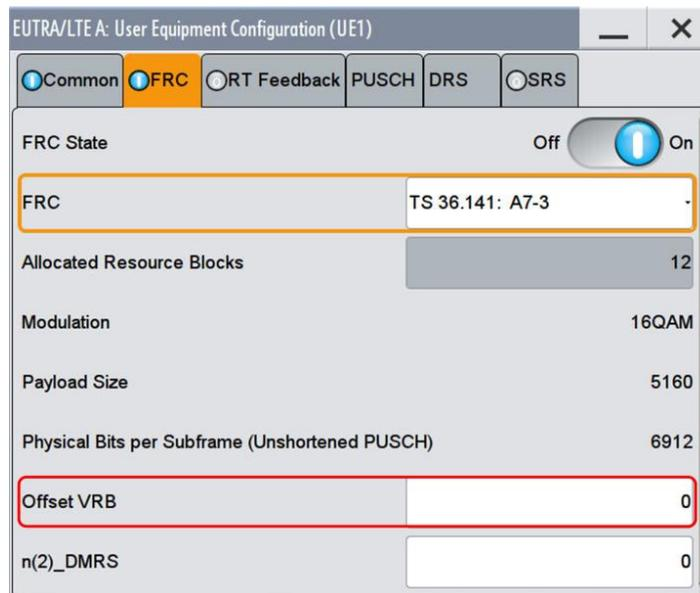
Fig. 3-55: Setting the FRC and Offset VRB (path A)
