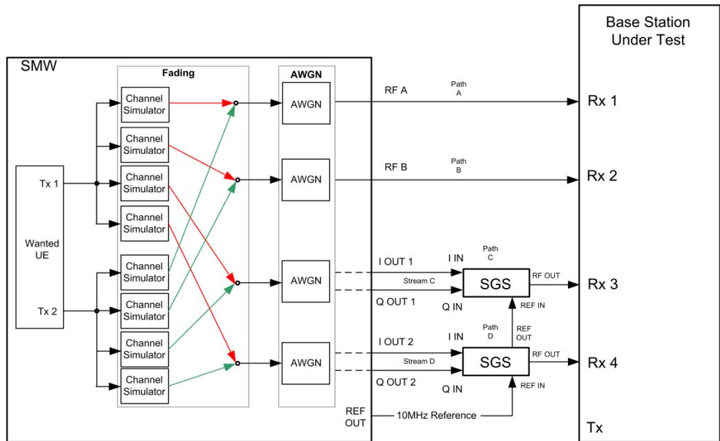
Fig. 3-142: Test setup for PUCCH test 8.3.7 for 4 antennas with one SMW
