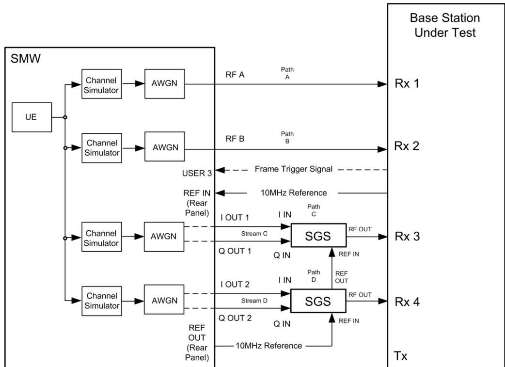
Fig. 3-207: Test Setup for PUCCH Test 8.4.1 for 4 Antennas with one SMW
