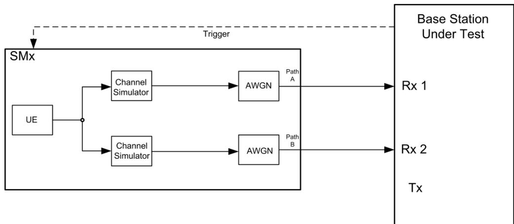
Fig. 3-195: Test setup for PUCCH test 8.3.13
