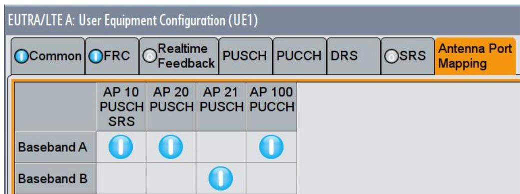
Fig. 3-46: Antenna port mapping for PUSCH 8.2.1A
