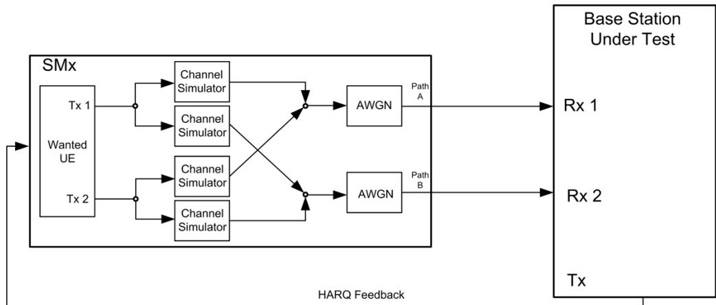
Fig. 3-40: Test setup for PUSCH test 8.2.1A for 2 antennas
