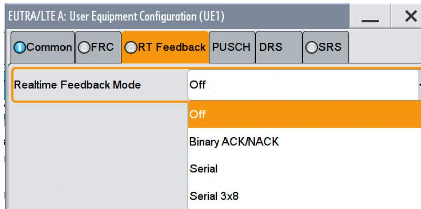
Fig. 3-30: The three supported mode in option SMW-K69
