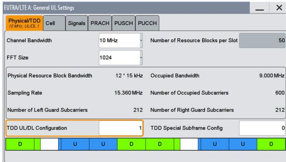
Fig. 3-5: Setting the TDD UL/DL Configuration in duplexing mode TDD (example: 1)
