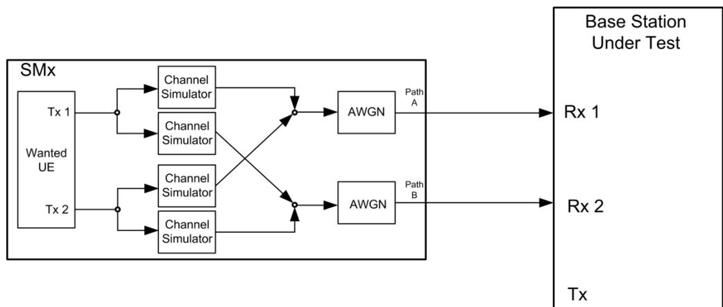
Fig. 3-153: Test setup for PUCCH test 8.3.8
