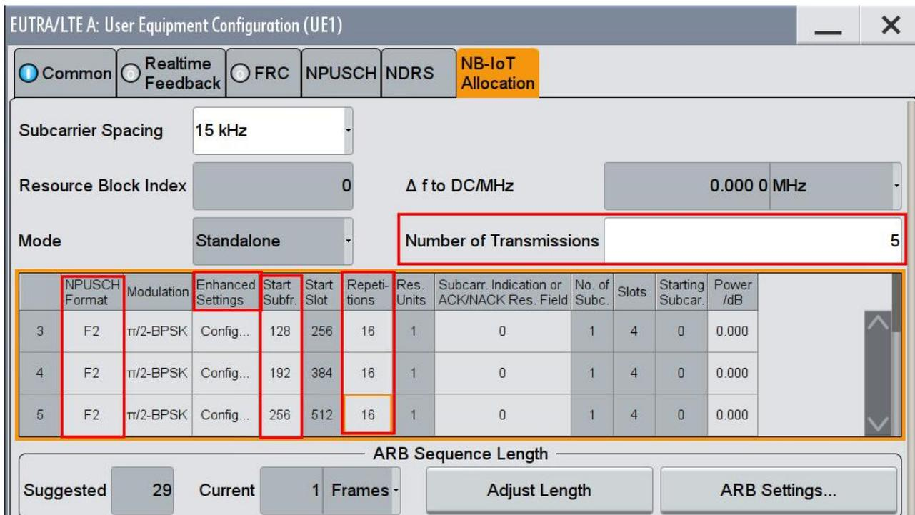
Fig. 3-229: Five transmissions of NPUSCH format 2 to generate the wanted pattern
