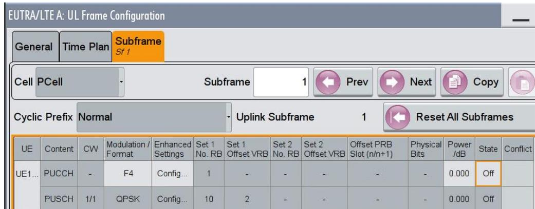
Fig. 3-191: In the second configurable subframe (subframe #1) the PUCCH is not transmitted (state Off)
