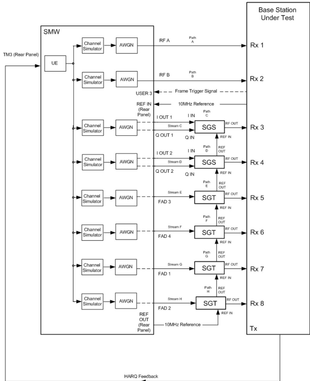
Fig. 3-35: Test setup for PUSCH test 8.2.1 for 8 antennas with one SMW
