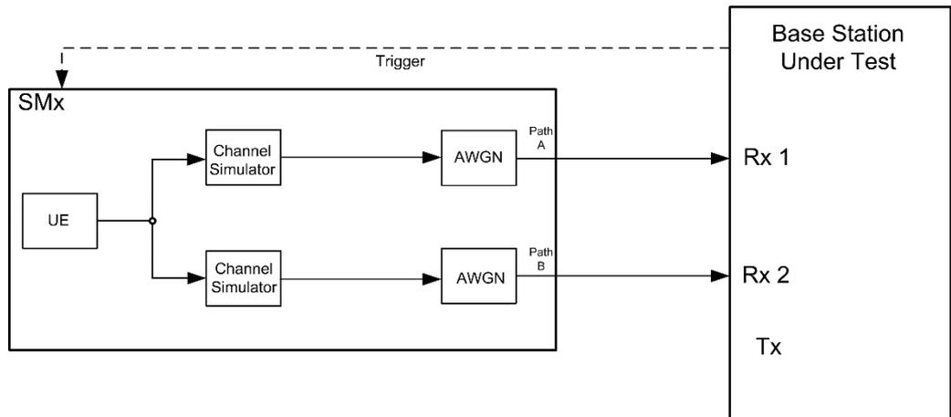
Fig. 3-162: Test setup for PUCCH test 8.3.9 for one Tx antenna
