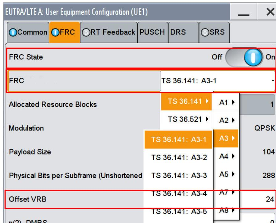
Fig. 3-37: Setting the FRC and the Offset VRB for UE1.
