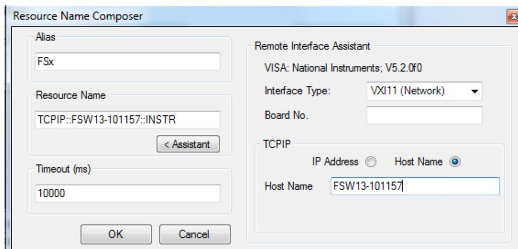
Fig. 4-5: Wizard for entering VISA parameters. Both the IP address and a host name can be entered directly.
