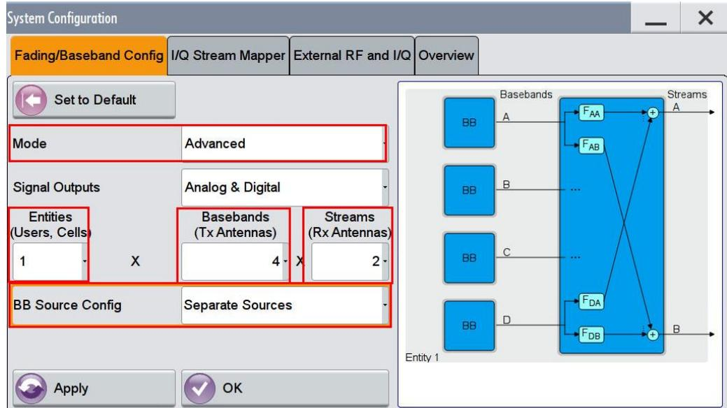
Fig. 3-100: System configuration for PUCCH 8.3.3. A network combining network similar to 4x2 MIMO is used. Baseband A simulates the wanted signal. Baseband B...D simulate the three interferers.
