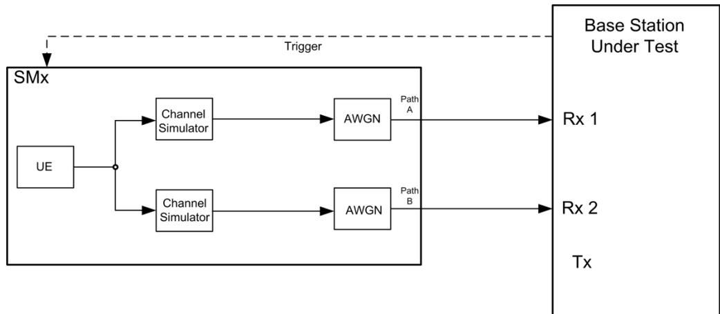
Fig. 3-91: Test setup for PUCCH test 8.3.2
