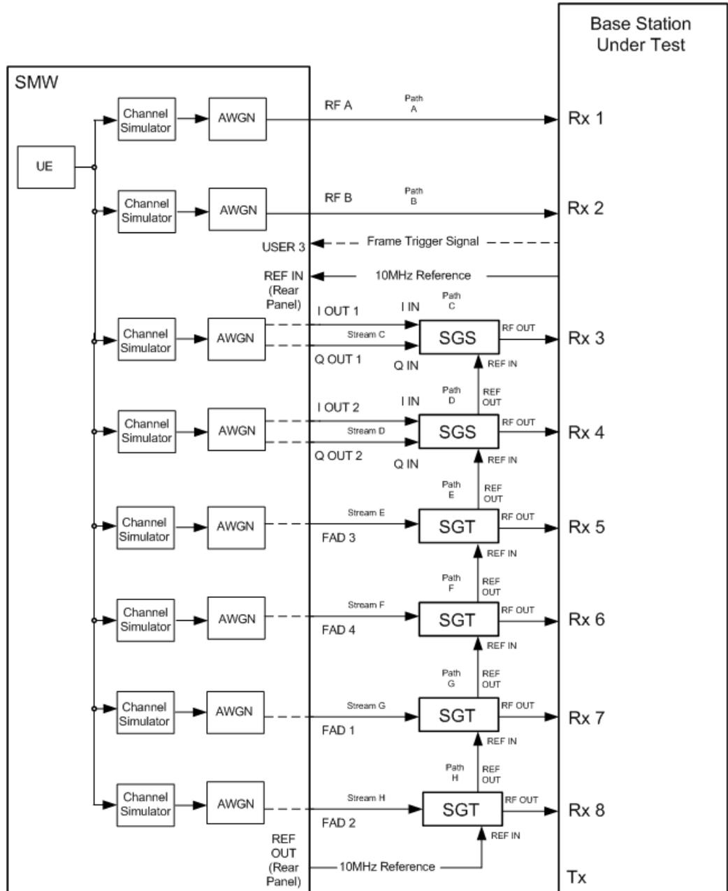
Fig. 3-208: Test Setup for PUCCH Test 8.4.1 for 8 Antennas with one SMW
