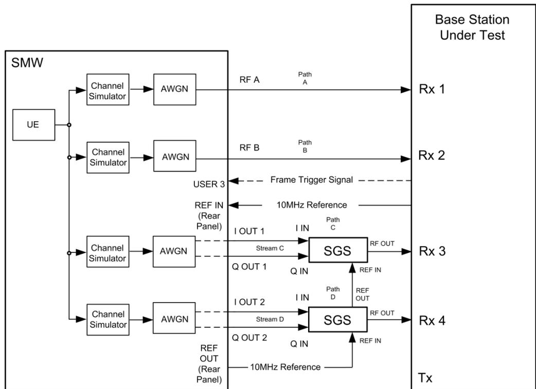
Fig. 3-82: Test setup for PUCCH test 8.3.1 for 4 antennas with one SMW
