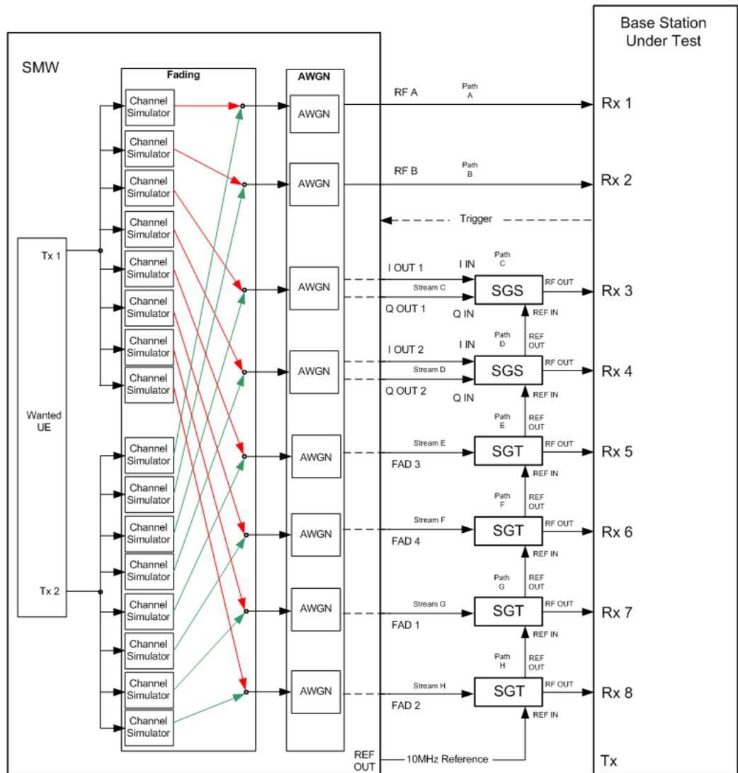
Fig. 3-143: Test setup for PUCCH test 8.3.7 for 8 antennas with one SMW
