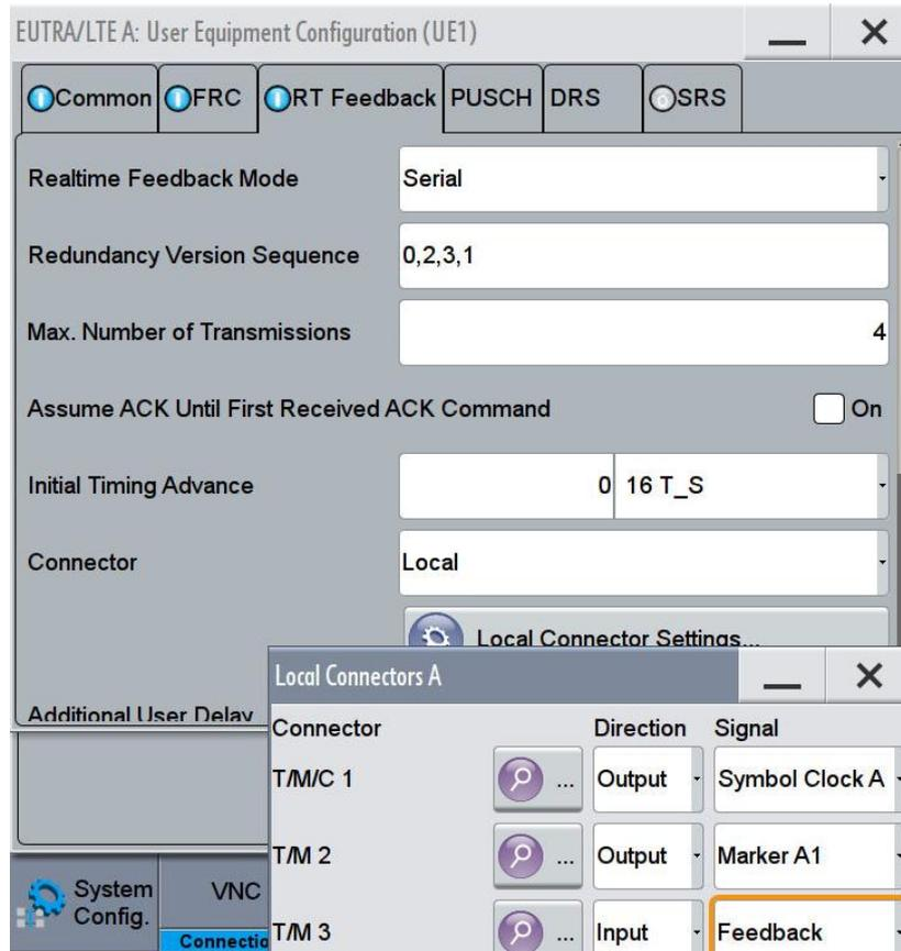
Fig. 3-32: Settings for using a serial feedback line from the BS to SMW. The HARQ-feedback line from the BS is connected with Local Connector T/M3 at the SMW rear panel.
