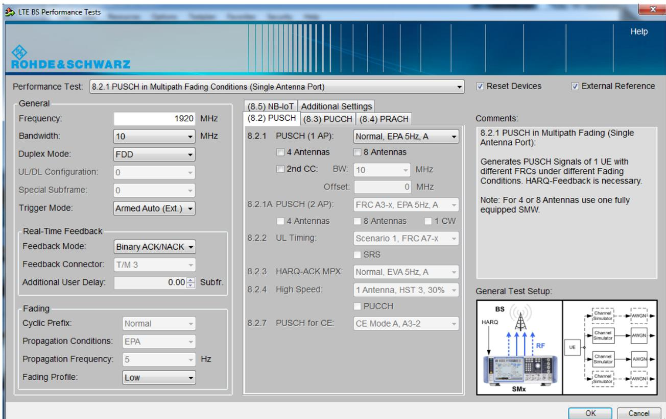
Fig. 3-24: Full overview: setting parameters for the LTE BS Performance tests.
