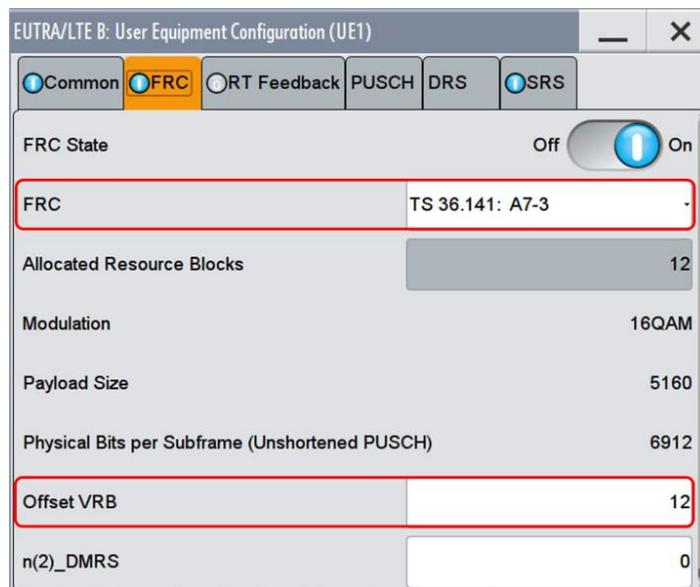
Fig. 3-56: Setting the Offset VRB of path B to ensure that the RBs are allocated consecutively.
