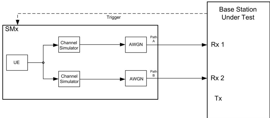
Fig. 3-121: Test setup for PUCCH test 8.3.5 for 2 antennas
