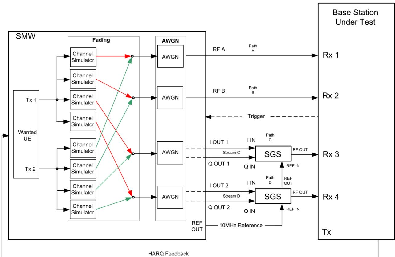
Fig. 3-41: Test setup for PUSCH test 8.2.1A for 4 antennas with one SMW
