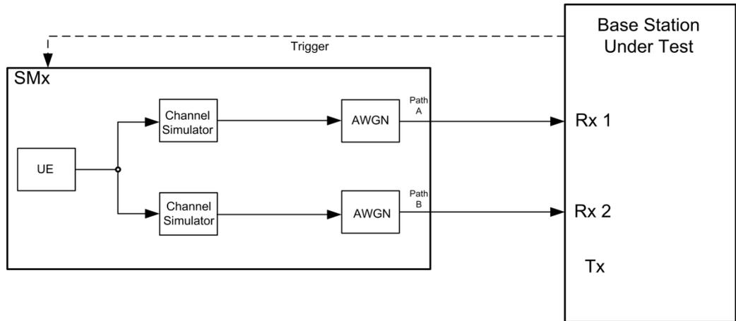
Fig. 3-81: Test setup for PUCCH test 8.3.1 for 2 antennas
