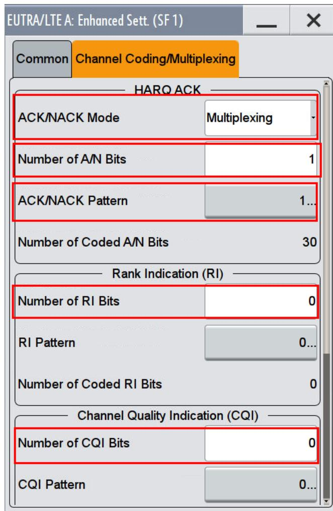
Fig. 3-68: PUSCH multiplexing settings: One ACK bit is multiplexed on the PUSCH
