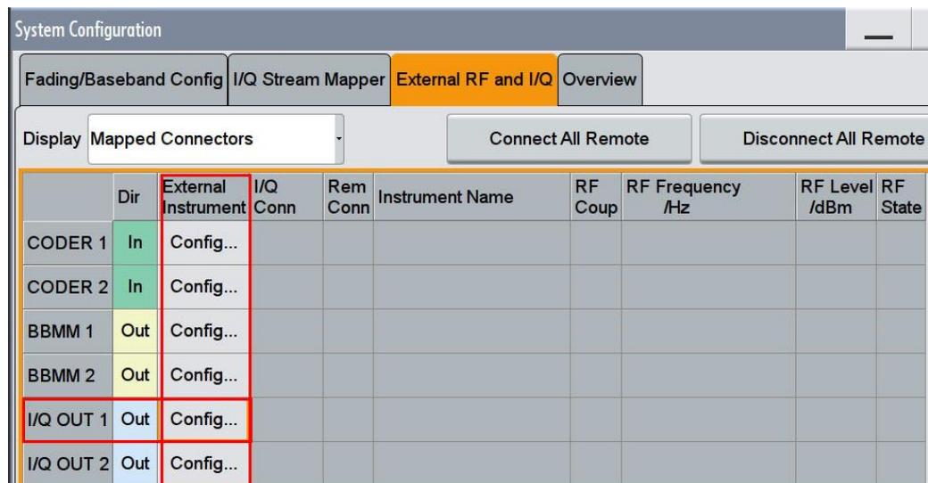
Fig. 3-21: Configuring external instrument at IQ1 Out
