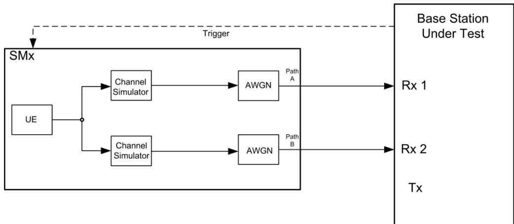
Fig. 3-184: Test setup for PUCCH test 8.3.10
