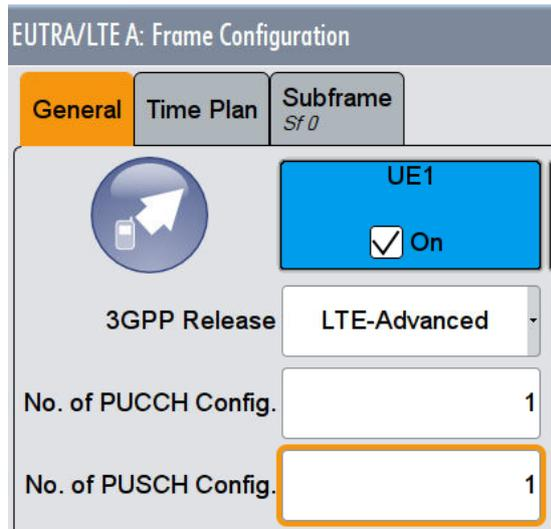
Fig. 3-43: Set one configurable PUSCH subframe. The SMW copies the setting to the other subframes automatically.
