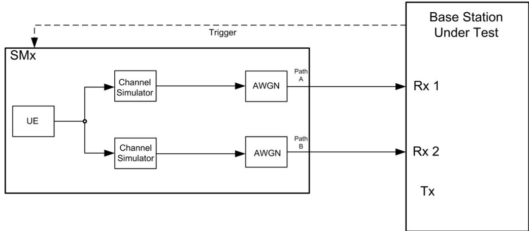
Fig. 3-131: Test setup for PUCCH test 8.3.6 for 2 antennas
