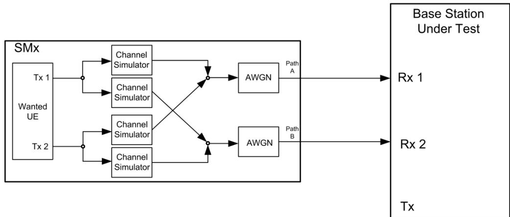
Fig. 3-163: Test setup for PUCCH test 8.3.9 for two Tx antennas
