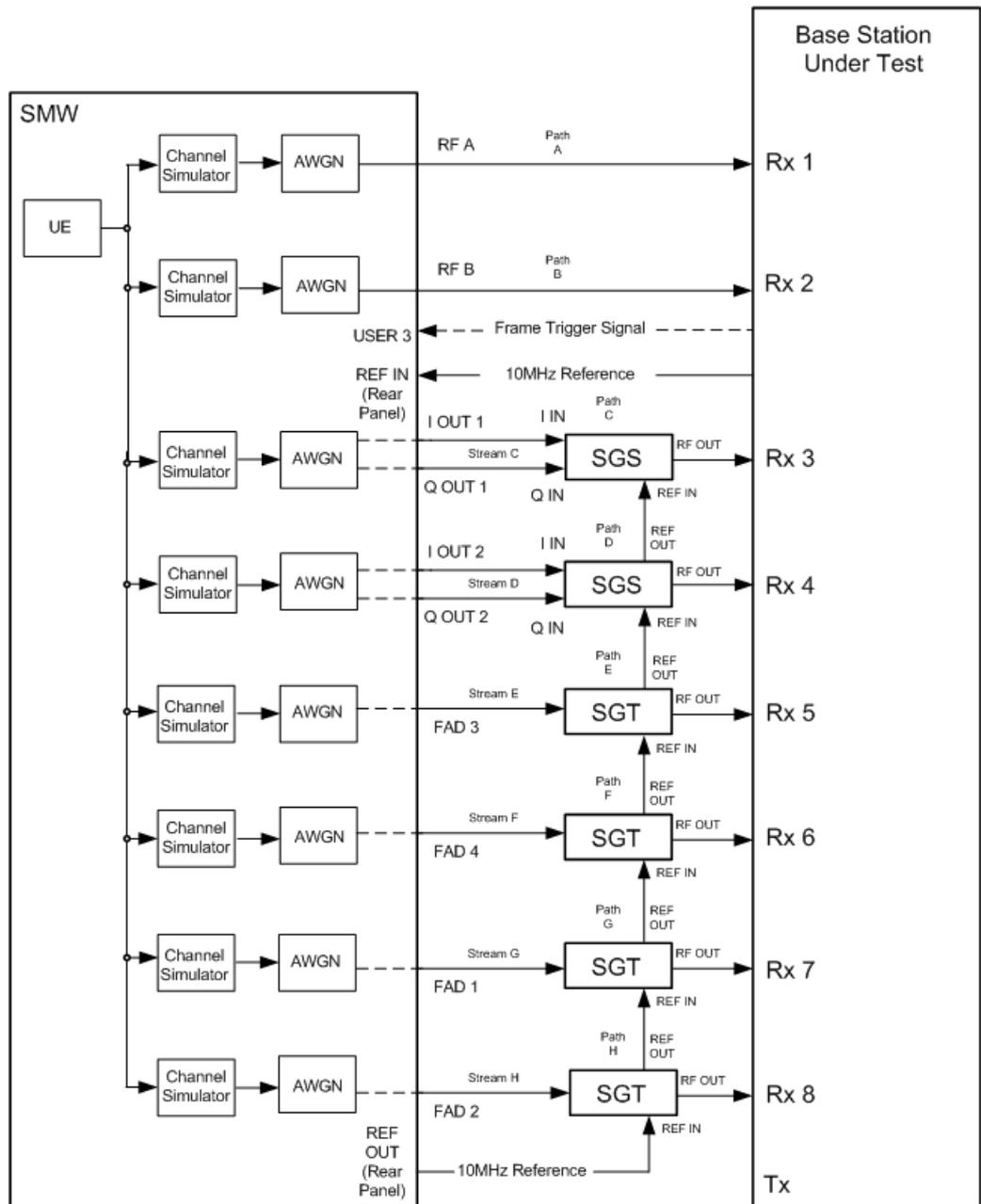
Fig. 3-186: Test setup for PUCCH test 8.3.12 for 8 antennas with one SMW
