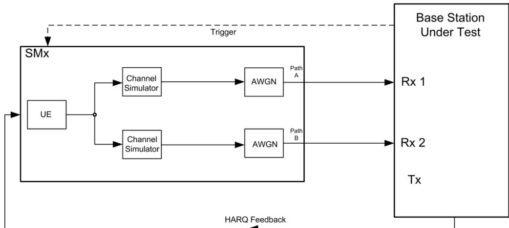
Fig. 3-71: Test setup for PUSCH test 8.2.4 for 2 antennas
