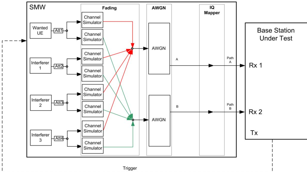
Fig. 3-99: Test setup 8.3.3. with one SMW.
