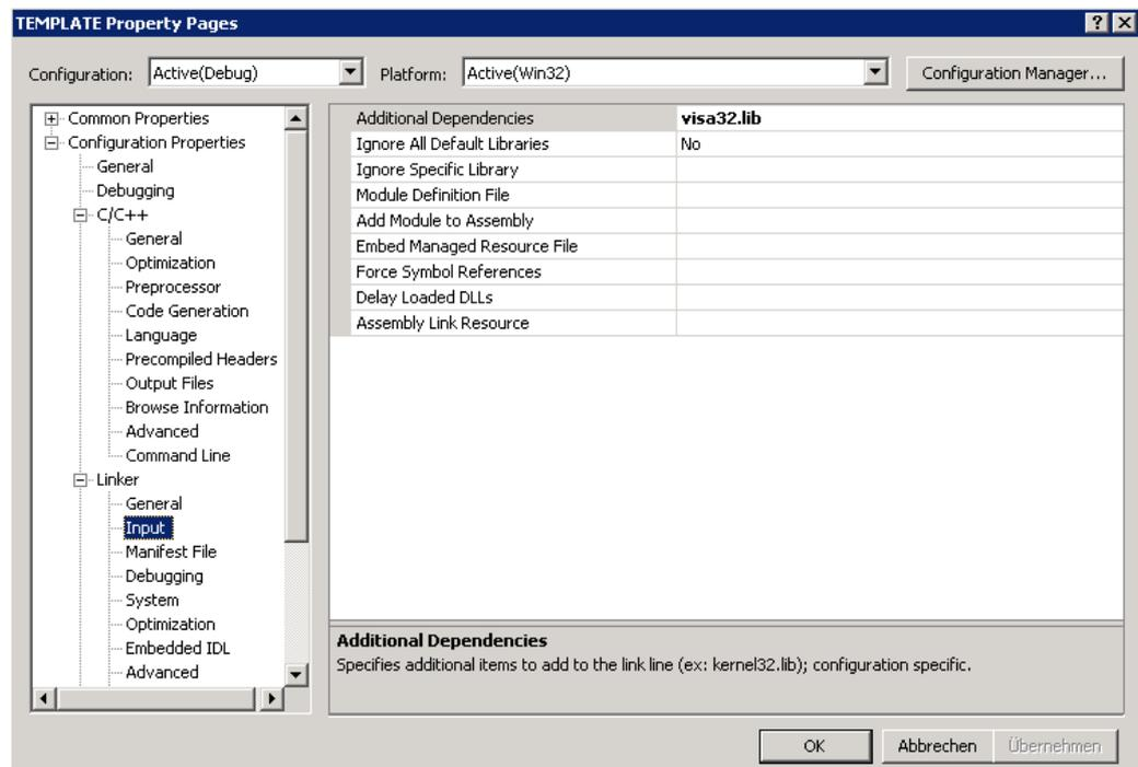
Figure 13: Setting up linker parameter "Additional Dependencies".
