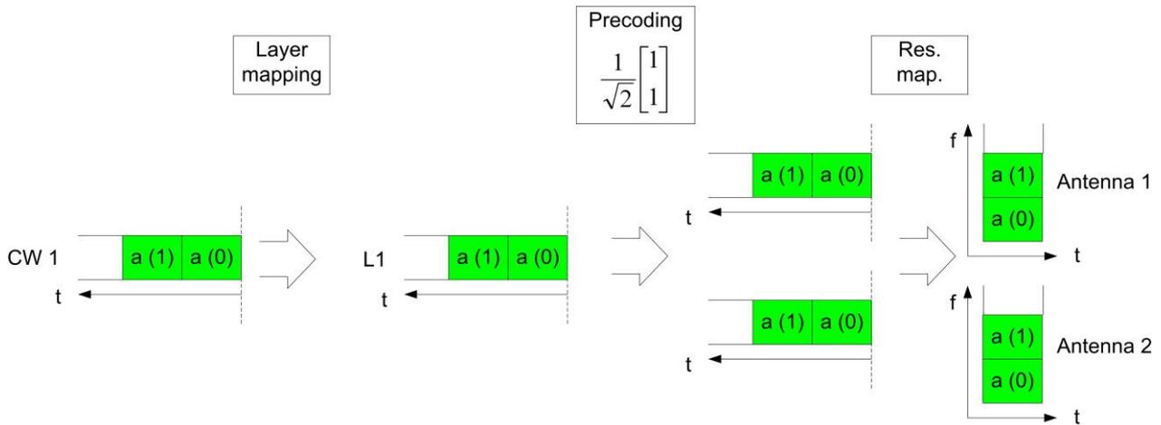
**Figure 3: Pre-coding one CW, one layer, index 0**
