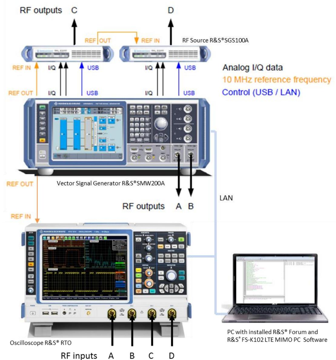
Figure 51: Setup with SMW, SGS and RTO for 4x4 MIMO demonstration
