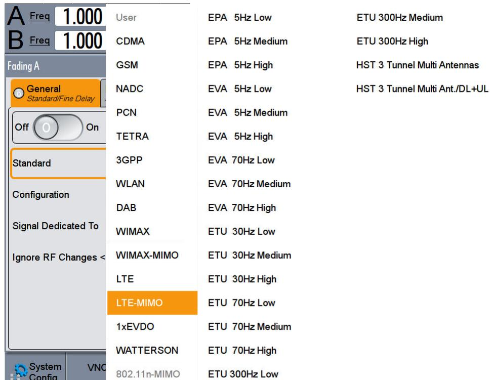
Figure 44: List of predefined fading scenarios for LTE-MIMO
