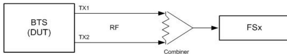
Figure 30: Test setup Time Alignment Error
