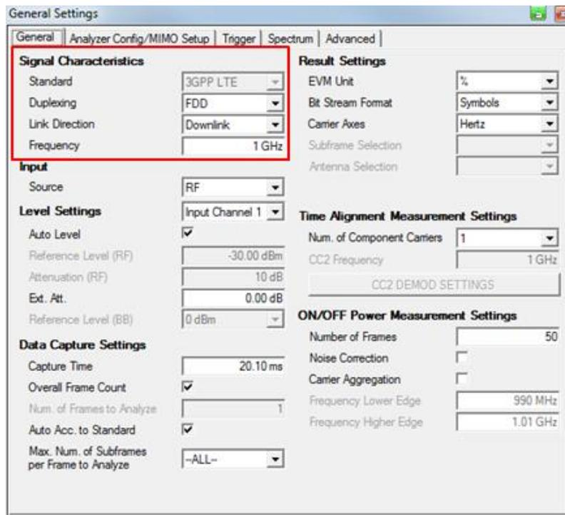
Figure 10: General Settings - Signal characteristics
