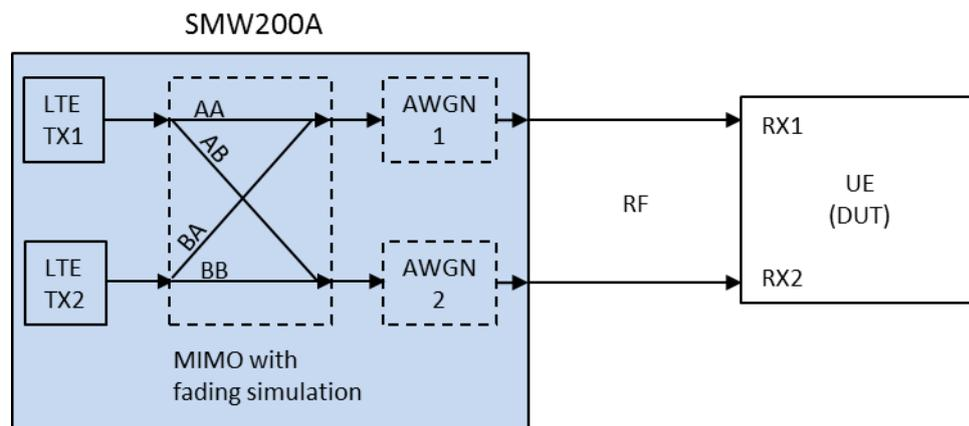
Figure 31: UE receiver test
