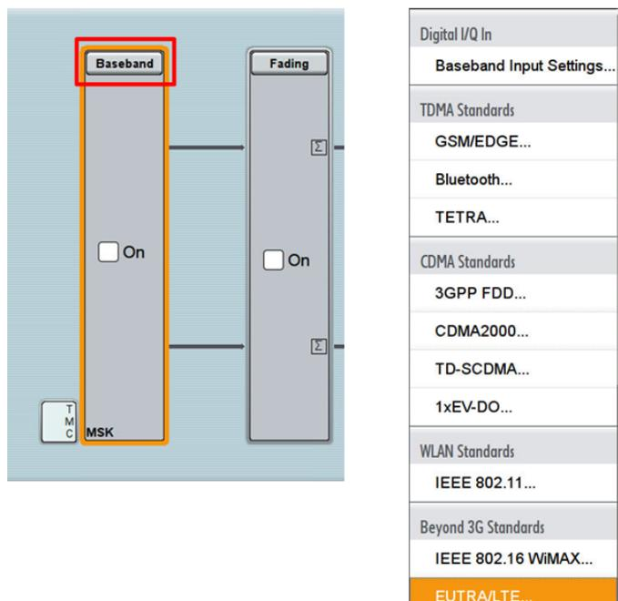
**Figure 33: Baseband A generates the first, baseband B the second transmit (Tx) signal. The internal real-time fading simulators simulate the four fading channels.**
