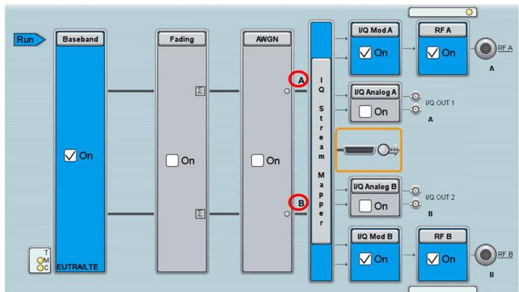
Figure 42: Block diagram on the SMW with stream A (TX1) and stream B (TX2)
