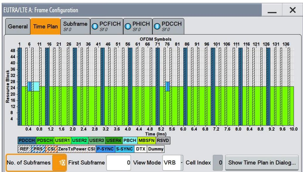
Figure 40: Time plan, example (all sub frames)
