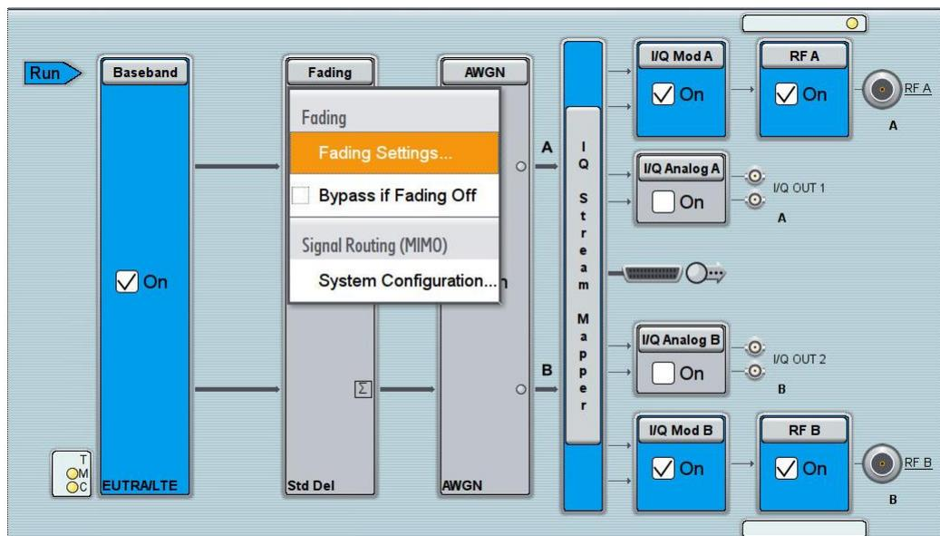
Figure 43: SMW Fading setting selection
