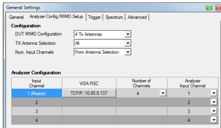
**Figure 55: configuration of the FSK-K102 LTE MIMO PC Software by using the 4 channel Oscilloscope RTO.**
