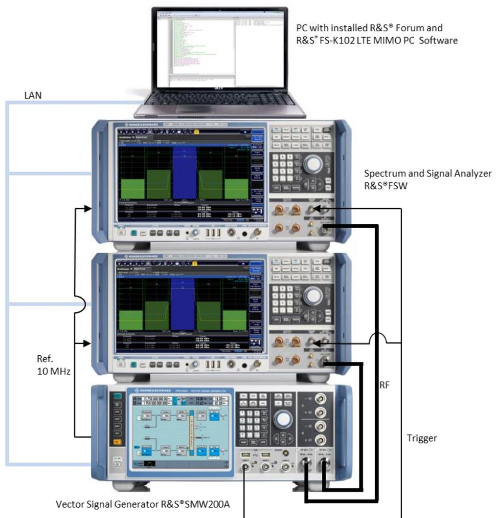
**Figure 50: Setup with SMW and two FSW for demonstration**
