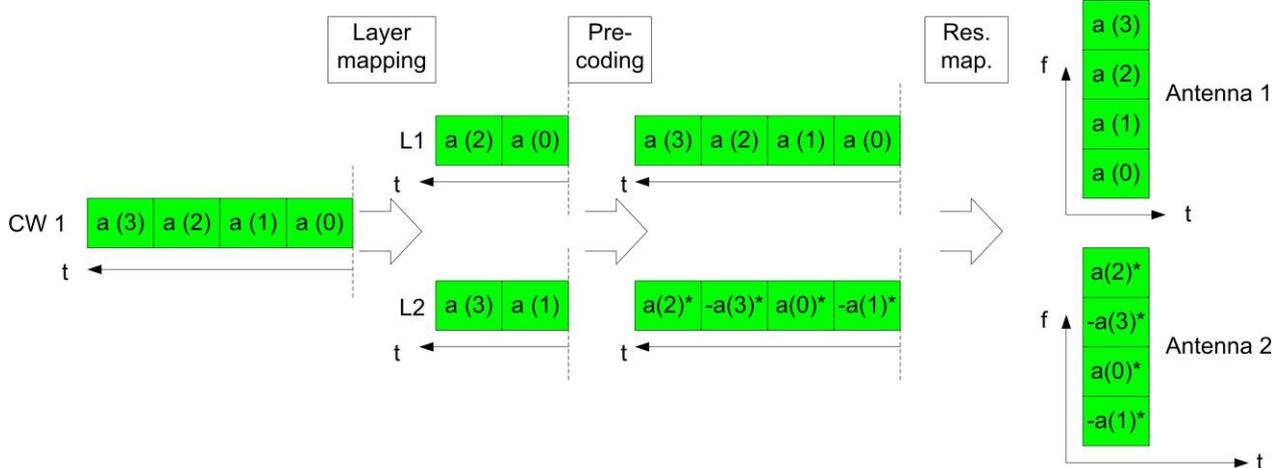
Figure 7: TX diversity with one CW, two layers
