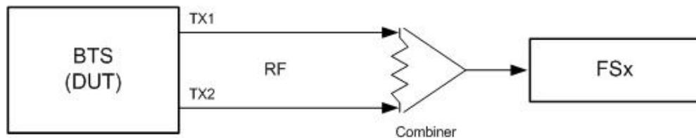
Figure 24: Test setup for time alignment measurements
