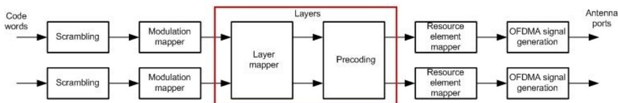
**Figure 1: Downlink physical structure**
