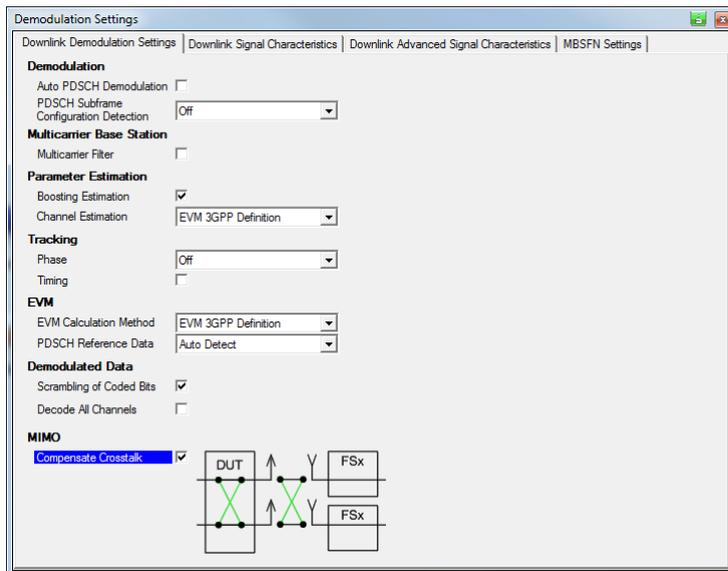
Figure 25: Enabling the Compensate Crosstalk feature
