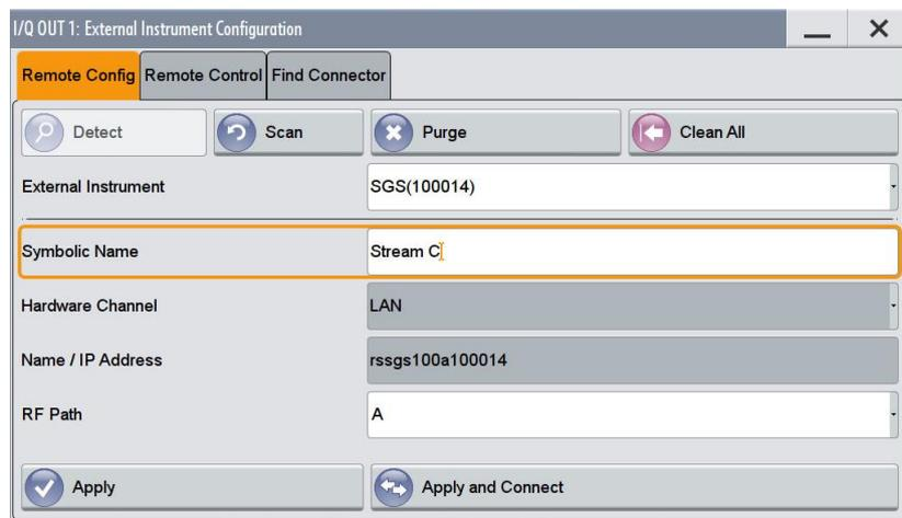
**Figure 53: Configuration of the external RF source R&S® SGS**
