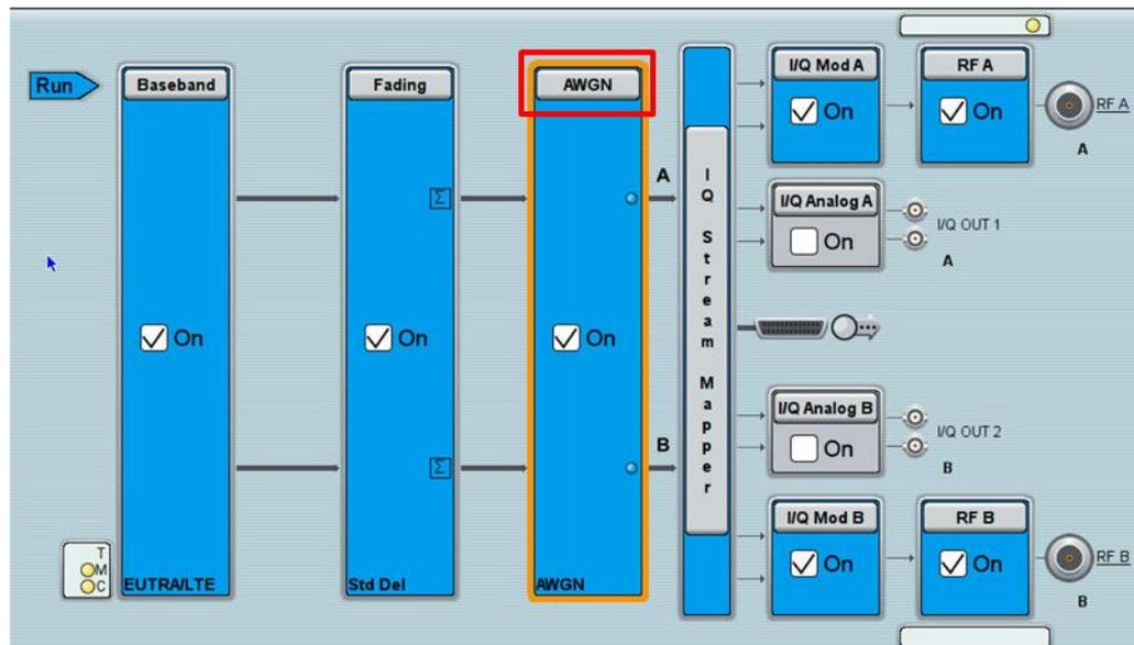
Figure 49: Adding white Gaussian noise
