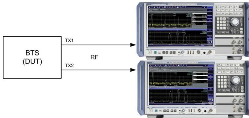
**Figure 8: General test setup for base station tests. For two transmit antennas up to two Analysers are required.**
