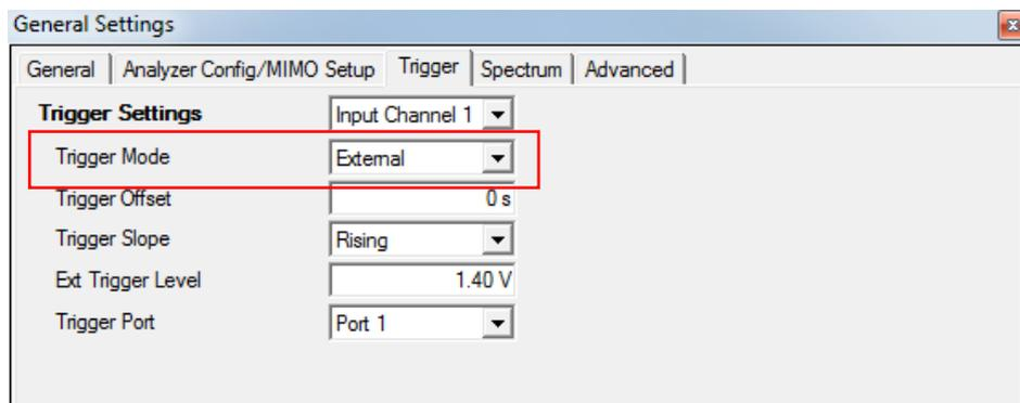
Figure 11: Trigger Settings: An external trigger is necessary to sample on more analyzers at the same time
