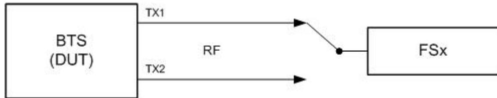
Figure 27: BTS transmitter test with one FSx
