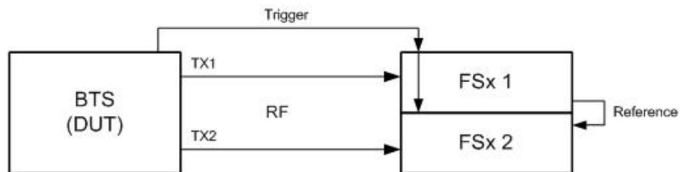
Figure 28: BTS transmitter test with two FSx units
