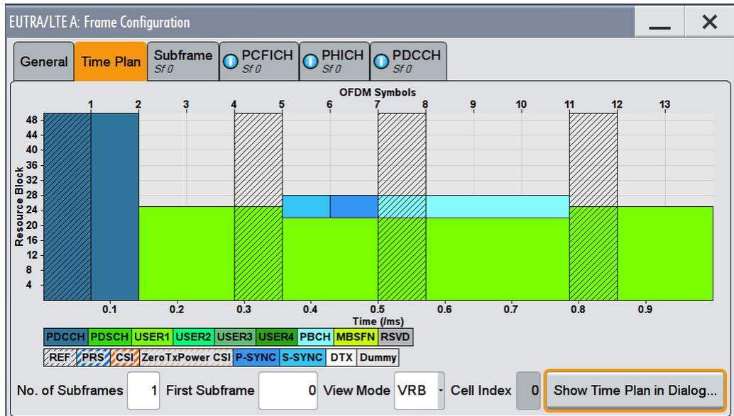
Figure 39: Time plan, example (one subframe)
