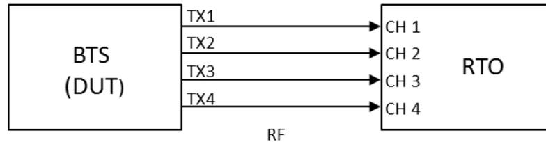
Figure 29: 4x4 MIMO BTS transmitter test with one RTO
