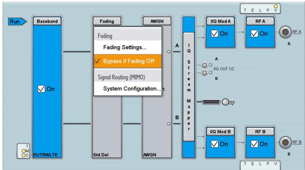
Figure 41: Bypass the fading simulator if it is not needed
