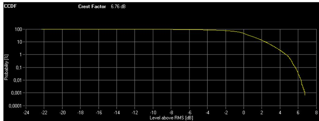
The PAPR depends on the filter used as well as on the modulation format, in contrast to the downlink, where OFDM(A) is used as transmission scheme.
