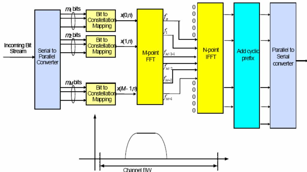
The major difference between the downlink and uplink transmission scheme is that each subcarrier in the uplink carries information about each transmitted modulation symbol ((b) in Figure 5), whereas in downlink each subcarrier only carries information related to one specific modulation symbol ((a) in Figure 5). The peak-to-average power-ratio is minimized and thus the uplink interference.
