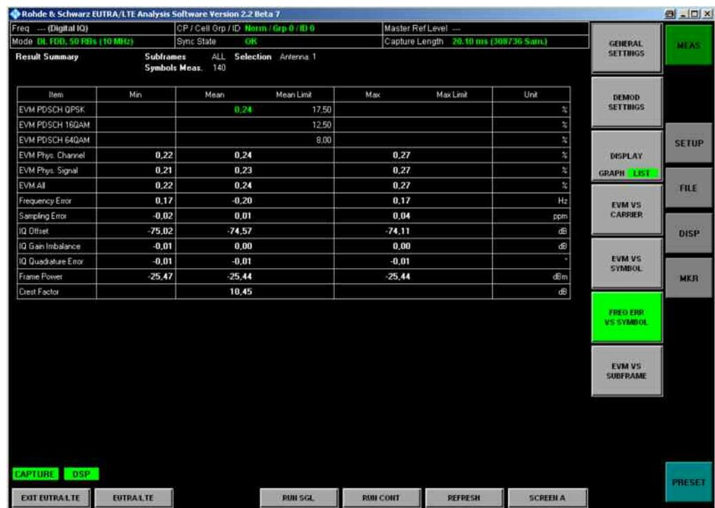
The last parameter listed in the table is the crest factor, also known as peak-to-average power ratio (PAPR). The maximum PAPR for LTE is approximately 12 dB, the same as it is for WiMAX, a competing technology for broadband wireless.
