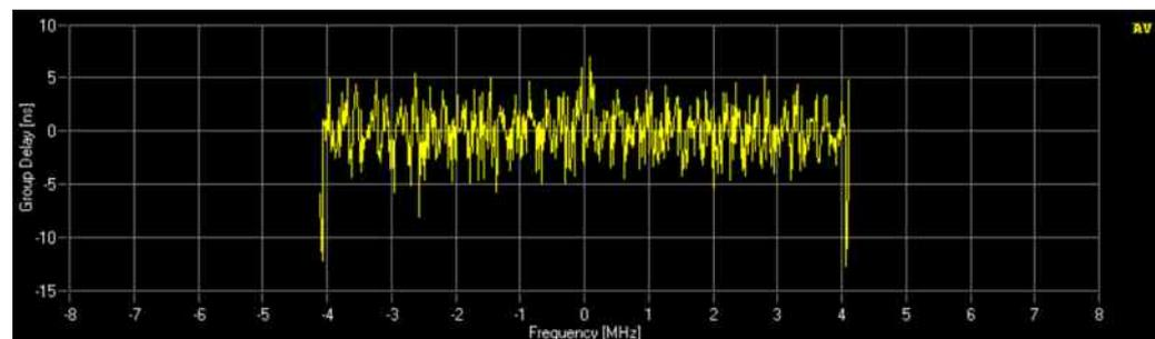
The group delay varies, depending on the filter used. The filter optimized for EVM will decrease the group delay, whereas the ACP-optimized filter will increase the group delay.
