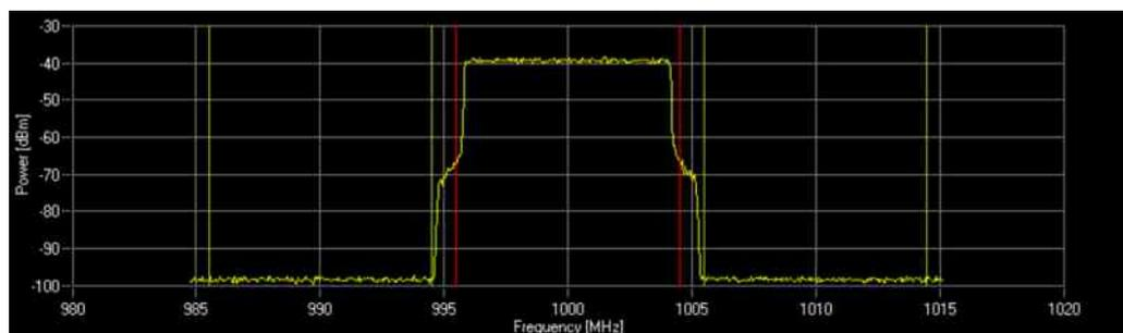
As show in Figure 22 compared to Figure 23 the signal is falling off more smoothly, which is resulting in much better EVM performance. The strong filtering applied to the signal by using the ACP filter (Figure 23) will decrease modulation quality, but improves the ACP and minimizes therefore the impact to other channels or signals.
