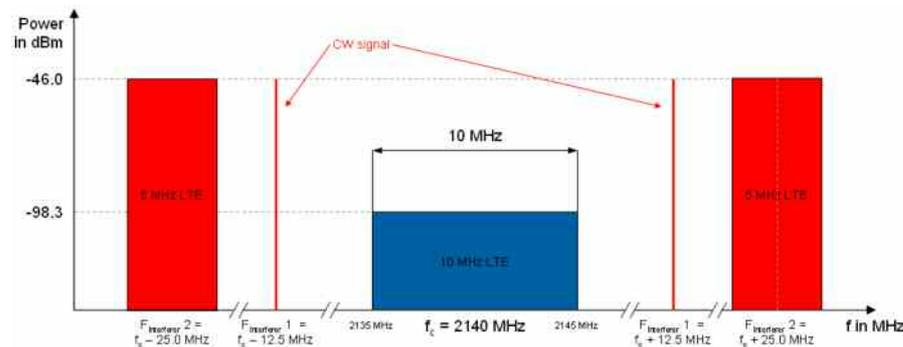
$$F_{\text{interferer 1}} = f_c - 12.5 \text{ MHz} = 2127.5 \text{ MHz} = f_1$$
