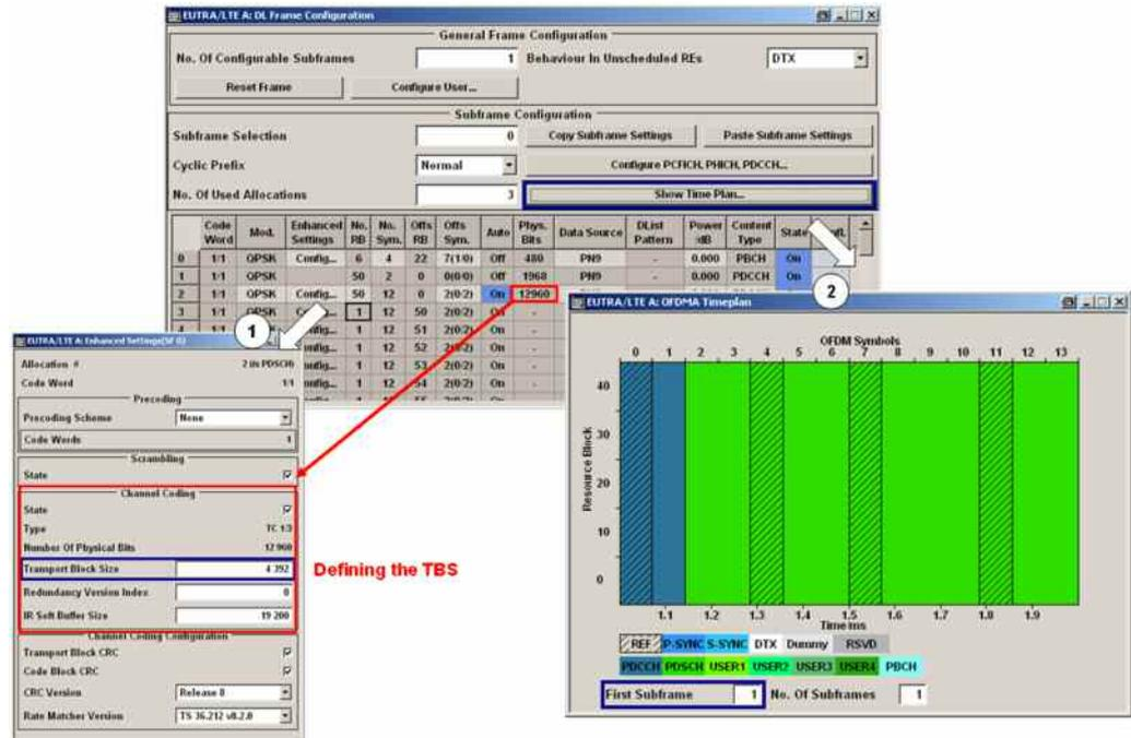
Since the TBS is equal for every subframe, the setting is applied automatically to each subframe by just configuring one frame as described above. This is the reason, why the number of configurable subframes is selected as 1 (see Figure 40). In the case, that a different TBS needs to be set for the individual subframes, the number of configurable subframes needs to be increased. Each subframes needs then to be configured individually.
