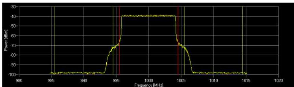
The filter optimized for ACP uses a cut-off frequency shift of 0.34.
