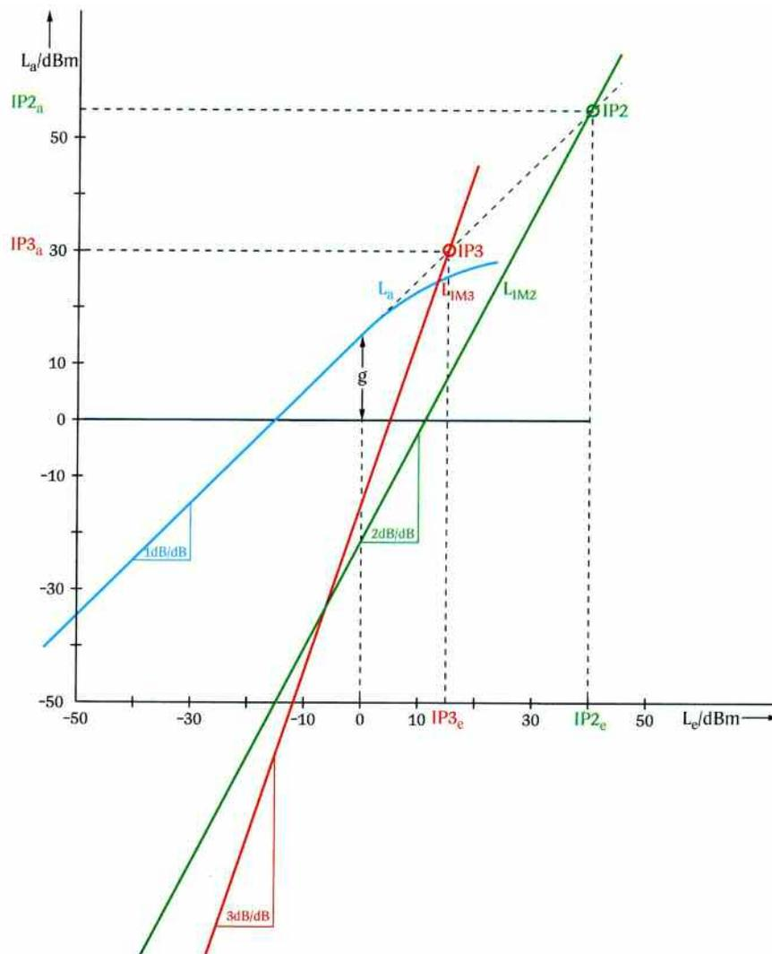
**3<sup>rd</sup> order input intercept point (IIP3).** To assess the LTE receiver for resistance from interference from internally generated intermodulation products, the receiver is tested according to 3GPP specification for its average throughput ( $R_{av}$  in kbps) in presence of third-order intermodulation products, by using two signals with equal power level as interferer. The first interferer is a CW signal, the second is another LTE signal, where
