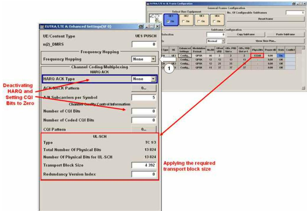
In addition – so that all available bits are used for data transmission – the HARQ ACK(knowledge) Type must be set to 'None' as well as the Number of CQI Bits needed is set to zero.
