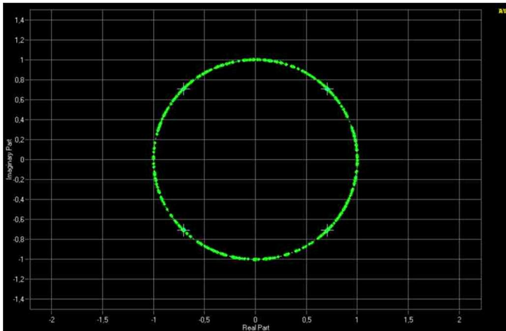
Using the evaluation filter the DRS can be found in SC-FDMA symbols #3 and #10, transmitted over the entire bandwidth, meaning all 552 subcarriers ( $\pm 276$  subcarriers).
