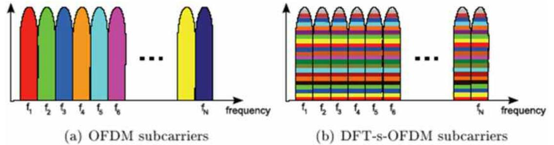
Resources for uplink transmission are also allocated based on resource blocks, using the same number of subcarriers, same time domain parameterization as in the downlink, but for normal and extended cyclic prefix only.
