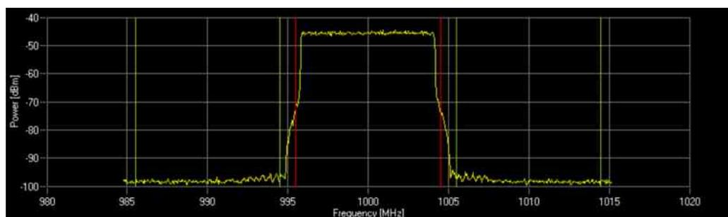
The default values for the EVM-optimized filter are a roll-off factor of  $\alpha = 0.10$  and a cut-off frequency shift of  $-0.20$ .
