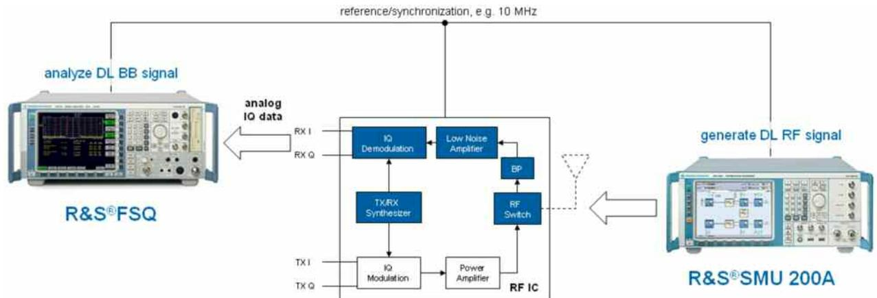
This setup analyzes the complete receiver chain. For measurements on specific components, such as the LNA, the setup changes. The signals are then fed into the LNA, taken from the LNA and analyzed. Accessing specific components depends on the design and is very often customer specific.
