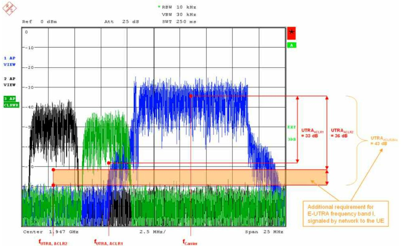
The limits for ACLR measurement are 33 dB respectively 36 dB for  $UTRA_{ACLR1/2}$  as shown in Table 8.
