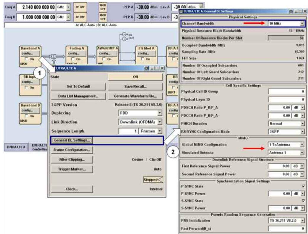
Next step is the frame configuration. By pushing the frame configuration tab the appropriate window will appear. As for uplink, no full resources can be allocated to the UE for user data transmission. Selecting three allocations for the first subframe is necessary for the transmitting of control and broadcast information. As explained in
