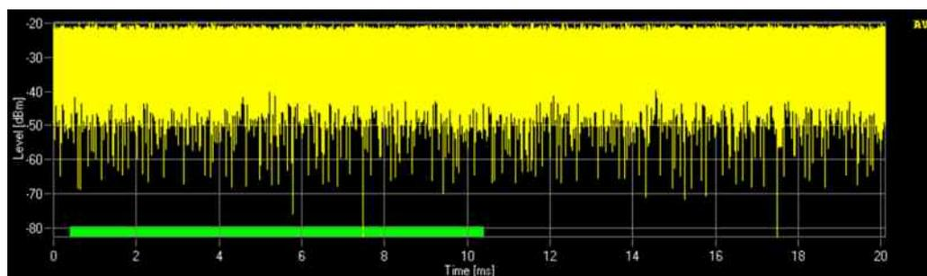
Different signal shapes can be seen, depending on the filter used. The following three example screenshots (Figure 21 to Figure 23) showing the impact of the three different filter types used in the SMU, on the shape of the uplink signal. Figure 21 shows the impact of the filter STANDARD.
