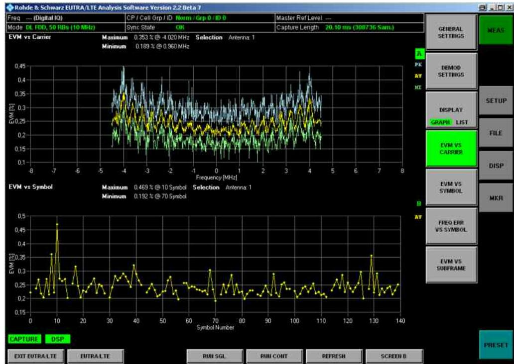
By changing the filter type to ACP the results change completely as shown in Figure 49. The strong filtering acts a like a delay and is impacting the signal quality at the edge of the transmission bandwidth. The EVM is increased so much, that under real conditions the performance is not good enough to use a higher order modulation scheme.
