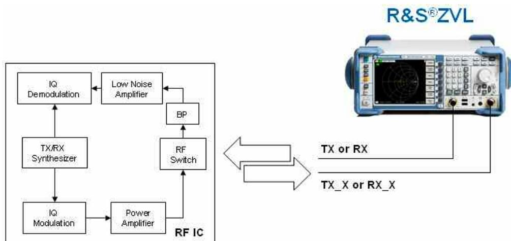
For transmitting as well as receiving it is important that the output and input impedance differ from the expected matching of 50 Ohm. Otherwise a poorer value for noise in the
