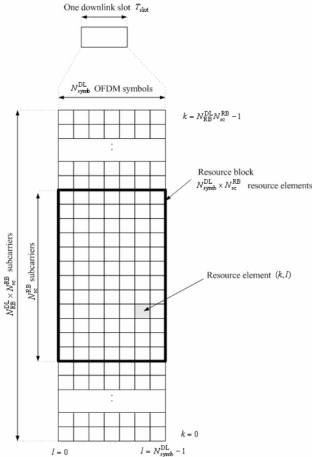
Depending on the assigned bandwidth, the number of subcarriers varies and so the number of resource blocks differs. The 3GPP specification defines the possible bandwidths resulting in the number of resource blocks shown in Table 2.
