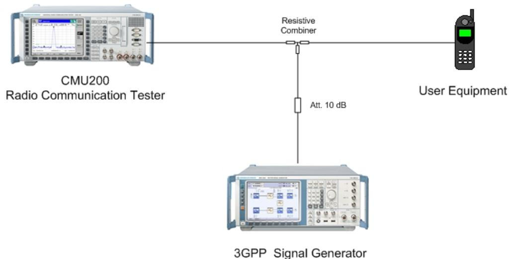
Fig. 14: Test setup for Adjacent Channel Selectivity test
