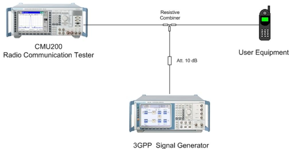
**Fig. 26: Test setup for narrow-band blocking characteristics**
