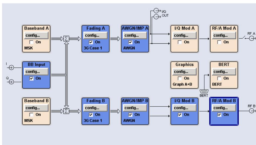
**Fig. 62: Functional signal processing inside the SMU**
