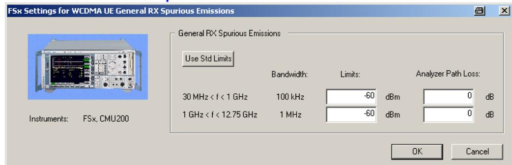
Fig. 36: Module RX General Spurious Emission tests
