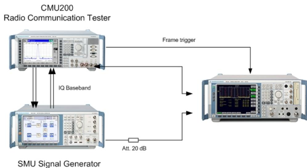
**Fig. 63: Setup path delay**
