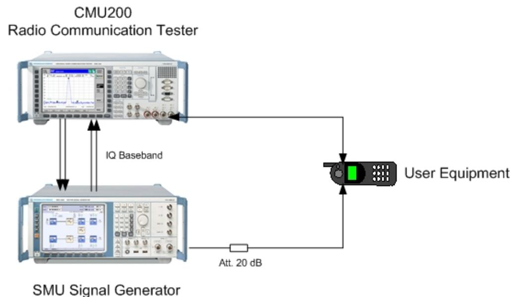
Fig. 55: HSUPA test setup
