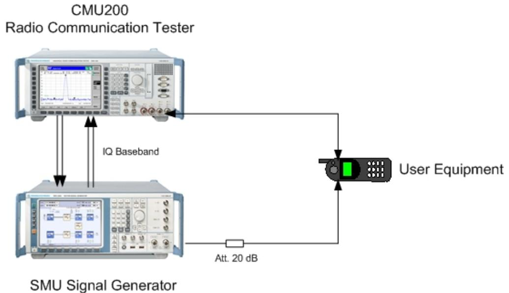
Fig. 47: Instrument test setup for HSDPA tests
