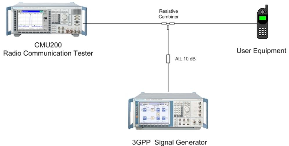
**Fig. 19: Test setup for in-band blocking characteristics**
