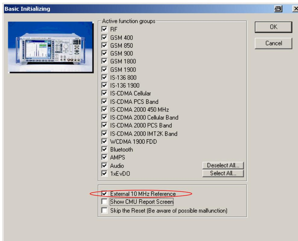
Fig. 4: Activating the external 10 MHz reference
