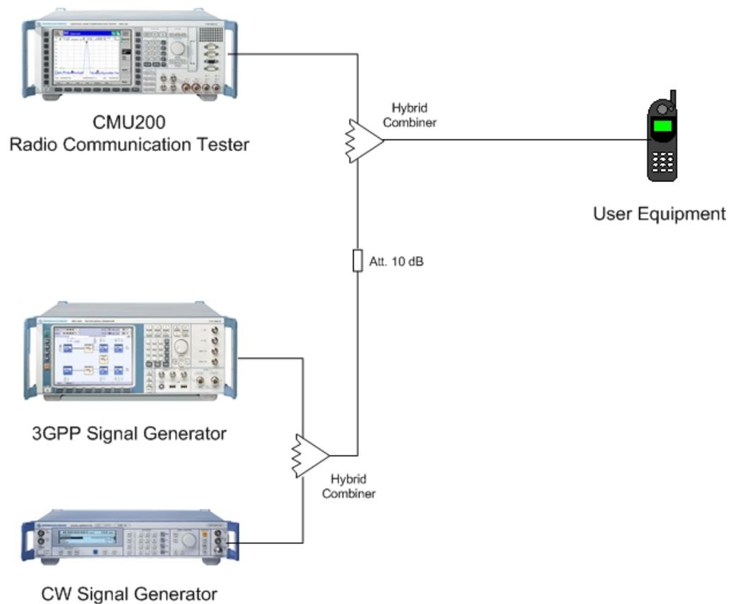
**Fig. 30: Test setup for RX intermodulation test using two separate generators**
