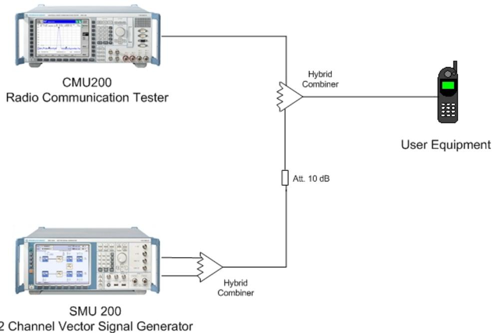
**Fig. 29: Test setup for RX Intermodulation test using a two-channel SMU**
