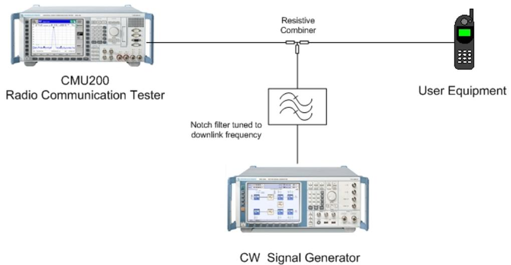
**Fig. 22: Out-of-band blocking below 3 GHz.**
