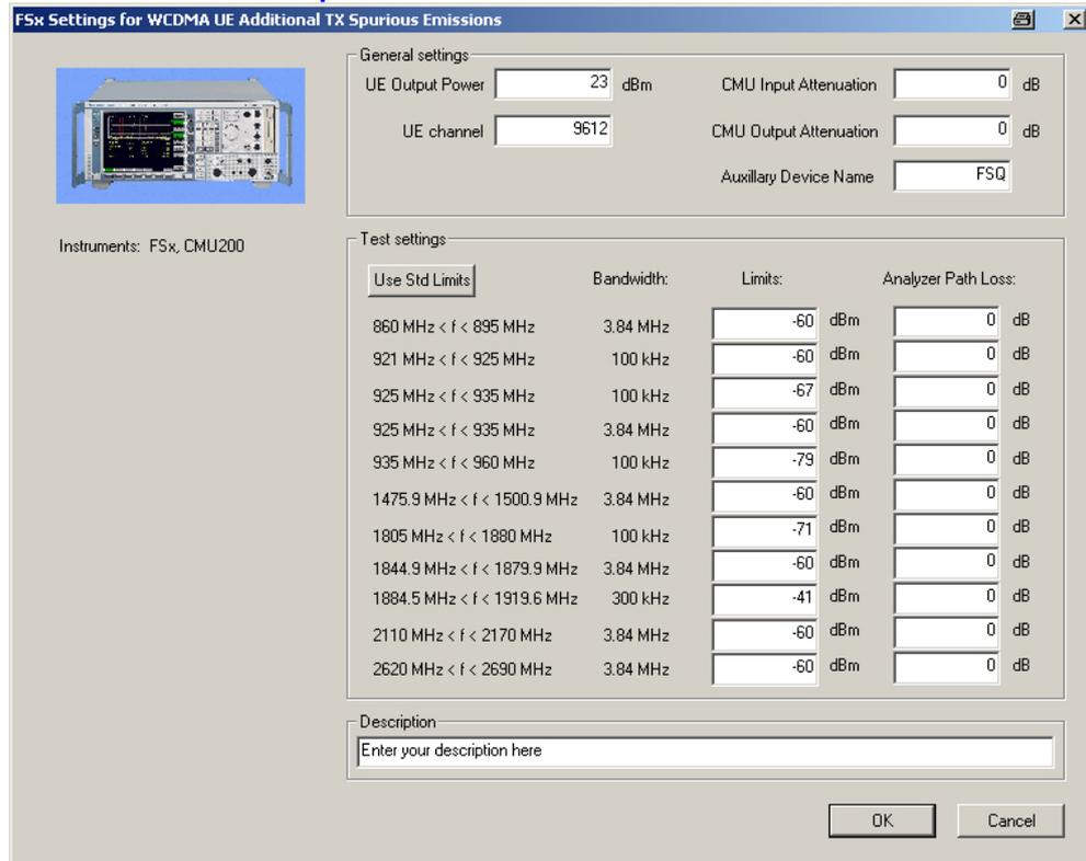
Fig. 7: Setup of the analyzer for Additional Spurious Emissions test
