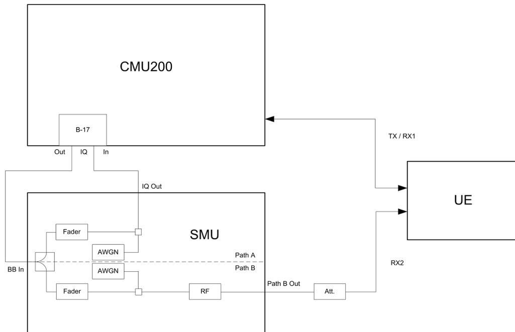
**Fig. 46: Block diagram of test setup for HSDPA tests**
