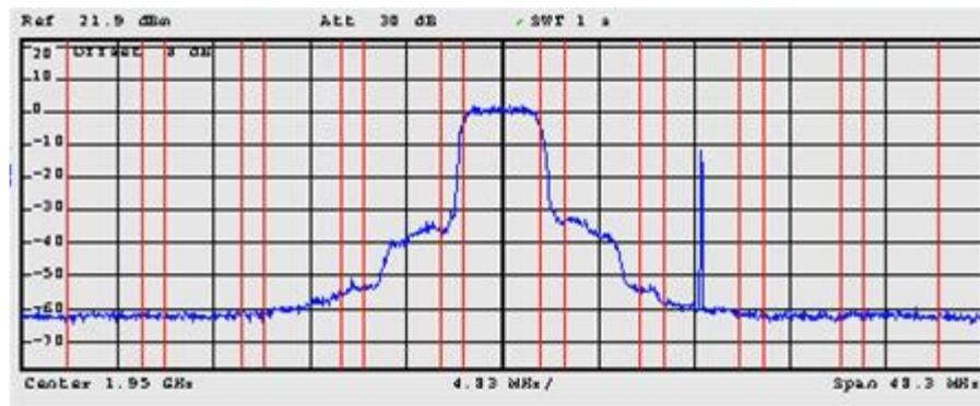
Fig. 12: Transmit Intermodulation test / 10 MHz interferer offset
