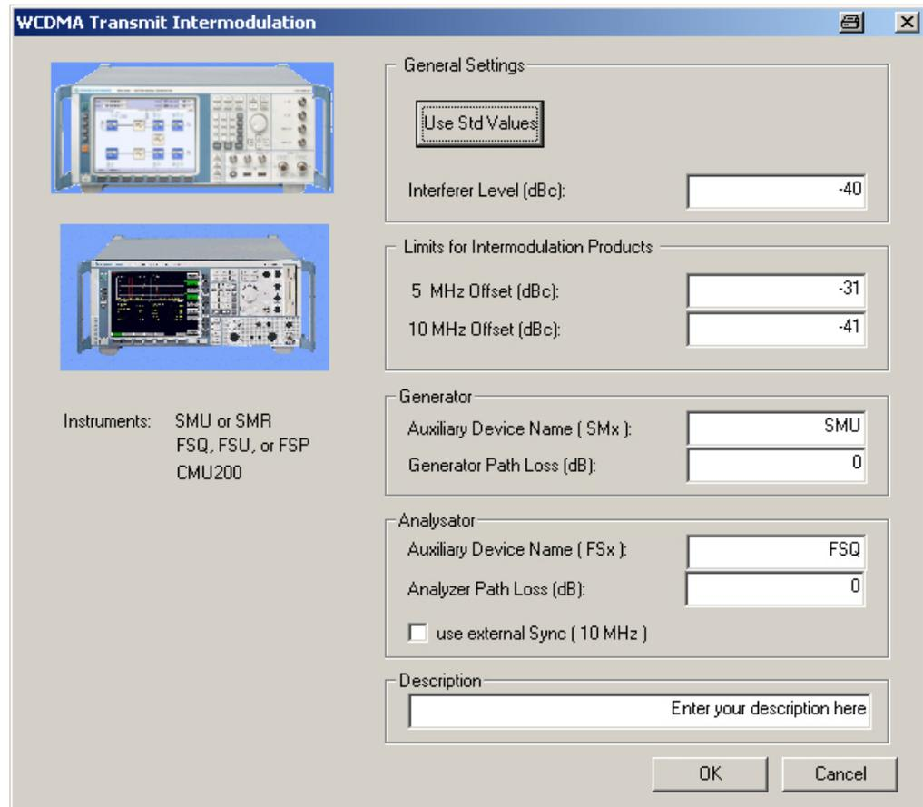
Fig. 11: WCDMA Transmit Intermodulation test module
