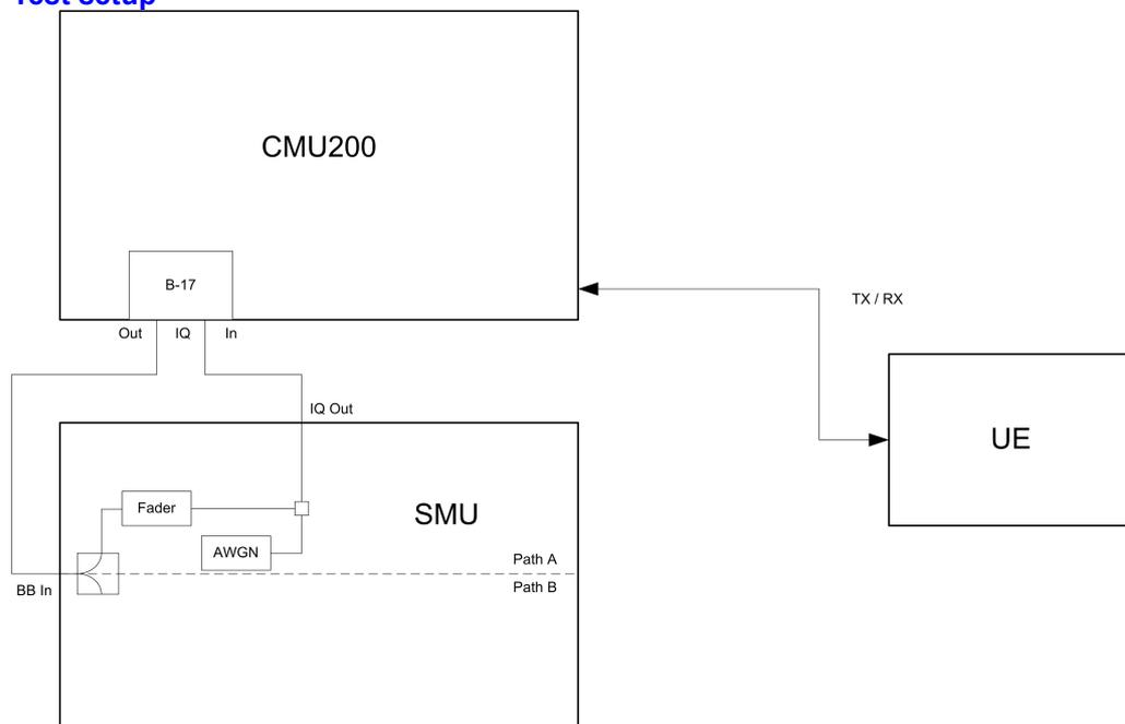
**Fig. 40: Block diagram of test setup for WCDMA fading**
