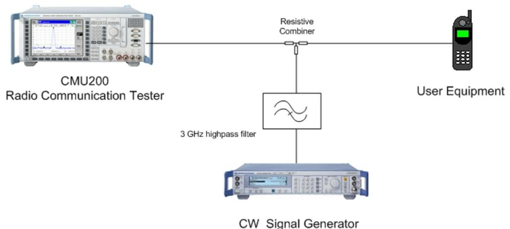
**Fig. 23: Out-of-band blocking above 3 GHz.**
