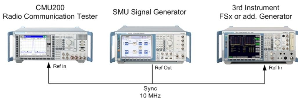
Fig. 3: Synchronization with 10 MHz
