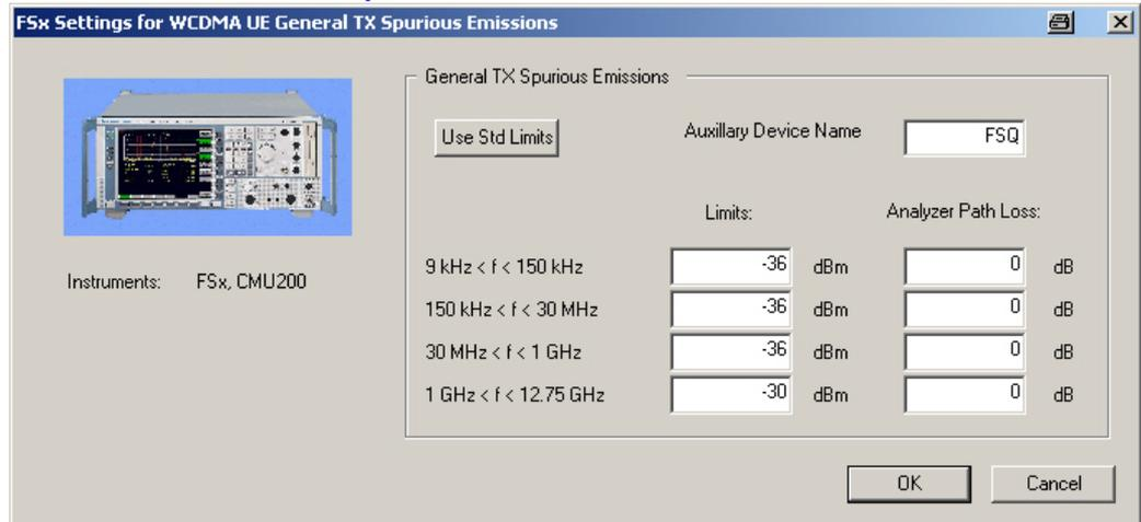
Fig. 6: Setup of the analyzer for General Spurious Emissions test
