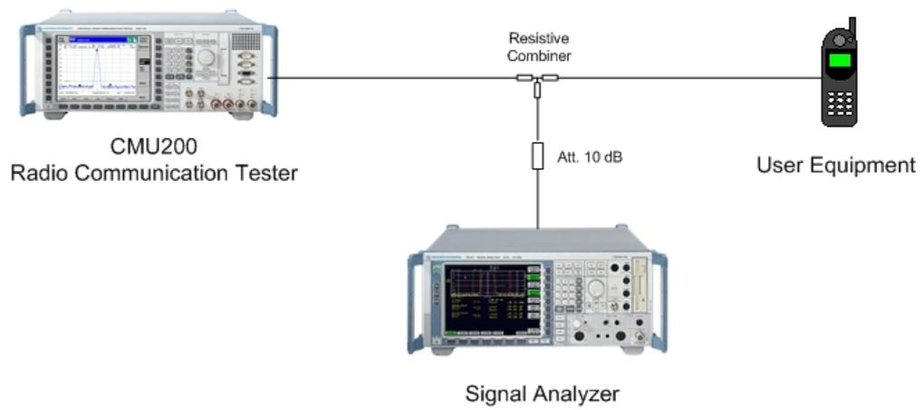
Fig. 35: Test setup for RX Spurious Emission test
