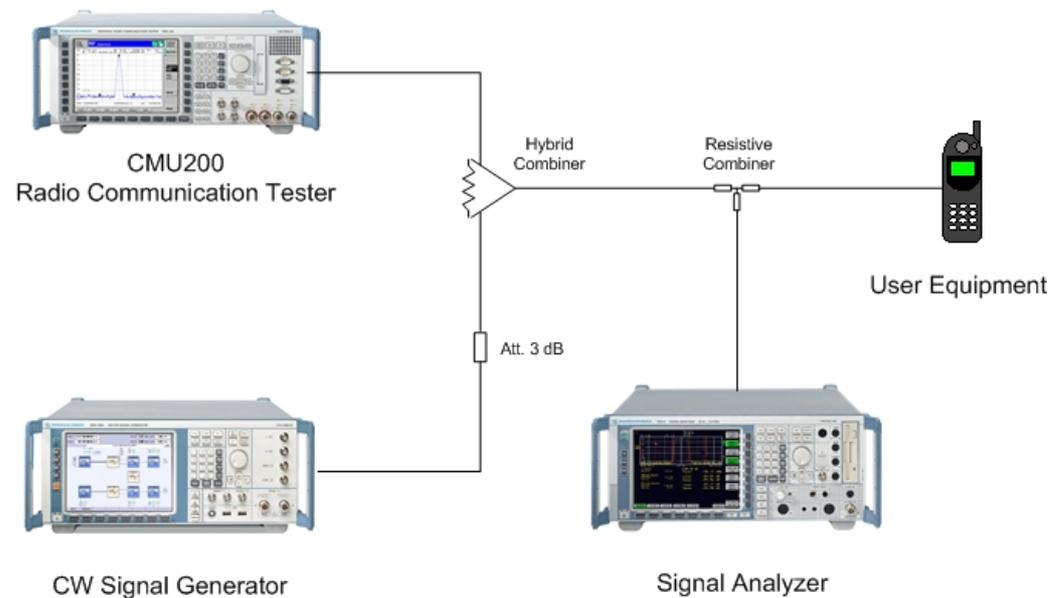
**Fig. 10: Test setup for Transmit Intermodulation test**
