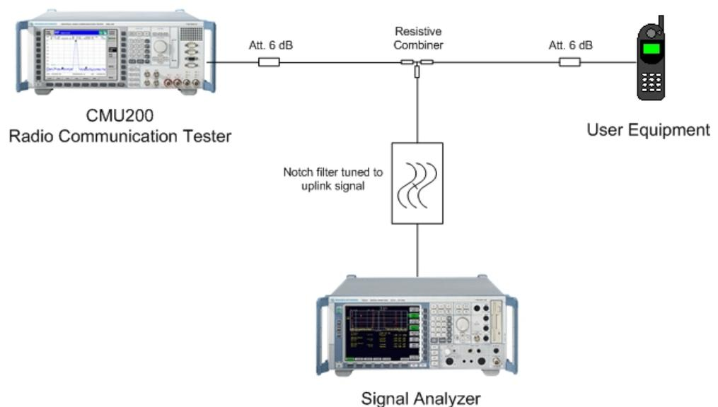
**Fig. 5: Test setup for Spurious Emissions test**
