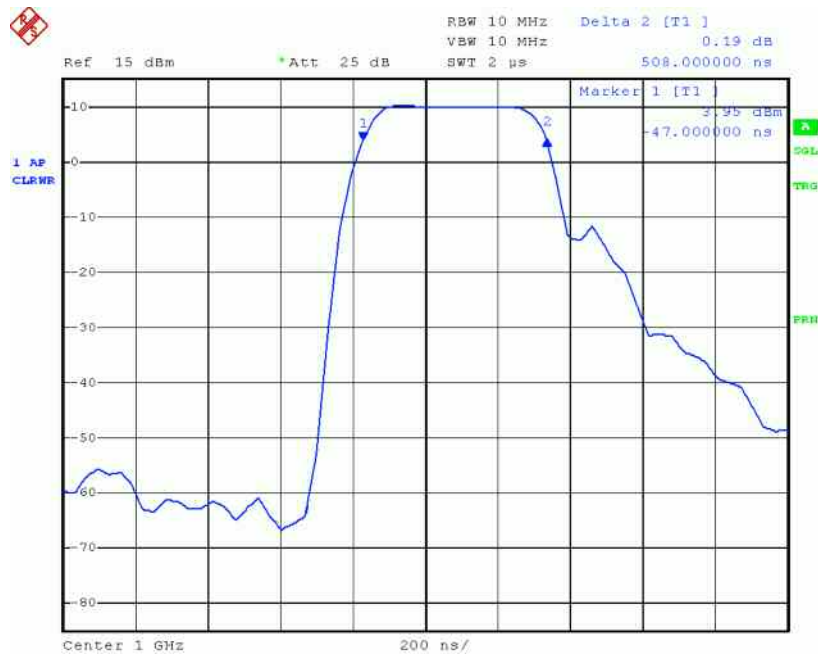
Figure 15. Pulse width is usually defined as the point at which the signal level is at 50% of its average voltage across the pulse length.
