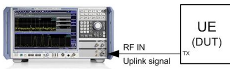
Fig. 37 Basic test setup for user equipment TX.
