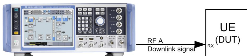
Fig. 13 Basic downlink test setup.
