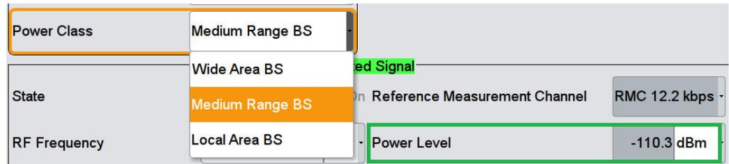
Fig. 3-10: Select the BS power class to set the power level. Example: Medium range BS results in a power level of -110.3 dBm.
