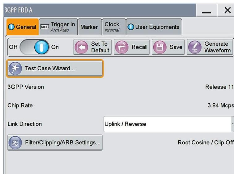
Fig. 3-6: Open Test case wizard for easy and convenient generation of signal according to standard
