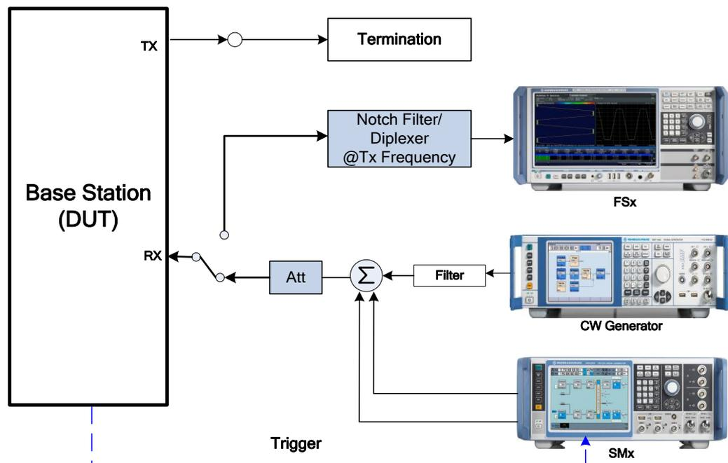
Fig. 2-1: General test setup for Rx test. Additional settings are required for some tests.
