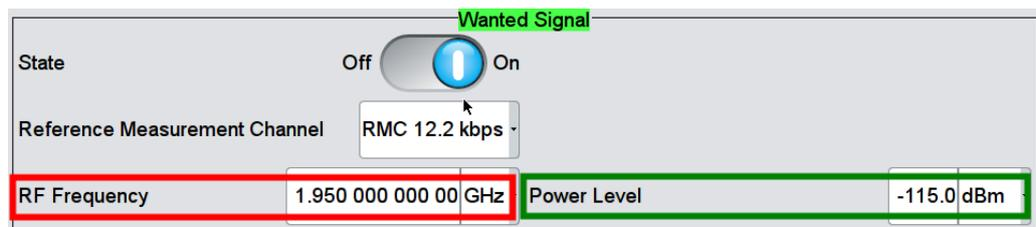
Fig. 3-36: Set reference measurement channel, RF frequency and Power level of the wanted signal
