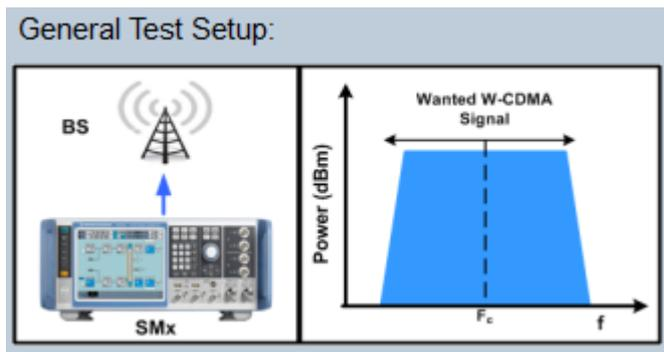
Fig. 3-17: The Test Setup section (bottom right) displays a basic setup for the selected test case along with the location of the signals in the spectrum.
