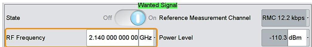
Fig. 3-11: Set the RF frequency
