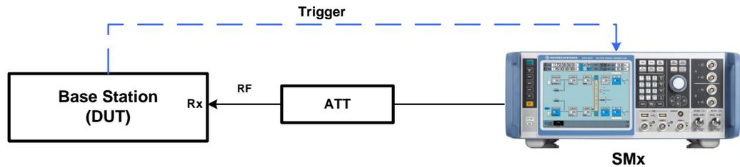
Fig. 3-22: Test Setup for Dynamic range. The SMx generates the wanted W-CDMA uplink reference measurement channel and the AWGN interferer.
