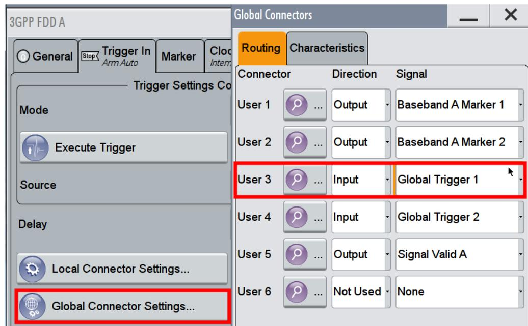
Fig. 3-5: SMW: Configure the connector settings. Example: for the current configuration, Trigger 1 has to be supplied at the input connector USER 3.
