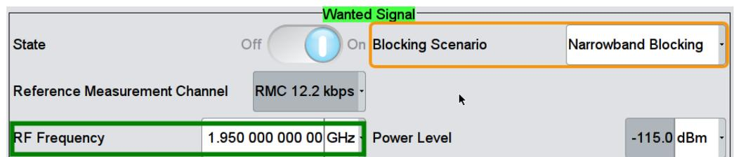
Fig. 3-41: Select Narrowband Blocking. Set RF Frequency
