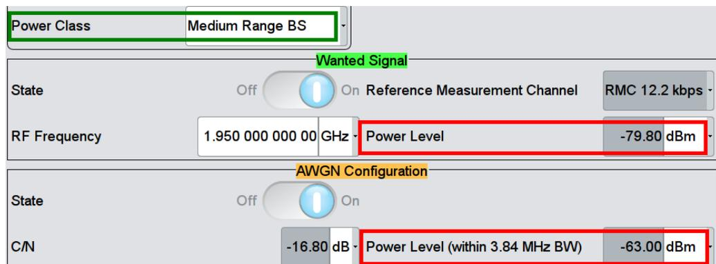
Fig. 3-23: Select power class to set wanted signal power and AWGN power level. Example: for medium range BS , wanted signal power is set as -79.8 dBm and AWGN is set as -63 dBm (according to standard)
