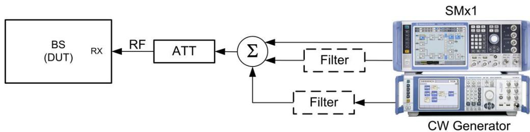
**Fig. 3-32: Test setup for blocking characteristics.** The SMx generates the wanted W-CDMA signal and the interfering signal with two paths. The CW generator provides the CW interferer up to 12.75 GHz
