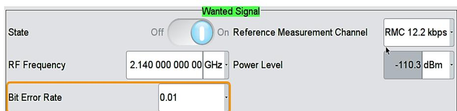
Fig. 3-59: Set Bit error rate of the wanted signal
