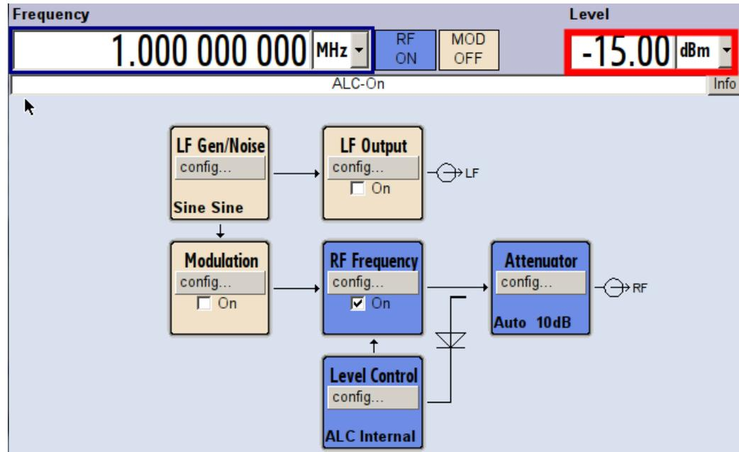
Fig. 3-38: CWx: set RF frequency and Power level of CW signal
