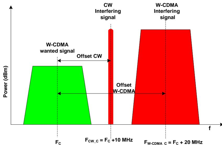
Fig. 3-45: Intermodulation performance. W-CDMA and CW interfering signals cause interference in the wanted signal frequency band.
