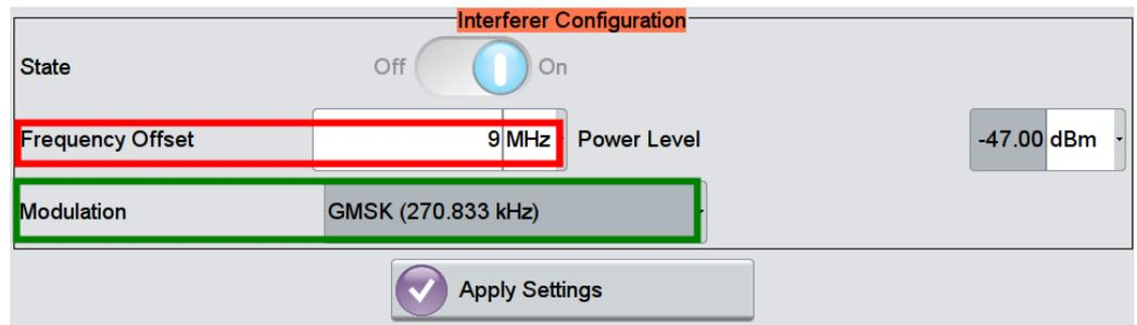
Fig. 3-42: Set Frequency Offset. GMSK modulation is set automatically.
