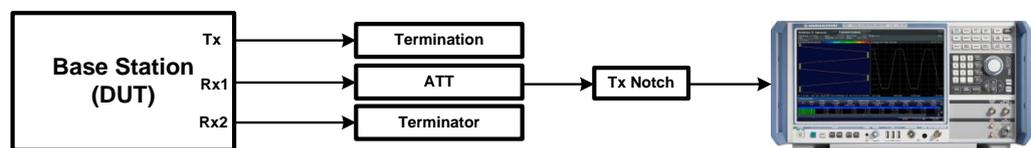
Fig. 3-51: Receiver spurious emission test setup. A notch filter suppresses the Tx signal
