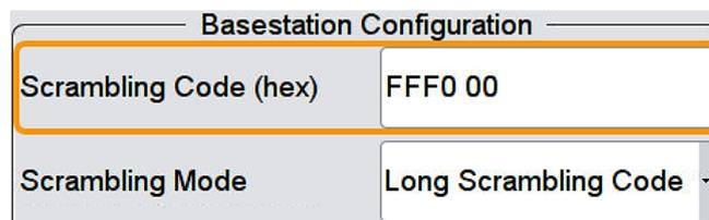
Fig. 3-9: Enter the scrambling code and select the mode
