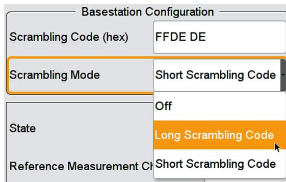
Fig. 3-35: Set scrambling code and scrambling code mode of the wanted W-CDMA signal
