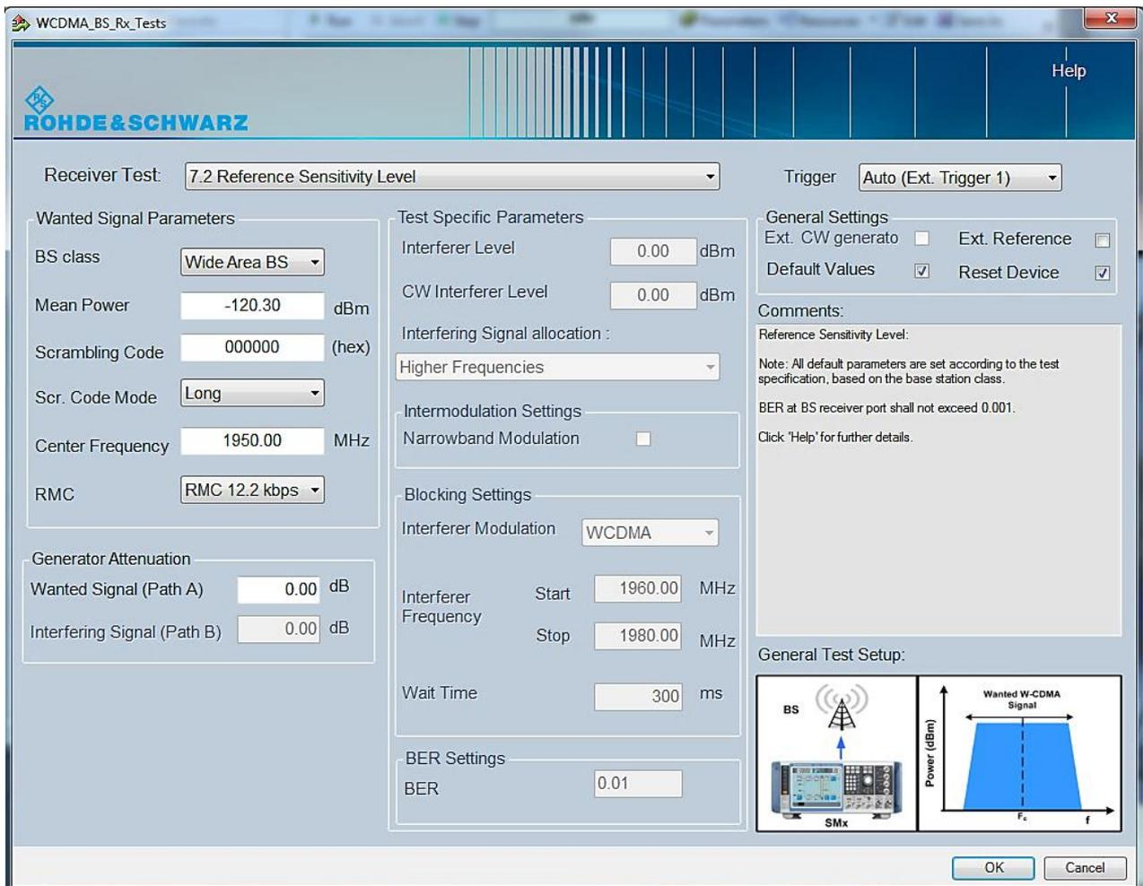
Fig. 3-12: Full overview: setting parameters for the W-CDMA BS Rx test
