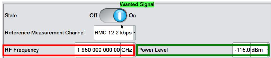
Fig. 3-36: Set reference measurement channel, RF frequency and Power level of the wanted signal
