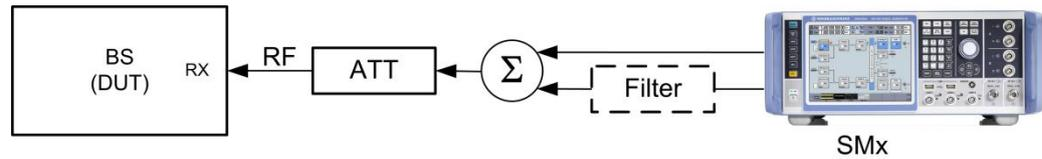
Fig. 3-46: Test setup for Intermodulation characteristics. The SMx generates the wanted W-CDMA signal and the interfering signal with two paths.
