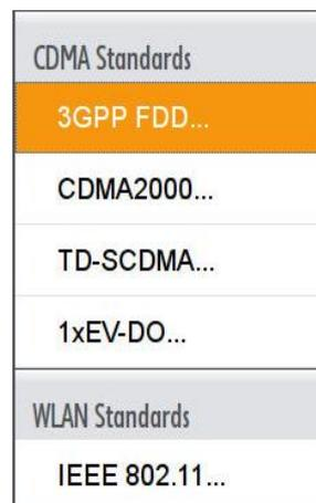
Fig. 3-2: Select 3GPP FDD for W-CDMA signal
