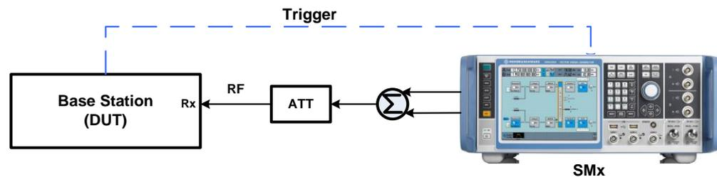
Fig. 3-27: Test Setup for ACS Test. The SMx generates the wanted W-CDMA uplink signal and the interfering W-CDMA signal at  $\pm 5$  MHz offset frequency with two paths.
