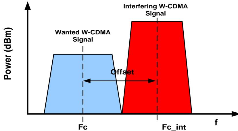
Fig. 3-26: Adjacent channel selectivity. An interfering W-CDMA signal is placed at an offset of  $\pm 5$  MHz
