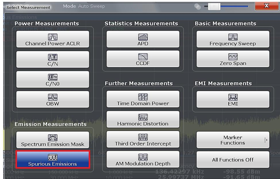
Fig. 3-52: Select spurious emissions via hardkey MEAS
