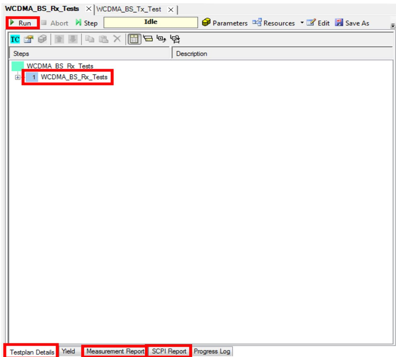
Fig. 4-2: Overview of a test plan in R&S RUN. The test plan in the example contains only one test (WCDMA\_BS\_Rx\_Tests). After the test is completed, the bar along the bottom can be used to display the measurement and SCPI reports.
