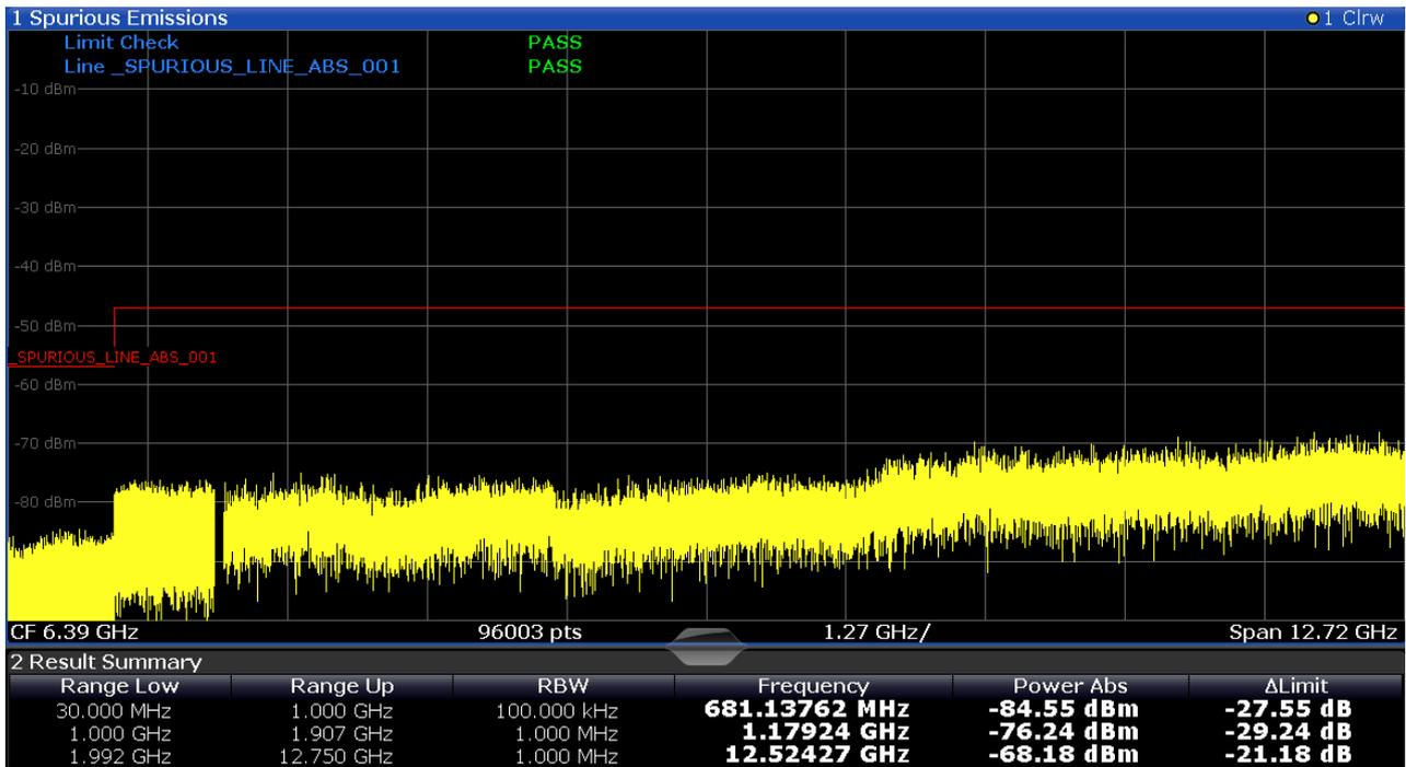
Fig. 3-54: Result for spurious emission. Limit check shows “Pass” if spurious emission remains below the limit. Measurements for individual range are shown in the result summary section
