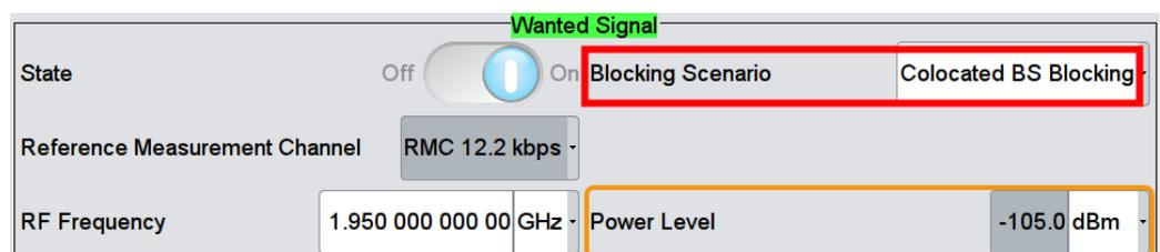
Fig. 3-39: Set blocking scenario as Colocated BS Blocking. Set Frequency
