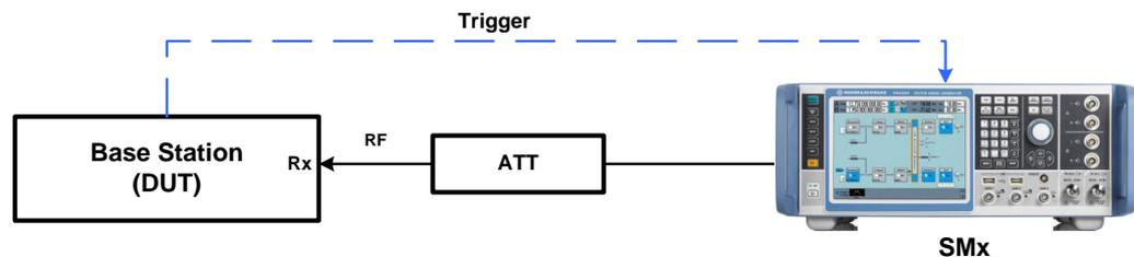
Fig. 3-58: Verification of the internal BER calculation test setup. The SMx generates the W-CDMA uplink reference measurement channel with data rate 12.2 kbps.
