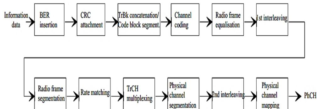
Fig. 3-57: BER insertion into the information data [1]
