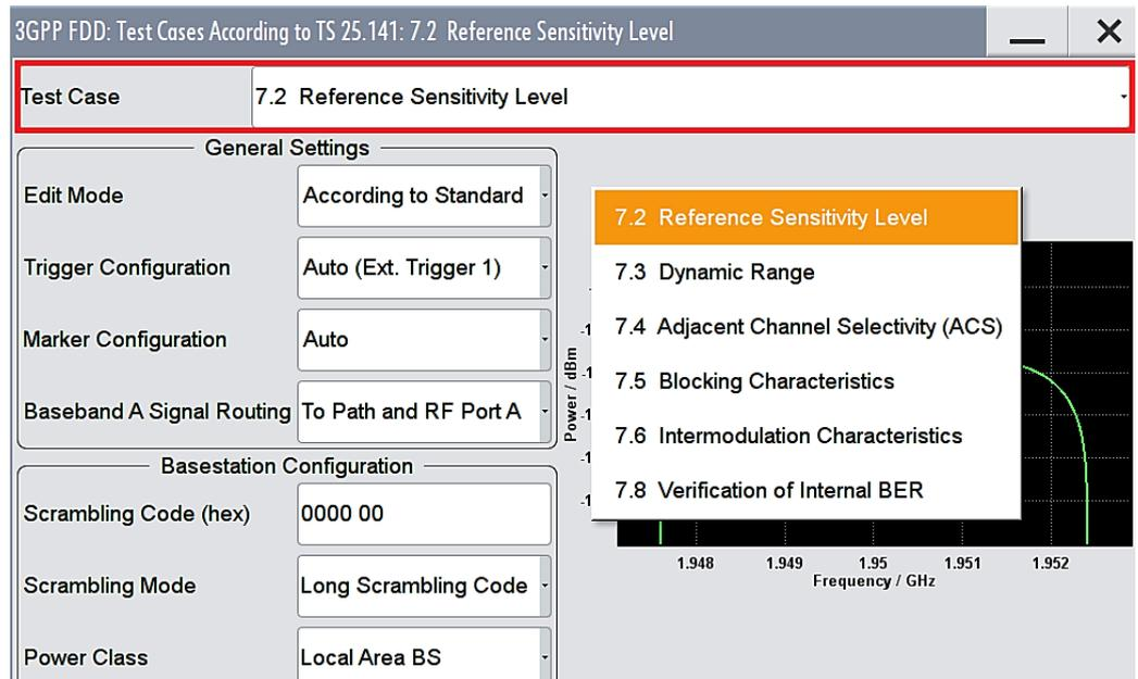
Fig. 3-7: Select the desired test to be performed. Example: “7.2 Reference sensitivity level”
