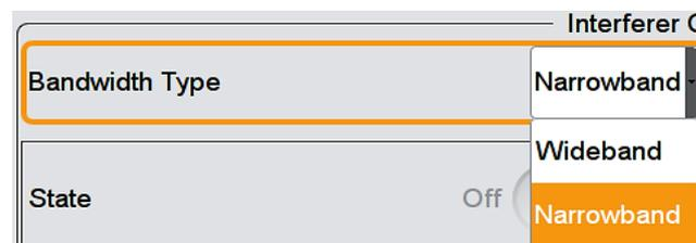
Fig. 3-47: Set bandwidth type of the interferer (Example: narrowband is chosen here).
