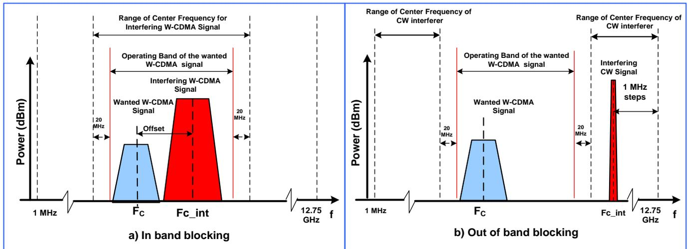
Fig. 3-31: Wideband blocking example. Fig a) shows in-band blocking with W-CDMA interferer where the center frequency of the interfering signal is within the operating band  $\pm 20$  MHz range. Fig b) shows out-of-band blocking with CW interferer where the center frequency of the interfering signal is out of the operating band  $\pm 20$  MHz range.
