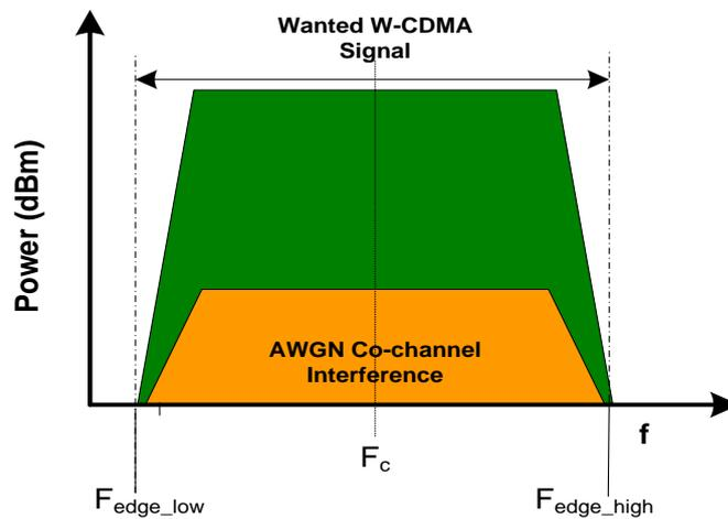
Fig. 3-21: Receiver dynamic range. W-CDMA carrier with AWGN interferer
