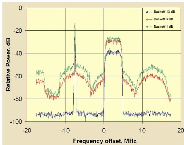
Figure 3. Output Spectrum,  $P_{GSM}/P_{WCDMA} = 0$  dB
