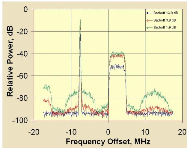
Figure 2. Output Spectrum,  $P_{GSM}/P_{WCDMA} = 15$  dB
