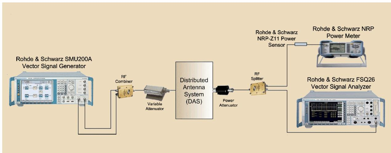
Figure 1. Measurement Setup Diagram
