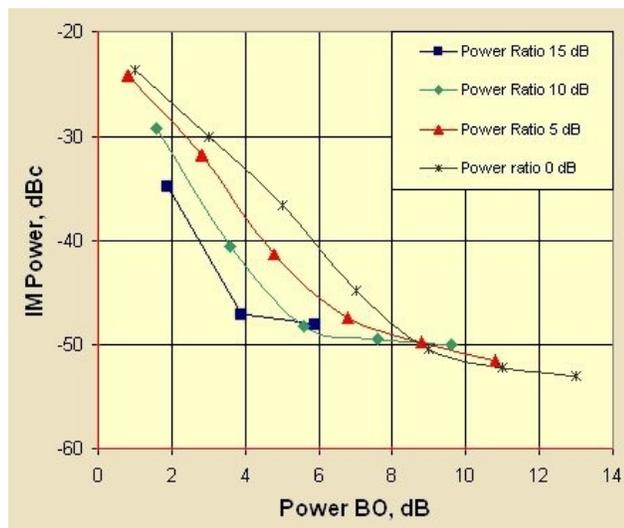
Figure 4. Relative IM Power Versus Power BO
