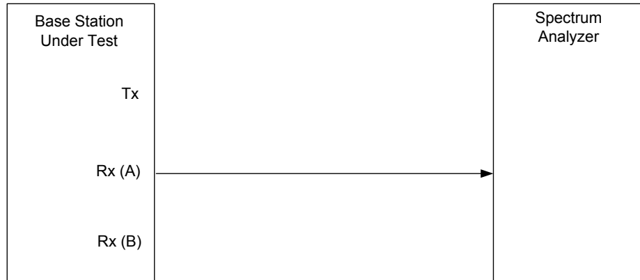
Figure 22 - Test setup: conducted spurious emissions
