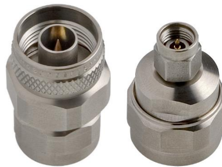
Figure 5-4: Test Port Adapter Heads with male Type-N (left) and male precision 3.5 mm (right).
