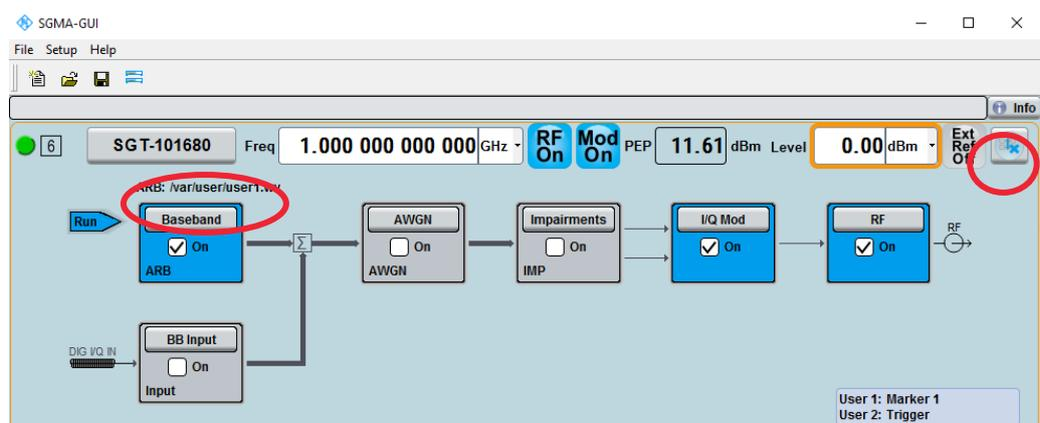
R&S®SGT100A. Check if the at step 2 entered file name is shown.
