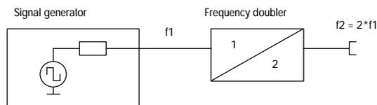
Fig. 1: Signal generator with frequency doubler
