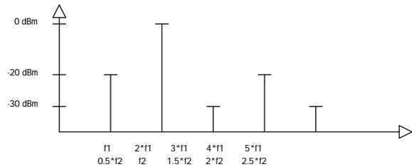
Figure 2: Output spectrum with doubler
