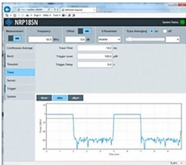
Figure 12. LAN-capable sensors with built-in Web servers enable real-time monitoring and manual control from multiple locations.
