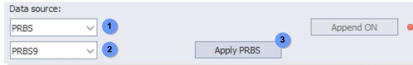
**Figure 22: Data Input – Data Source Section (PRBS)**
