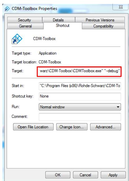
**Figure 8: CDM-Toolbox – Start with Command Line Parameter (--debug)**
