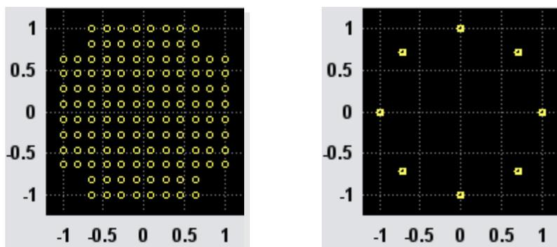
**Figure 2: Constellation Diagrams (left: 128QAM, right: 8PSK)**
