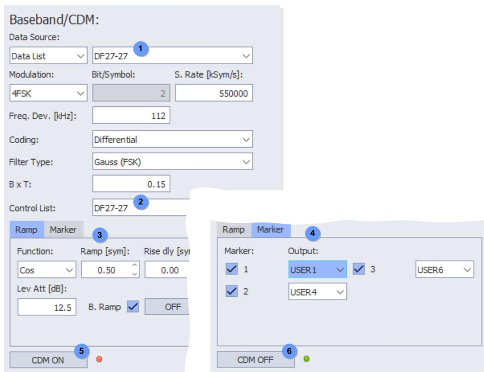
**Figure 15: Path A Tab – Baseband/CDM Section**
