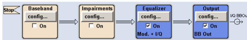
Note that the software configures both equalizers of the AFQ: “Modulator” and “I/Q”.
