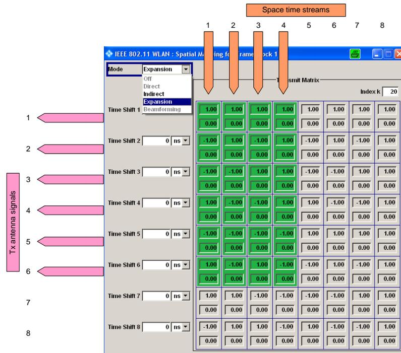
In this example, four space time streams are mapped to six Tx antennas by spatial expansion.
