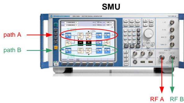
The SMU can be equipped with a 2.2 GHz, 3 GHz, 4 GHz or 6 GHz RF path and a second 2.2 GHz or 3 GHz RF path. The SMW and SMATE can be equipped with a 3 GHz or 6 GHz RF path and a second 3 GHz or 6 GHz RF path.
