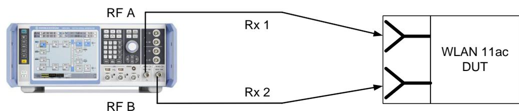
The remaining Rx signals cannot be routed directly to a baseband output but can be saved to a file by selecting “File” as output. The generated waveform files can then be played back via the internal ARB generators of further instruments. For example, to generate the Rx signals Rx3 and Rx4, e.g. two SMBVs are needed. Each SMBV plays back one of the generated waveform files and outputs the corresponding Rx signal at the RF output.
