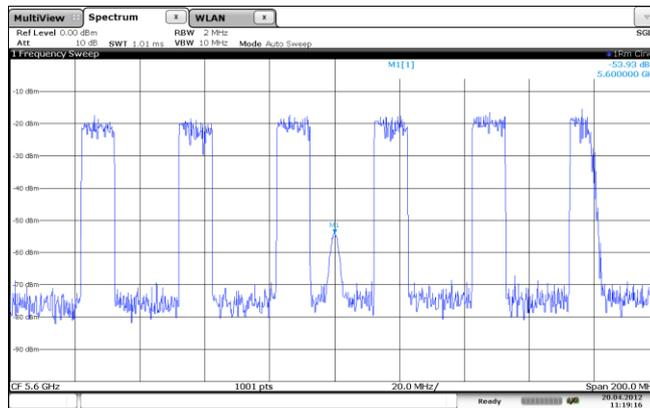
The carrier leakage is caused by a DC component in the I/Q signal. It can be suppressed by adjusting the I and Q offset of the I/Q impairments settings in the upconverter.
