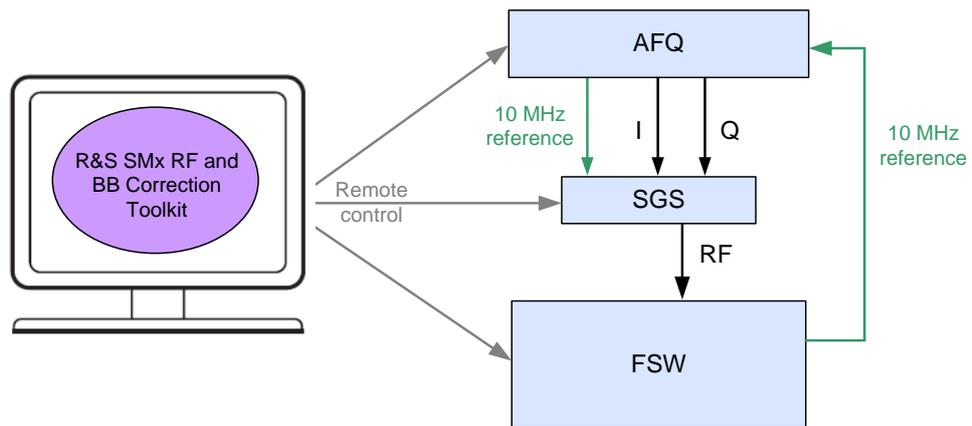
Open the software and select “AFQ Calibration” under the “Configuration” tab. Select the 10 MHz reference source.
