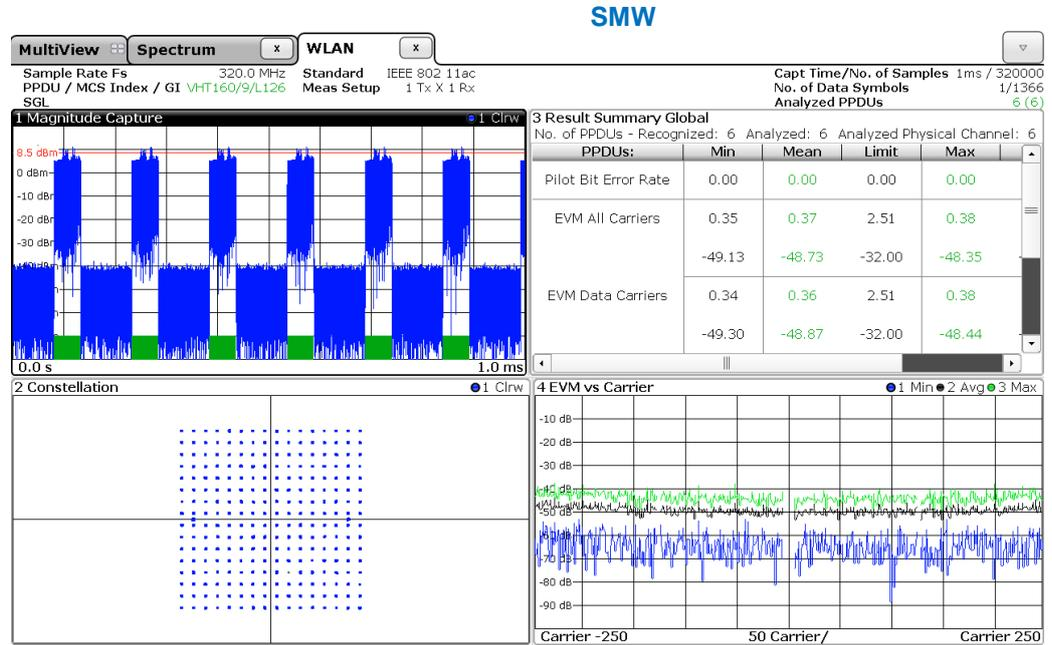
The measured EVM is  $-48.7$  dB (0.37 %) for a 160 MHz signal with 256 QAM modulation.
