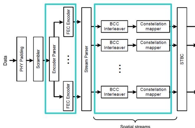
Choose a modulation and coding scheme (MCS). All related parameters are set automatically. Alternatively, you can select the modulation type (BPSK, QPSK, 16QAM, 64QAM, 256QAM) to be applied to the spatial streams. The binary convolution coding (BCC) is enabled by default. Low density parity check (LDPC) coding is also supported. Depending on the selected MCS, the number of forward error correction (FEC) encoders to use is set automatically.
