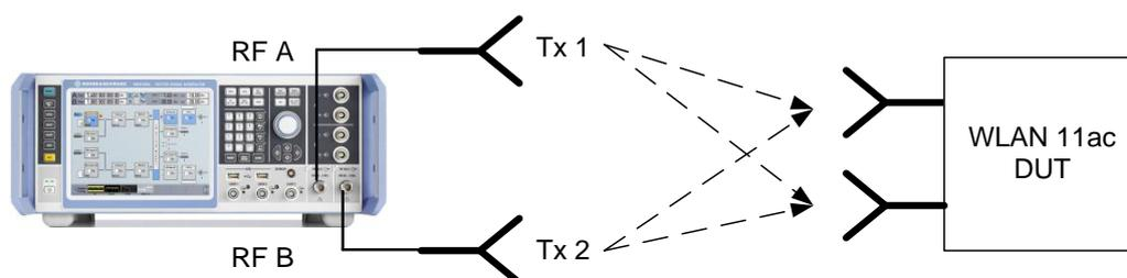
The remaining Tx signals cannot be routed directly to a baseband output but can be saved to a file by selecting “File” as output. The generated waveform files can then be played back via the internal ARB generators of further instruments. For example, to generate the Tx signals Tx3 to Tx8, e.g. six SMBVs are needed. Each SMBV plays back one of the generated waveform files and outputs the corresponding Tx signal at the RF output.
