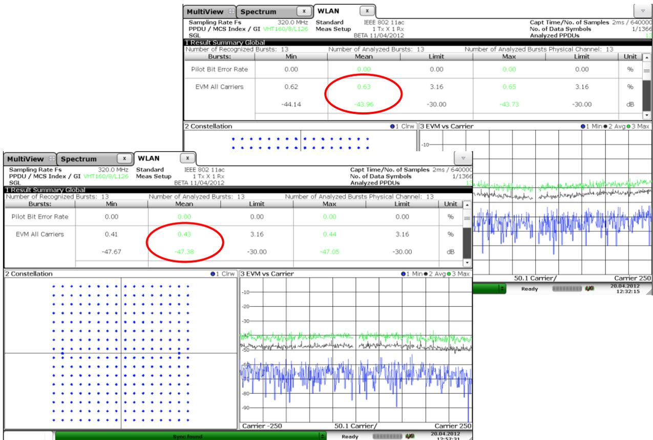
The measured EVM for a 160 MHz signal with 256 QAM modulation is  $-44$  dB before and  $-47$  dB after the calibration.
