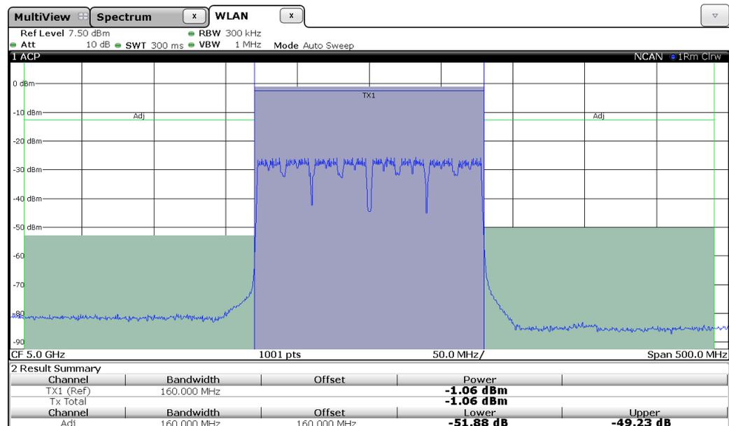
The measured channel power is  $-1.1$  dBm. The result matches (apart from cable loss) the RF level set at the SMW.
