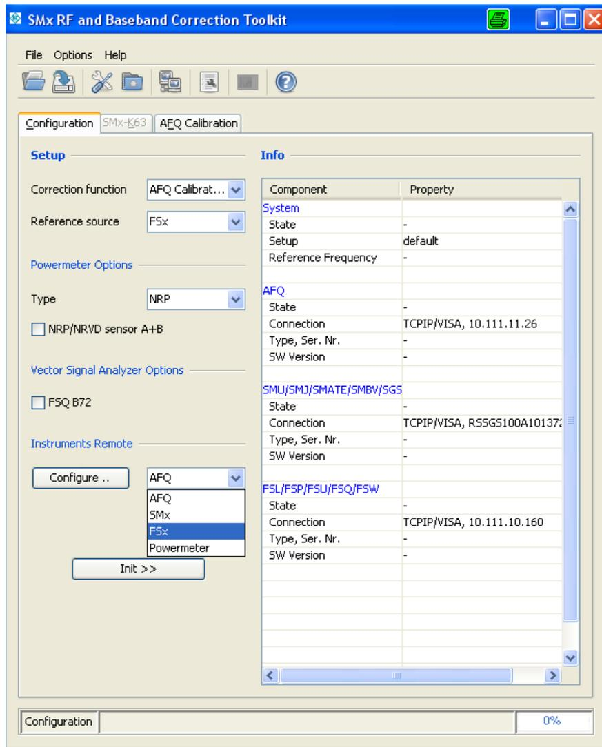
Select the remote interface, e.g. “TCPIP/VISA”. Connect the instrument via LAN to the control PC and enter the IP address of the instrument. Use the “Test Connection” button to quickly test the remote connection.
