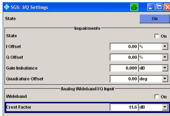
Since the signal is fed in from external and is thus unknown to the SGS, the user needs to provide information about the crest factor of the input signal. The SGS can determine the RMS level of the signal from the peak amplitude (500 mV expected) and the entered crest factor value. This enables the instrument to level its RF output correctly which is important if the channel power of the WLAN 11ac signal is to be measured.
