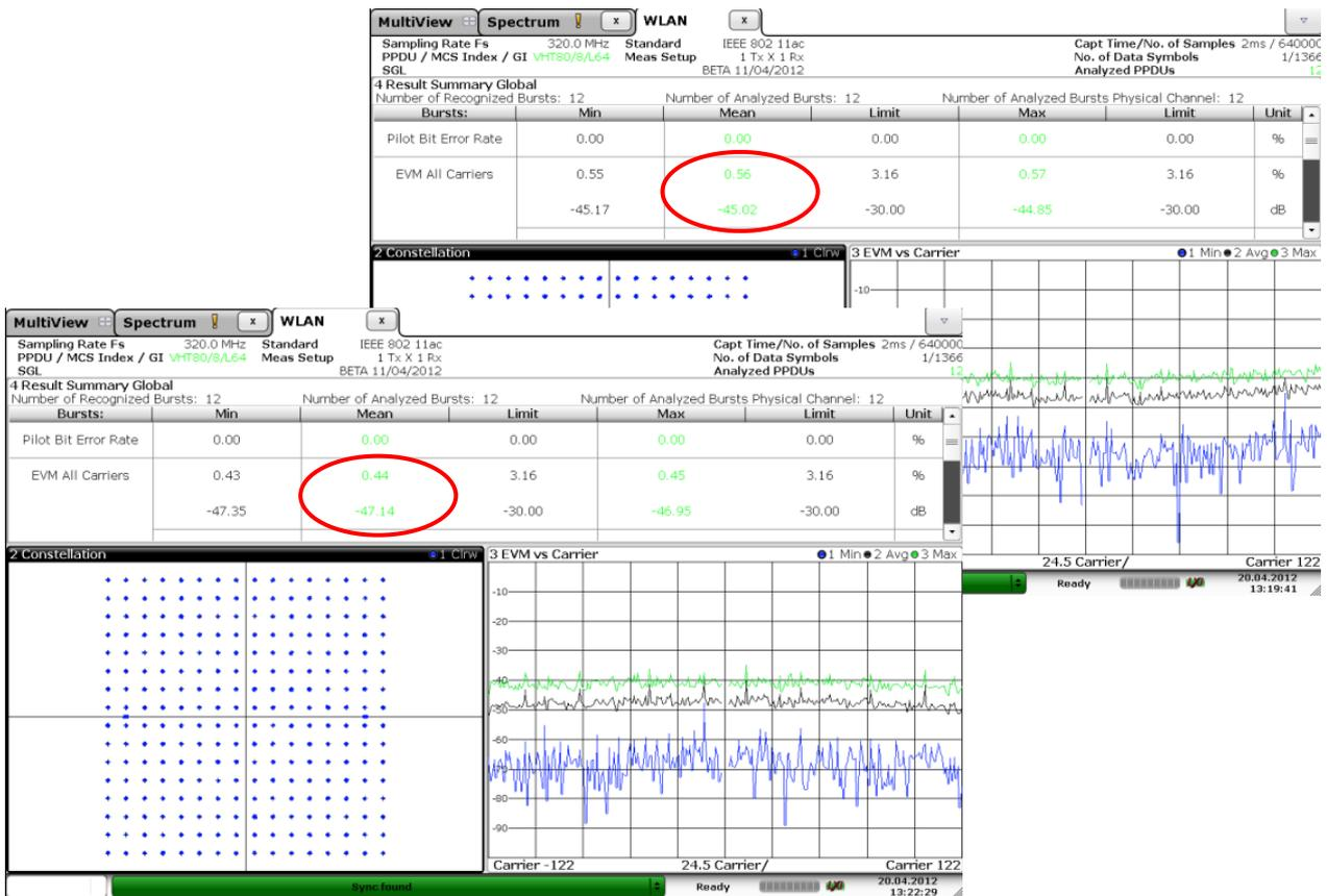
The measured EVM for an 80 MHz signal with 256 QAM modulation is  $-45$  dB before and  $-47$  dB after the adjustment.
