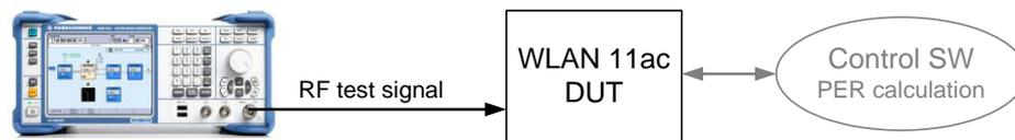
For PER measurements, e.g. 1000 frames are generated and evaluated. Set the desired number of frames in the frame blocks configuration menu.
