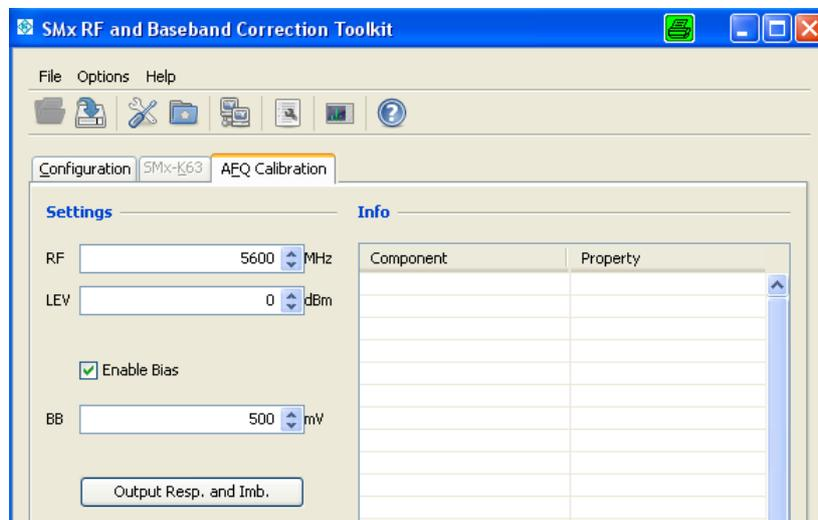
Start the calibration by pressing the “Output Resp. and Imb.” button. While the calibration is running, the following window is displayed:
