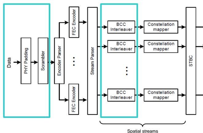
You can define the size of the data field or alternatively the number of data symbols. The scrambler uses either a fixed, selectable initialization value or a random initialization value that is different for each frame. The interleaver is enabled by default.
