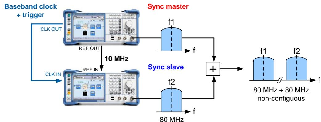
One SMBV acts as master instrument and supplies all necessary synchronization signals to the slave instrument via just two connection cables. The master-slave setup is simple, easy to configure and provides highly synchronized test signals. It is described in detail in the application note "Time Synchronous Signals with Multiple R&S SMBV100A Vector Signal Generators" (1GP84).
