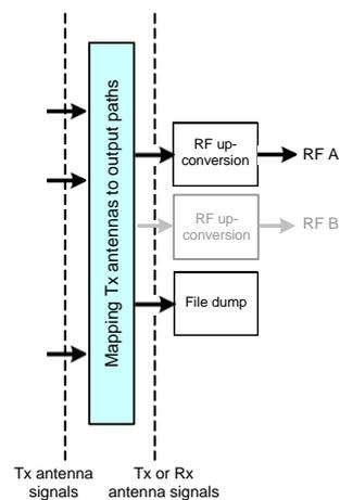
The Tx antenna signals (Tx1 to Tx8) are mapped to the baseband output. The mapping determines if a single Tx signal or multiple superimposed Tx signals are present at the output of the baseband. By mapping multiple Tx signals to the baseband output, these signals are combined and form an Rx signal that can be used for MIMO testing (see section 4.2.5.2 for background information).
