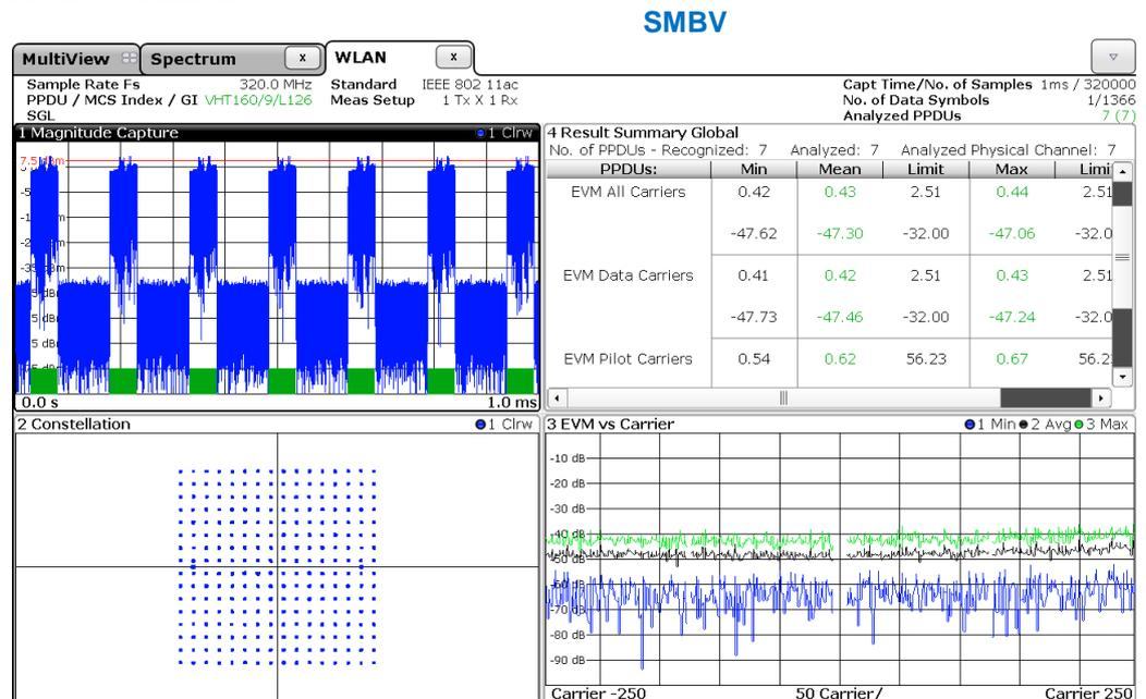
The measured EVM is  $-47.3$  dB (0.43 %) for a 160 MHz signal with 256 QAM modulation.
