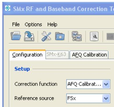
Next, configure the three instruments of the setup: AFQ, SGS (or SMx) and R&S®FSx. Select the instrument and click the “Configure..” button.
