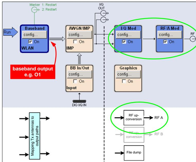
For example, the output signal O2 is routed to “File”. The signal is saved to the hard drive by entering a file path and name in the “File” column for O2.
