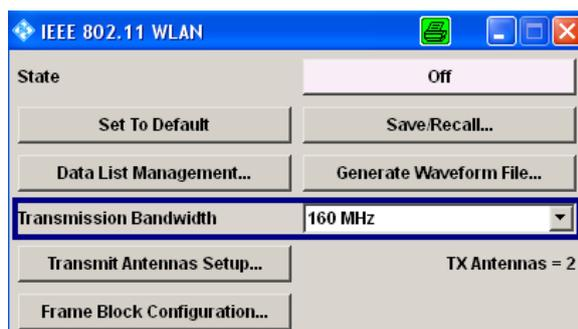
Click the “Transmit Antennas Setup...” button to open the TX Antenna Setup menu. Set the “Antennas” parameter to the desired number of Tx antenna signals to be generated.
