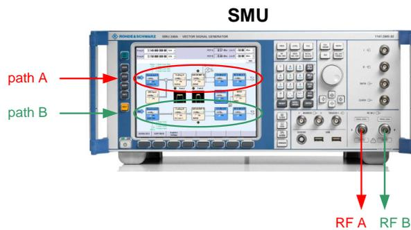
The SMU can be equipped with a 2.2 GHz, 3 GHz, 4 GHz or 6 GHz RF path and a second 2.2 GHz or 3 GHz RF path. The SMW and SMATE can be equipped with a 3 GHz or 6 GHz RF path and a second 3 GHz or 6 GHz RF path.
