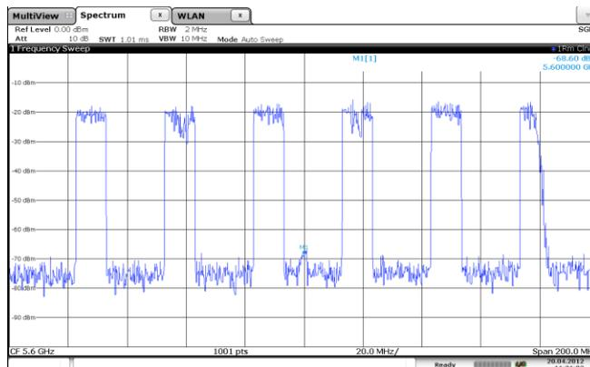
Note that the carrier leakage has no effect on the measured EVM of the WLAN 11ac signal (since there is no OFDM carrier at the carrier frequency).
