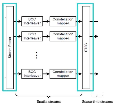
The scrambled and encoded data is distributed to one, two, three, four, five, six, seven or eight spatial streams.
