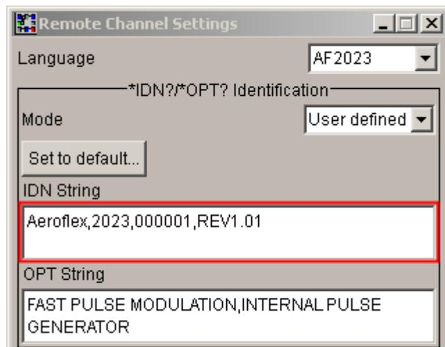
Finally select the OPT String text box and edit the response text to \*OPT? queries. When finished, confirm the text:
