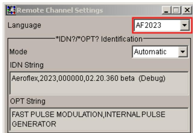
Select the Mode and open the drop-down list. Pick either "Automatic" or "User defined" from the list and confirm the selection. In "Automatic" mode, the response text to \*IDN? and \*OPT? queries is generated by the signal generator itself. In "User defined" mode, the response text to \*IDN? and \*OPT? queries must be entered in the corresponding IDN string and/or OPT string text boxes:
