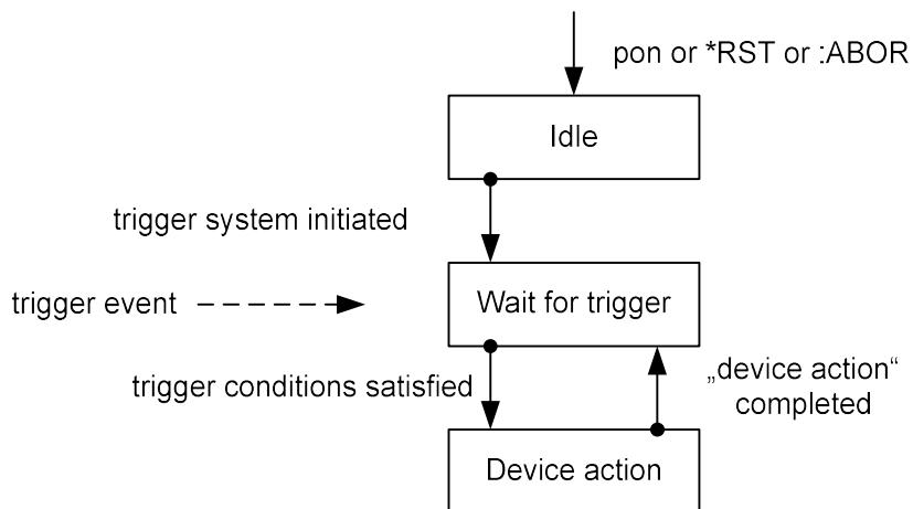
The main difference between the emulated instrument's and the SMB's trigger control system is that there is no "Initiated" state in the SMB. The SMB implementation assumes that the trigger system is initiated automatically in the "Idle" state. As a result, any sweep operation in the SMB, once activated, can only be controlled by internal or external trigger events.
