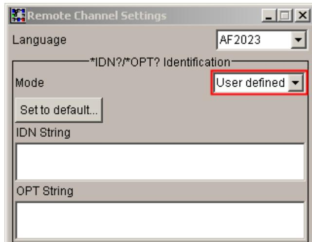
In “User defined” mode, press the “Set to default...” button to preset the corresponding IDN string and/or OPT string text boxes with the default settings from the selected remote emulation:
