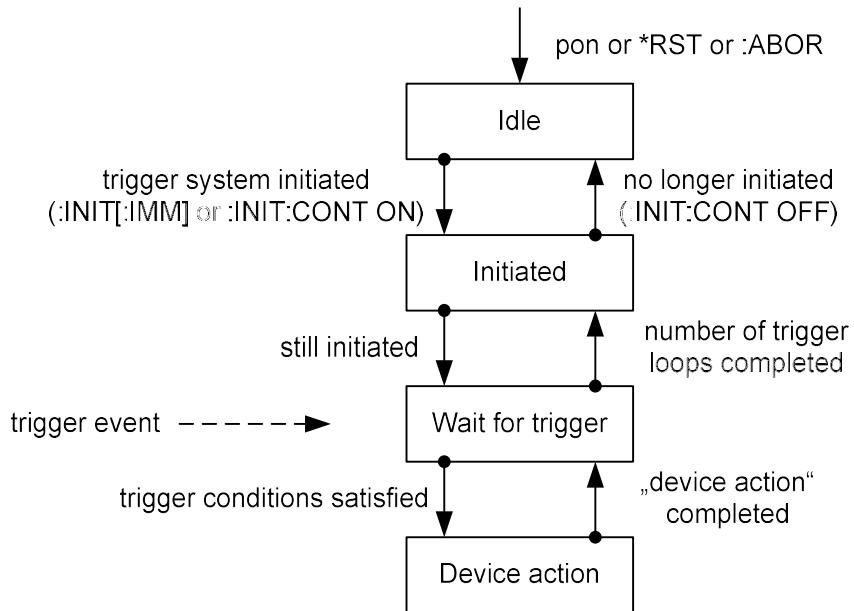
Other emulated instruments and also the SMB implement the trigger control system shown in the following figure:
