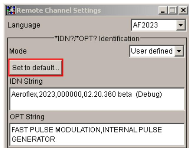
Then select the IDN String text box and edit the response text to \*IDN? queries. When finished, confirm the text:
