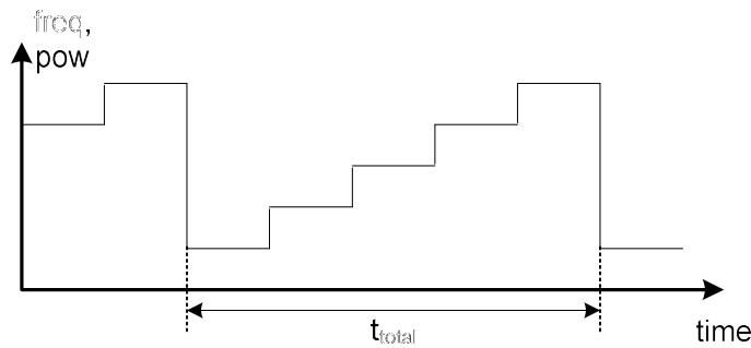
Changing the start, stop or steps parameter of the sweep operation does not have an impact on the total sweep time.
