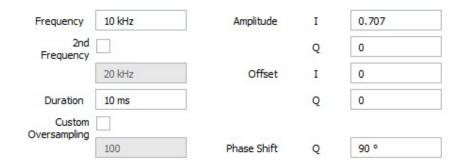
Setting a second frequency creates a frequency sweep. The result is a waveform that starts with the signal frequency and ends with the second frequency. The duration defines the amount of time in which the frequency changes.
