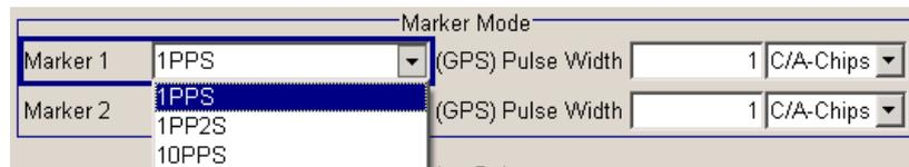
The marker signal, i.e. the 1PPS signal generated by the SMBV and the 1PPS signal generated by the receiver, can be compared by means of an oscilloscope (e.g. R&S RTO) and the timing accuracy can be measured. In this setup, the SMBV's 1PPS signal serves as the timing reference.
