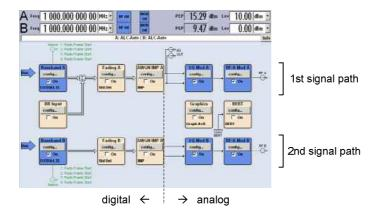
The two-path concept makes it possible to combine the two baseband signals internally. The SMU offers different routing possibilities that can be set via the "Baseband" block and/or the "Fading" block. The routing is done in the digital domain of the SMU, which enables lossless signal addition with highest precision.
