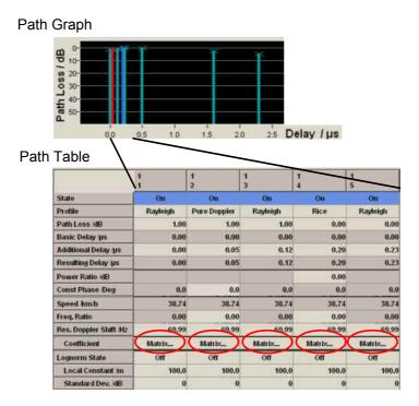
Note that the relative levels set with the matrix are only effective if the fading simulators are turned on. Nevertheless, the MIMO routing can also be used without fading simulation<sup>1</sup>. If fading is unwanted, a single fading path with a static fading profile can be selected. This setting effectively means no fading.
