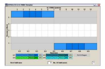
The occupied signal bandwidth is thus not 1.08 MHz but only 1.08 MHz / 6 = 180 MHz. In the LTE standard, the SNR is related to average power per (allocated) resource element. For this reason, the relevant noise level is the noise level within the occupied signal bandwidth. The noise level within a bandwidth of 180 kHz is -97.48 dBm.
