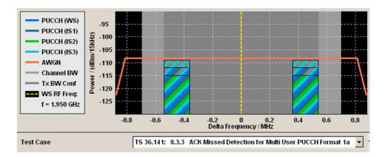
The test case wizard is the most easy-to-use solution for conformance testing of LTE base stations. Nevertheless, we use the test case 8.3.3 of TS 36.141as an advanced example to explain how to perform the signal routing, baseband leveling and AWGN setting manually for this practical test.
