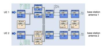
UE 1 is simulated by baseband A, and UE 2 by baseband B. UE 1 is faded, UE 2 is unfaded.
