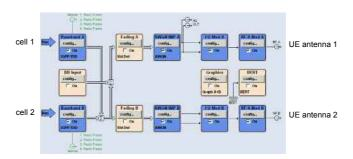
Cell 1 is simulated by baseband A, and cell 2 by baseband B.
