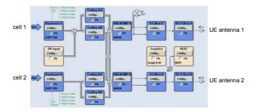
Cell 1 is simulated by baseband A, and cell 2 by baseband B.
