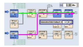
For example, if a summation ratio of –3 dB is set, then the level of baseband B is 3 dB higher, i.e. twice as high as the level of baseband A.
