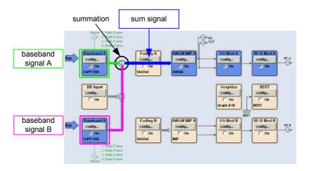
For example, the SNR is set to 7 dB. As a result, the SNR for each baseband is 4 dB (i.e. 3 dB lower) if the two basebands have equal levels. However, if the basebands have unequal levels, the calculation is not that easy.
