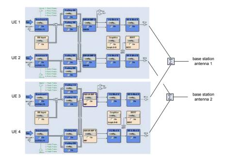
UE 1 is the wanted signal and is simulated by baseband A of SMU 1. UE 2, UE 3 and UE 4 are the interferers and are simulated by baseband B of SMU 1, baseband A of SMU 2 and baseband B of SMU 2, respectively. All four basebands are triggered externally by the base station. The RF outputs A of both instruments are combined externally and connected to antenna 1 of the base station. The RF outputs B of both instruments are also combined externally and connected to antenna 2.
