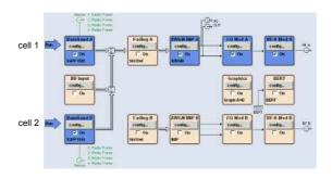
Cell 1 is simulated by baseband A, and cell 2 by baseband B.
