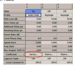
For the fading profiles "Static Path", "Pure Doppler" and "Const. Phase" the matrix reduces to a vector – basically the off-diagonal elements of the MIMO matrix disappear and the diagonal elements form now a vector. The attenuation is entered in dB. For example, fading channels AA and AB can be attenuated by a factor of two relative to channels BA and BB by setting –3.0 for AA and AB. The vector elements BA and BB are set to 0.0 (no attenuation).
