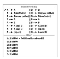
For example, the two baseband signals can be added *after* the fading simulators and routed to RF output A by selecting "A  $\rightarrow$  A, B  $\rightarrow$  A" routing. If, for example, "2x2 MIMO" routing is selected, the baseband signals are faded and added as required for 2x2 MIMO testing.
