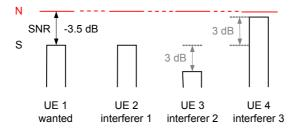
The relative baseband levels are set via the parameter "Power Offset Relative to Level Display". The level of UE 4 is the highest level and thus serves as the reference level for the power offsets. The levels of UE 1, UE 2 and UE3 have to be attenuated accordingly.
