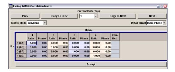
The matrix can be used to set different baseband levels if the baseband signals are added using one of the MIMO routings.
