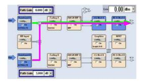
For example, if a path gain of 3 dB is set for path B, then the level of baseband B is 3 dB higher, i.e. twice as high as the level of baseband A.
