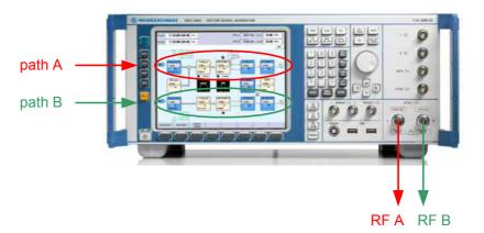
The SMU provides internal realtime fading simulation and additive white Gaussian noise (AWGN) generation. Furthermore, the user can take advantage of the various routing possibilities. For example, the two baseband signals can be combined and routed to one RF port, e.g. for transmit diversity tests. Or one baseband signal can be split and routed to both RF ports, e.g. for receive diversity tests. Even more complex signal routings required for MIMO tests are possible.
