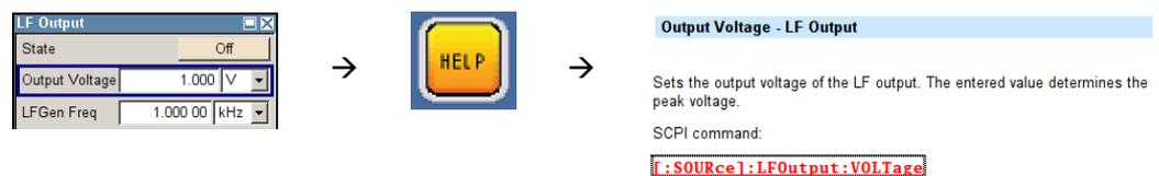
In manual operation via remote desktop or VNC viewer, select a particular setting parameter and then press the "F1" key on your keyboard to open the instrument's online help.
