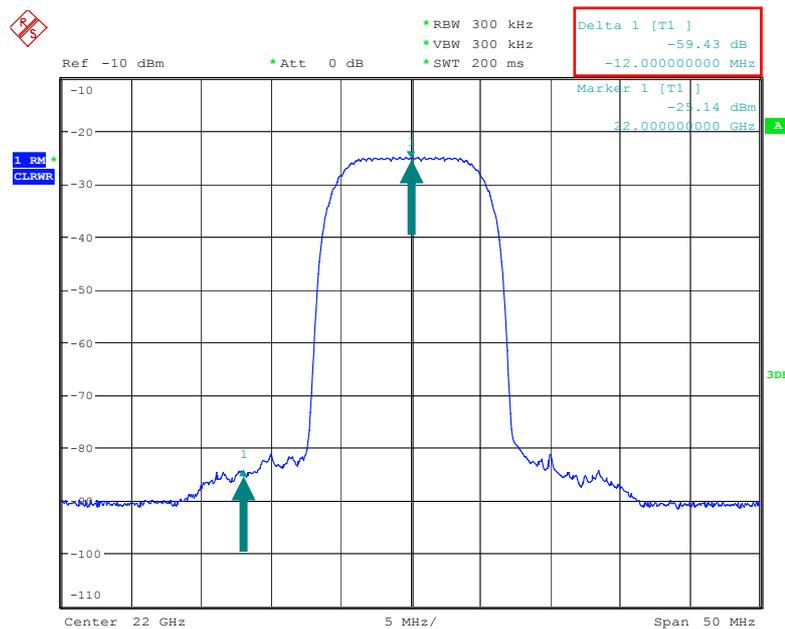
Fig. 26: RF frequency spectrum of the upconverted 16QAM test signal (10 Msym/s).
