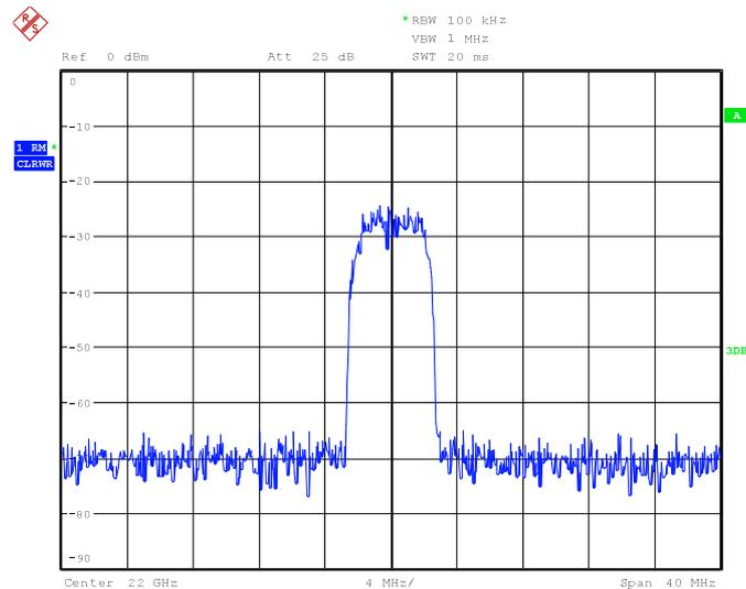
Fig. 8: Frequency spectrum of the vector-modulated microwave signal at 22 GHz. The frequency span is 40 MHz.
