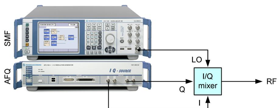
Fig. 3: Example of a test setup for vector signal generation up to 43.5 GHz using two Rohde & Schwarz signal generators and an I/Q mixer.
