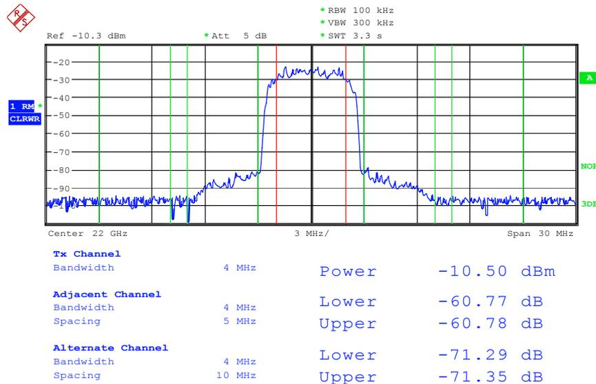
Fig. 10: ACLR measurement of the vector-modulated microwave signal.
