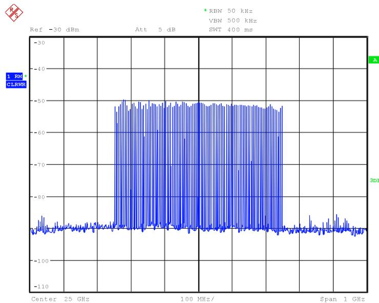
Fig. 12: Multi-tone signal at 25 GHz with a bandwidth of 500 MHz.
