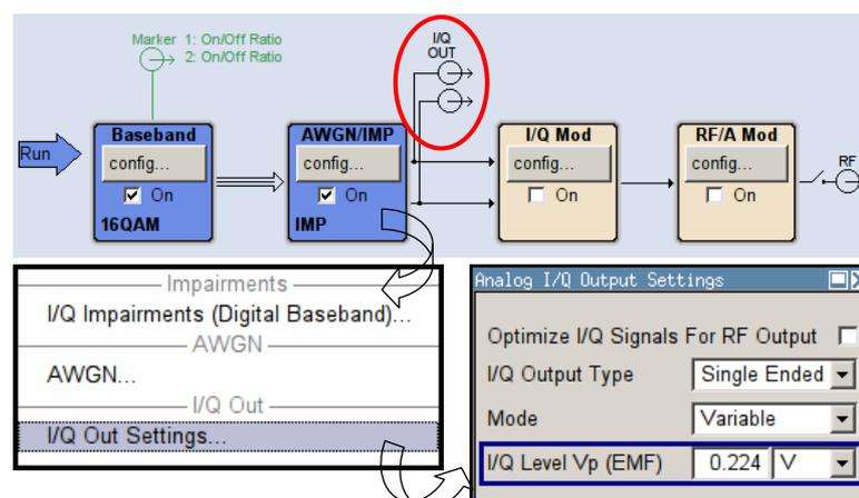
Fig. 21: Details of the graphical user interface of the SMBV showing the settings required for adjusting the IF input power.
