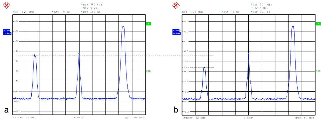
Fig. 14: RF frequency spectrum showing the sideband rejection of the original IF signal (a) and of the IF signal with applied I/Q phase difference (b).
