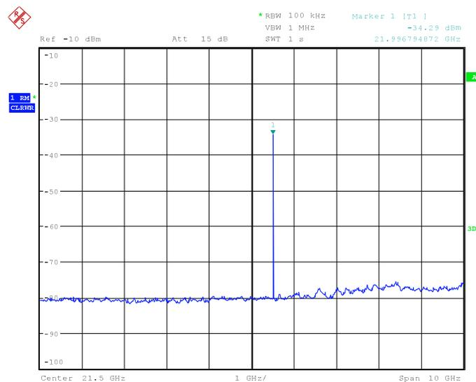
Fig. 7: Frequency spectrum of the vector-modulated microwave signal at 22 GHz. The frequency span is 10 GHz.
