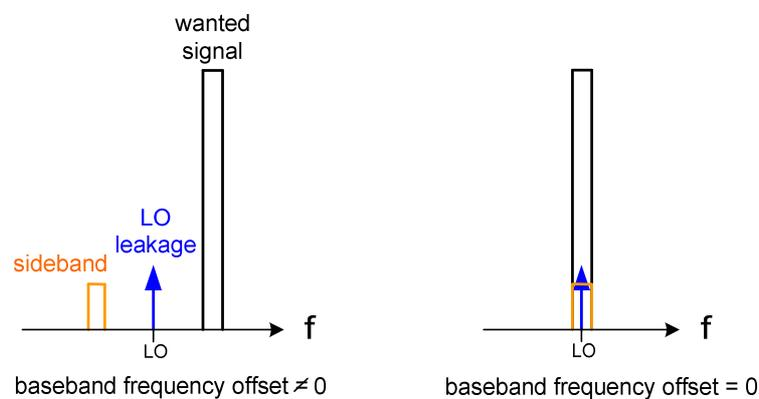
Fig. 2: RF spectrum of an I/Q mixer with and without baseband frequency offset (i.e. IF frequency).
