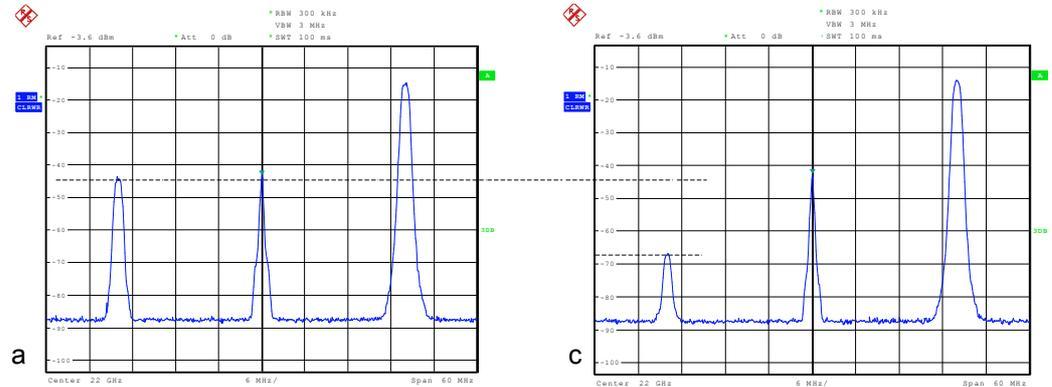
Fig. 16: RF frequency spectrum showing the sideband rejection of the original IF signal (a) and the IF signal with applied I/Q phase difference and I/Q gain imbalance (c).
