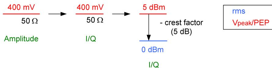
Fig. 6: Calculation of the IF or I/Q level (rms) for the AFQ.
