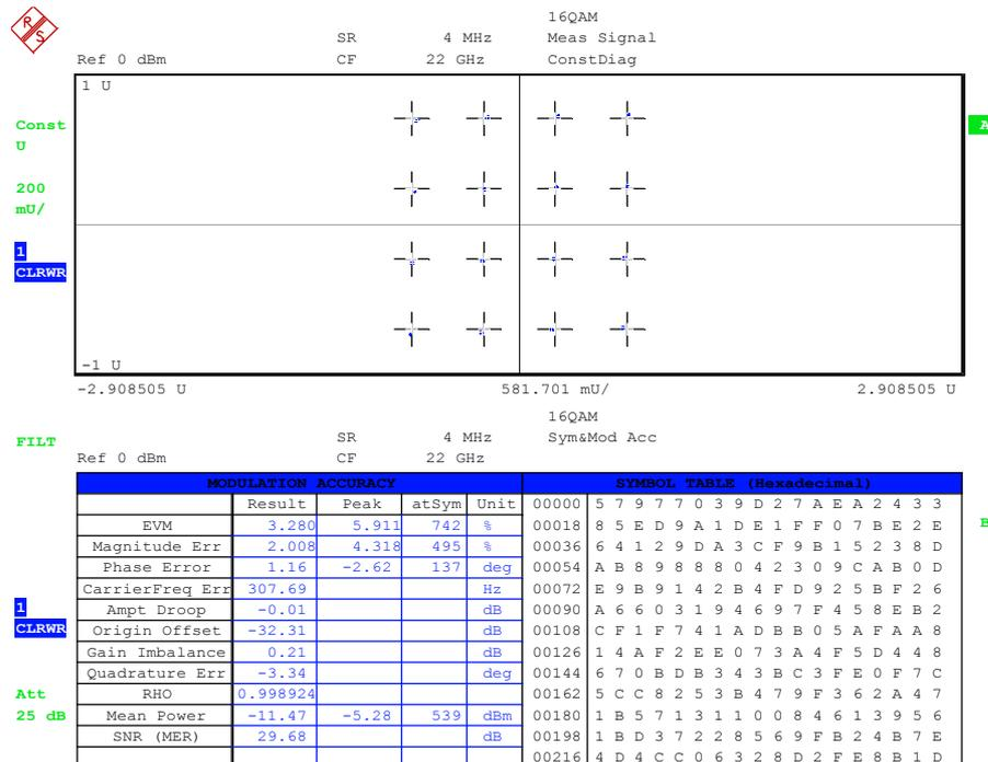
Fig. 9: EVM measurement of the vector-modulated microwave signal.
