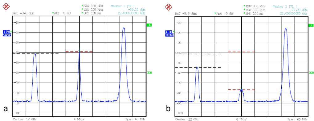
Fig. 25: RF spectrum showing the sideband and LO carrier suppression of the IF signal without (a) and with applied I/Q impairments (b).
