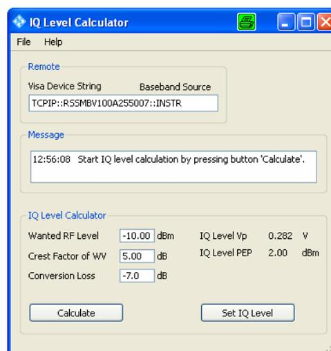
Fig. 11: Graphical user interface of the program IQ Level Calculator (V1.0.0).
