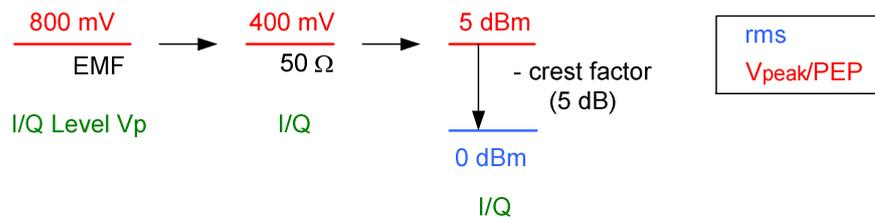
Fig. 22: Calculation of the IF or I/Q level (rms) for the SMBV.
