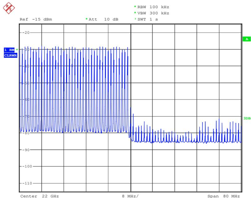
Fig. 29: RF spectrum of the upconverted multi-tone signal visualizing image rejection.
