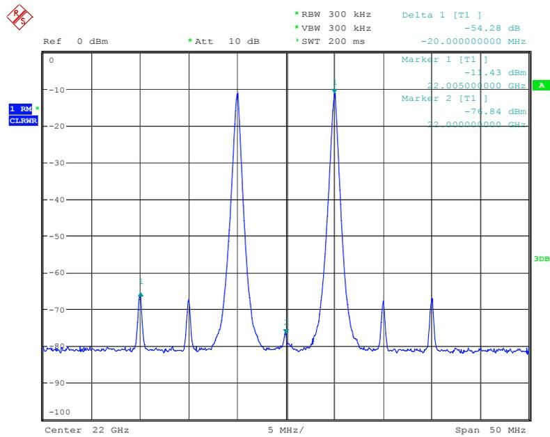
Fig. 27: RF spectrum of the upconverted two-tone signal.
