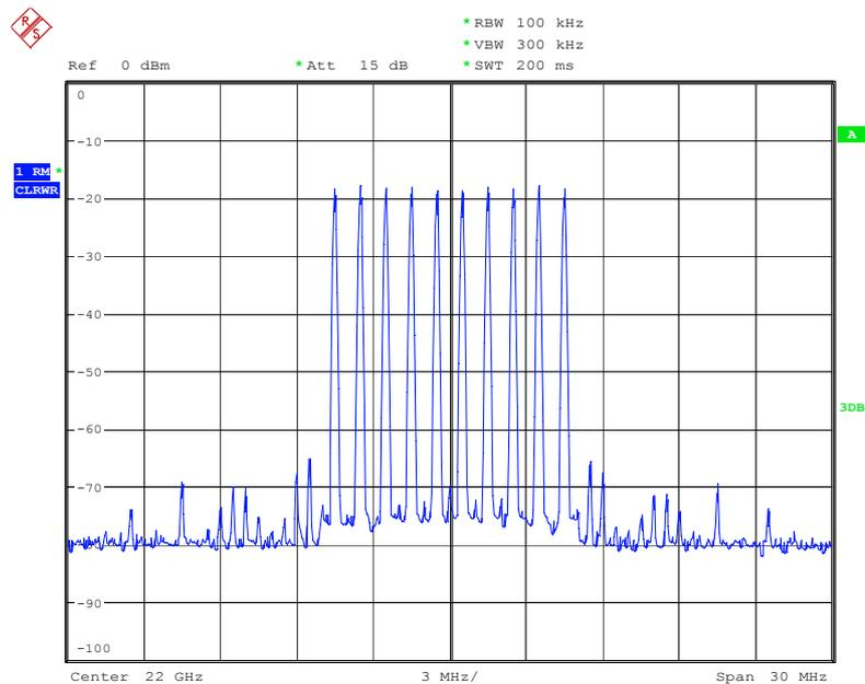
Fig. 28: RF spectrum of the upconverted multi-tone signal.
