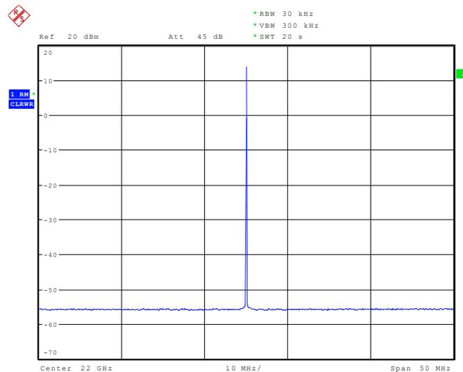
Fig. 4: Frequency spectrum of the 22 GHz LO input signal.
