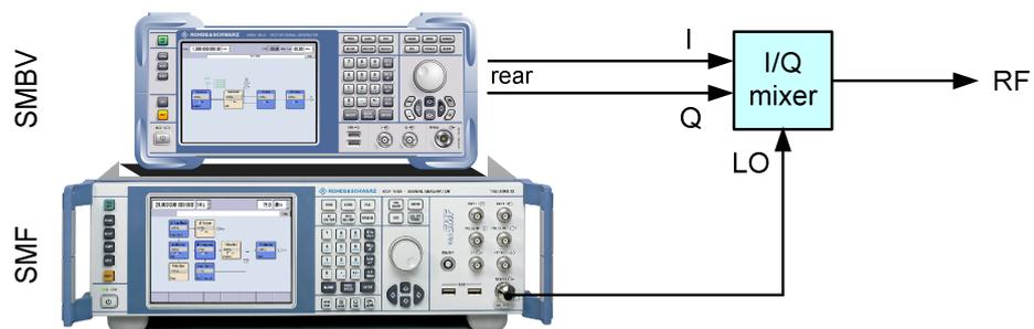
Fig. 20: Schematic of the test setup for vector signal generation using an I/Q mixer.
