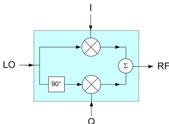
Fig. 1: Input and output signals of an I/Q mixer used as an upconverter.
