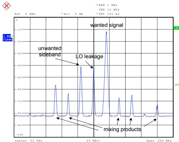
Fig. 13: RF frequency spectrum for an up-converted I/Q signal (16QAM) having a frequency offset of 20 MHz.
