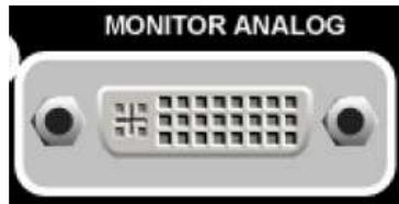
*Fig. 28: Monitor analog connector on the rear panel*
