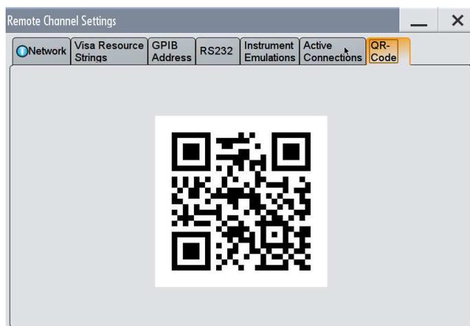
Fig. 26: The instrument address displayed as QR code (SMW only)
