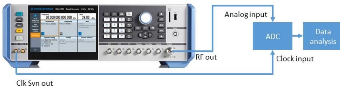
Figure 2 Modern ADC performance test setup
