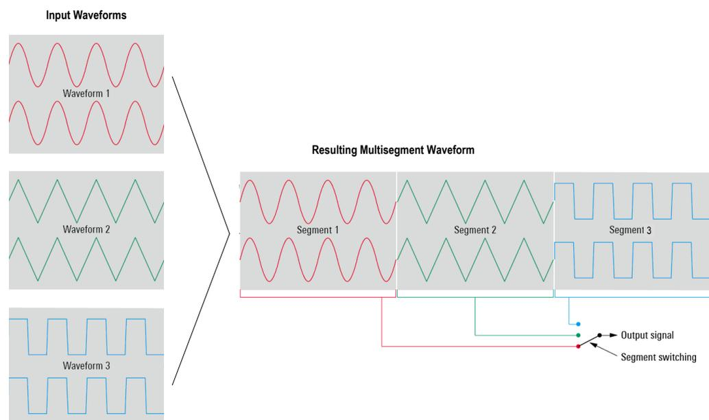
**Fig. 1: Multisegment waveform concept.**
