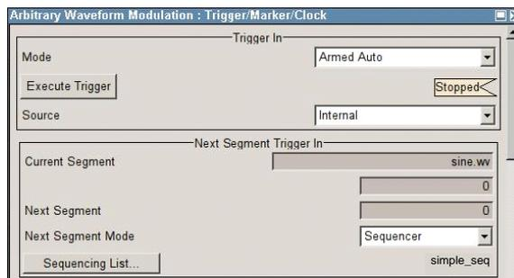
Fig. 8: Required trigger settings for Sequencer Example 1.
