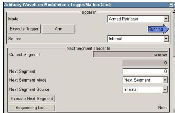
Fig. 5: Required trigger settings for Example 1.
