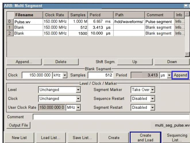
**Fig. 16: Required settings for multisegment waveform generation.**
