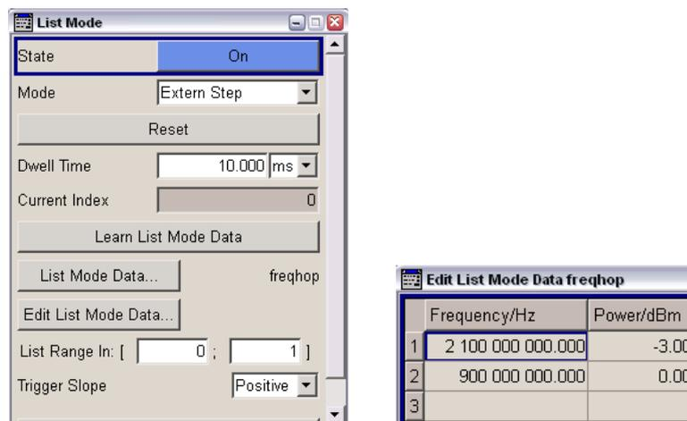
Fig. 24: Required RF list mode settings and RF list mode list.
