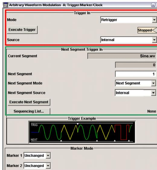
Fig. 3: Trigger/Marker/Clock menu of the arbitrary waveform generator.
