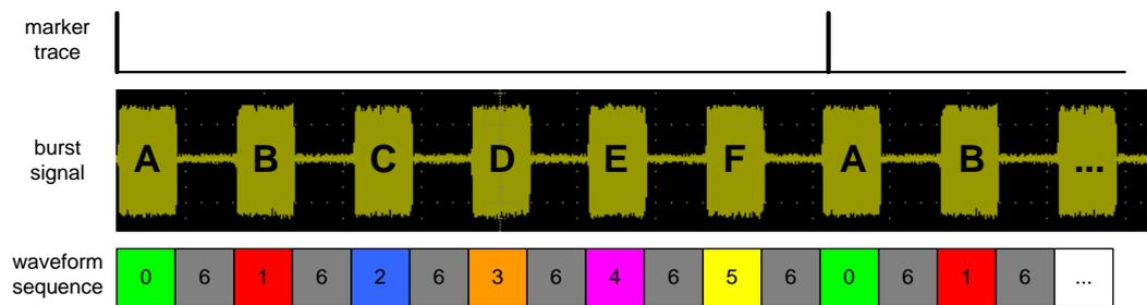
**Fig. 19: Generation of a burst signal via a multisegment waveform.**
