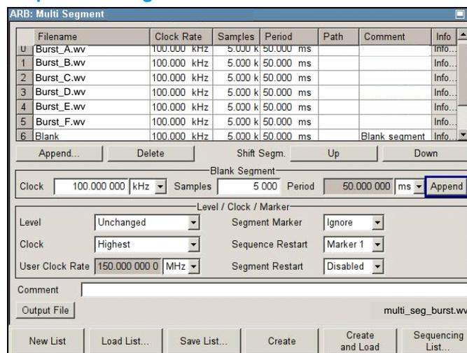
**Fig. 20: Required settings for multisegment waveform generation.**
