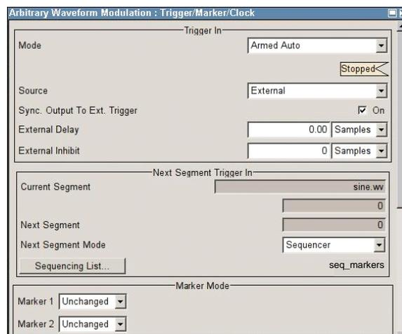
**Fig. 11: Required trigger and marker settings for Sequencer Example 2.**
