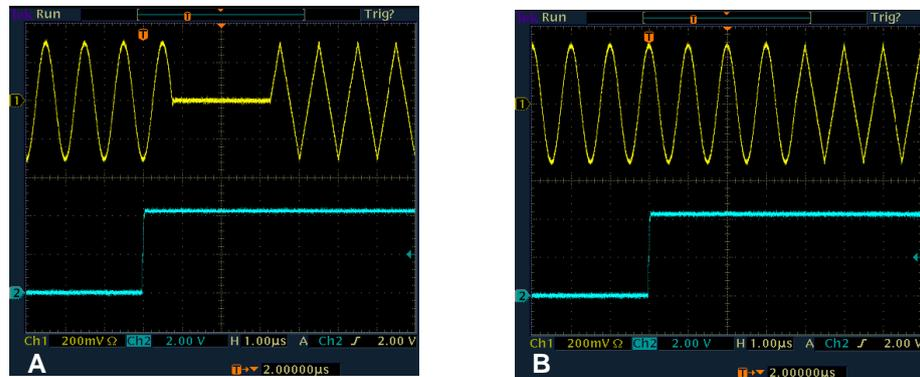
**Fig. 4:** Transition from one segment (sine signal) to another segment (triangle) triggered by an external trigger signal (shown on channel 2). **A:** Normal transition. **B:** Seamless transition.
