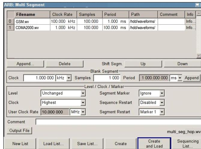
**Fig. 22: Required settings for multisegment waveform generation.**
