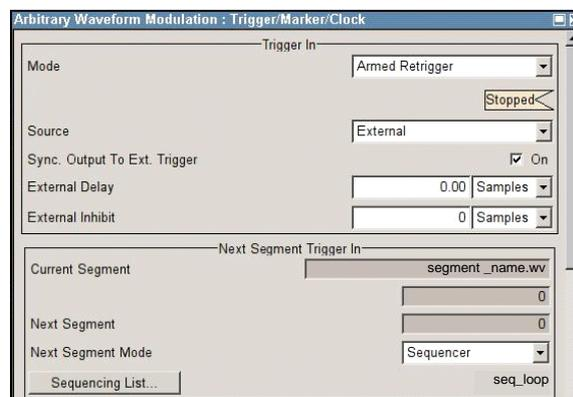
Fig. 13: Required trigger settings for Sequencer Example 3.
