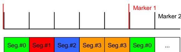
The marker traces must be inserted into the multisegment waveform. This can be easily done during generation of the multisegment waveform (see settings below). Marker signals can be used to trigger a DUT or to synchronize with other measurement instruments, for example. For precise adjustment, it is possible to delay the marker outputs during I/Q signal output without interrupting the signal output.
