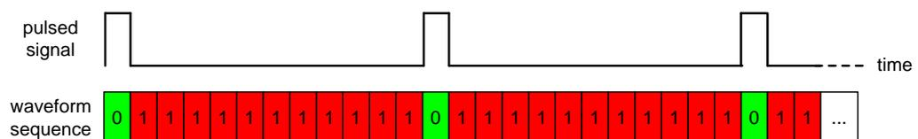
**Fig. 15: Generation of a pulsed signal via a multisegment waveform.**
