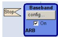
The second step is to turn on the list mode. The first entry in the list is now active, 2100 MHz in our example (although no signal is currently generated).
