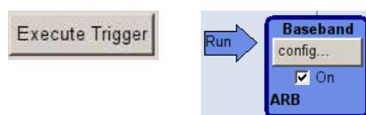
Together with the start of the waveform a marker signal is issued which triggers the list mode to step to the next list entry. The *second* entry in the list is now active, 900 MHz in our example. As a result, the GSM signal is played back at 900 MHz as desired. All further marker events will trigger the list mode to step to the next frequency such that the waveforms are output at alternating RF frequencies.
