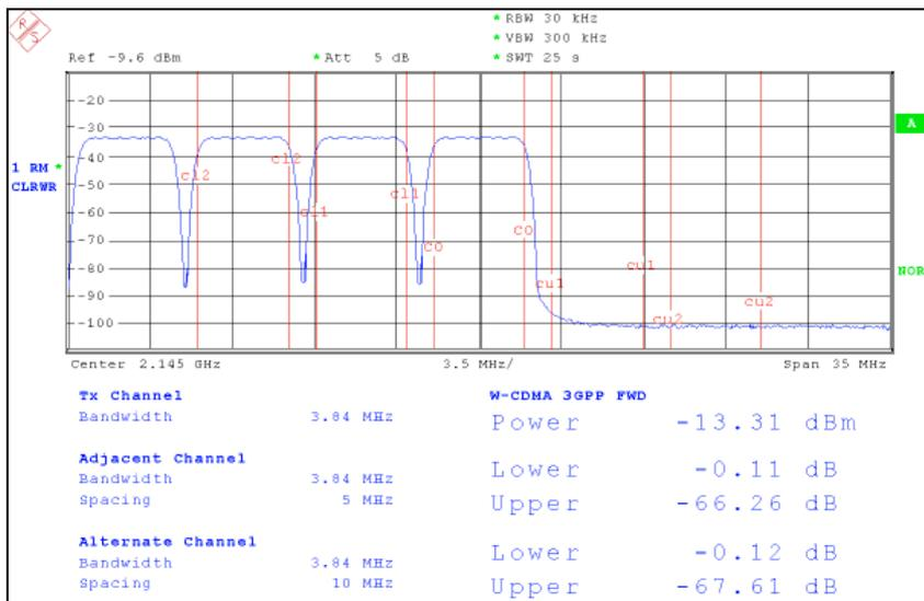
Fig. 6.6: The upper adjacent and 1<sup>st</sup> alternate channel ACLR performance for the same setup and signal as in Fig. 6.5.
