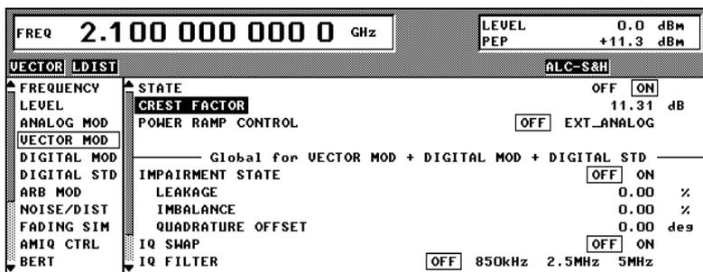
Once the waveform is transmitted to AMIQ the **VECTOR MOD STATE** in the SMIQ is set to **ON**, and the **CREST FACTOR** is automatically set to the correct value.
