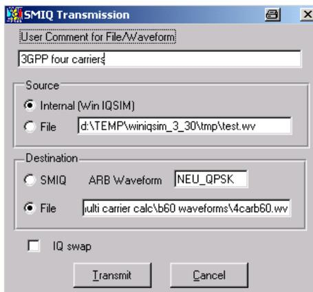
Enter a User File Information in the **User Comment for File/Waveform** text box and a **ARB Waveform** file name in the **Destination** section of the transmission panel.
