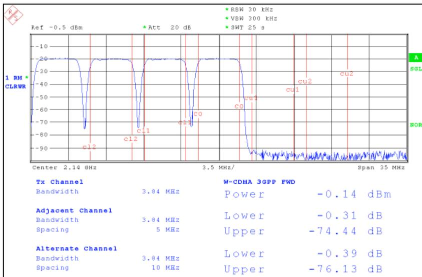
Fig. 6.4: The upper adjacent channel and the upper alternate channel ACLR performance of 4 SMIQ03HD generating a 4 carrier WCDMA/3GPP using the SMIQB57 for each carrier separately.
