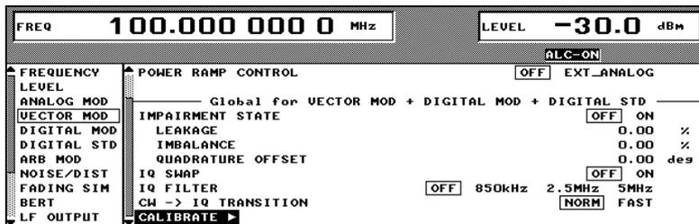
In the *VECTOR MOD* menu, scroll to *CALIBRATE* and execute the calibration.
