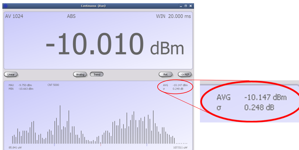
Fig. 32: Measurement of the average RF level of a faded test signal using the Power Viewer Plus software.
