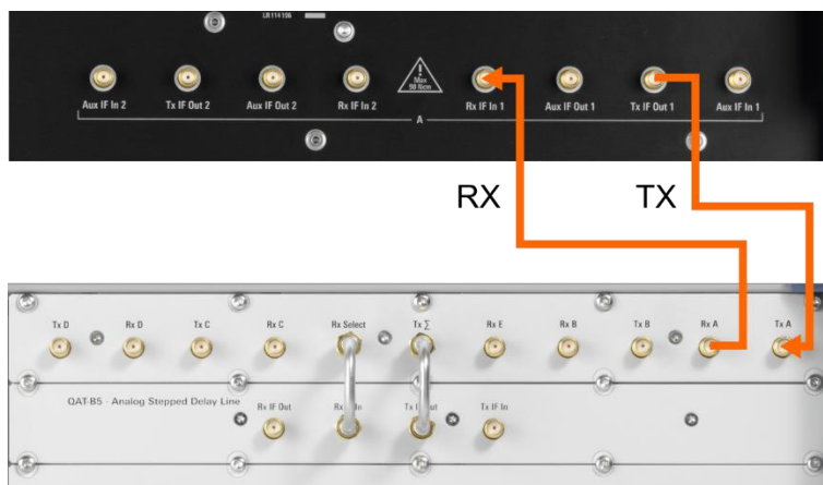
Figure 12: AREG IF channel A1 connected to QAT segment A in segment mode.
