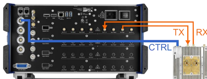
Figure 4: Diagram showing IF signal and control connections for a mmWave frontend connected to the AREG A1 IF channel.
