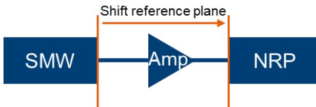
Figure 4: Setup to shift the reference plane
