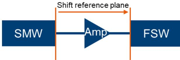
Figure 12: Setup for shifting the power reference plane
