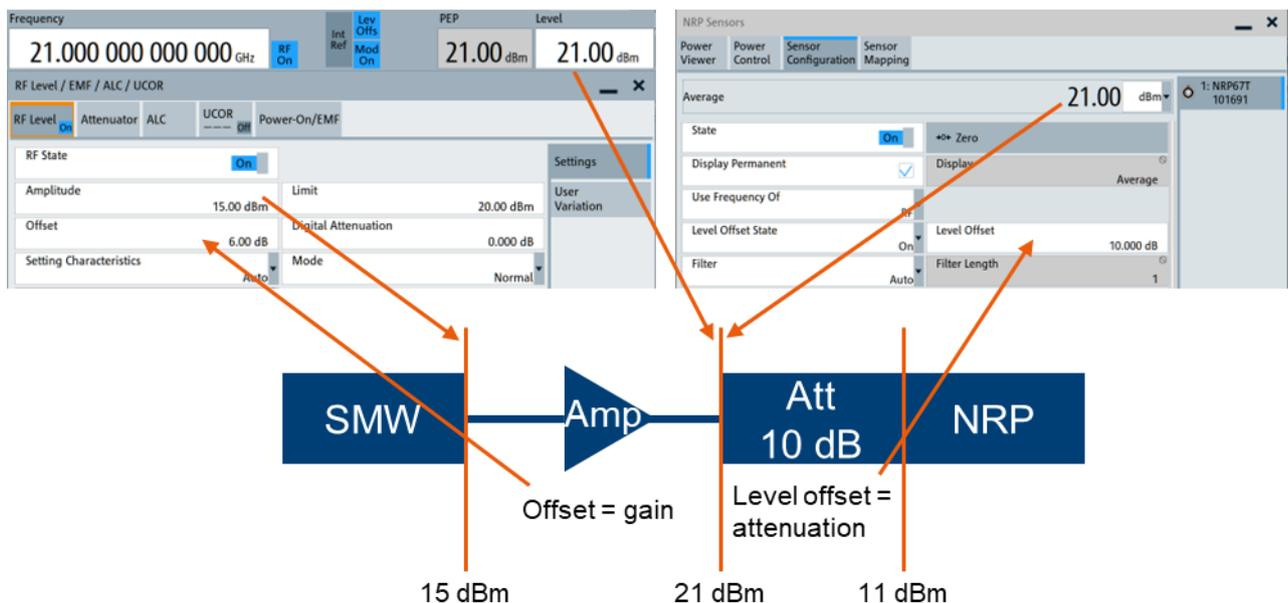
Figure 5: Relation between parameters in the SMW's GUI and levels along the signal path as well as properties of the components. For signals with crest factors higher than 0 dB, the "PEP" is higher than the "Level" by the value of the crest factor. As an example, a crest factor of 8 dB and a "Level" of 21 dBm would result in a "PEP" of 29 dBm.
