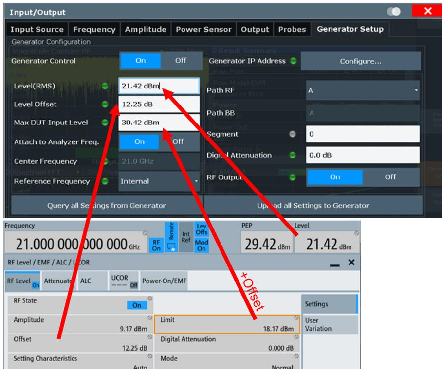
Figure 10: Relation between parameters of the SMW and parameters of the FSW
