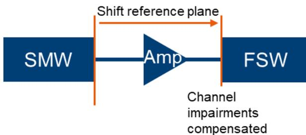
Figure 7: Setup for running Direct DPD and generating a Hammerstein model
