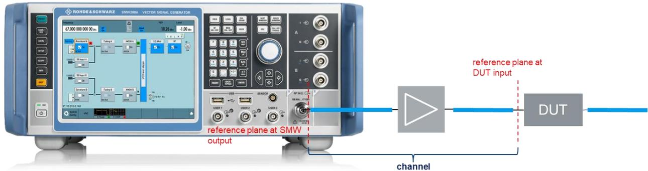
Figure 1: Block diagram showing R&S®SMW200A, external amplifier, cables and DUT
