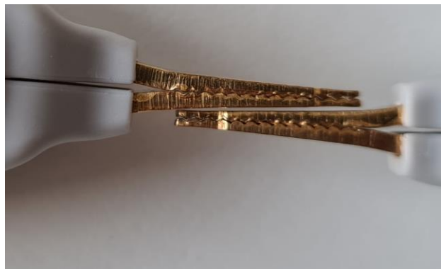
During test measurement: The tips are close but do not touch each other
